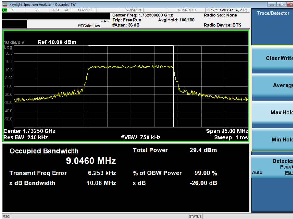
Plot 7-18. Occupied Bandwidth Plot (LTE Band 4 - 10MHz 16-QAM - Full RB)
