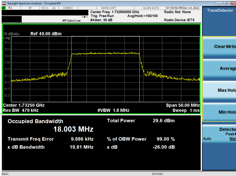
Plot 7-14. Occupied Bandwidth Plot (LTE Band 4 - 20MHz 16-QAM - Full RB)
