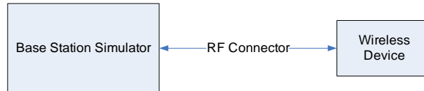
Figure 9-3 Power Measurement Setup – NR FDD
