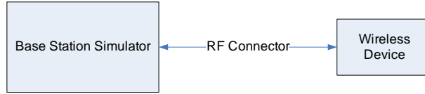
Figure 9-1 Power Measurement Setup
