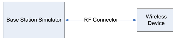
Figure 9-2 Power Measurement Setup
