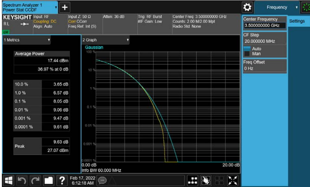
Plot 7-183. PAR Plot (NR Band n77 - 60MHz CP-OFDM 256-QAM - Full RB- DoD-Band - Ant G - SRS 1)
