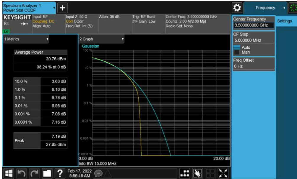
Plot 7-197. PAR Plot (NR Band n77 - 15MHz CP-OFDM QPSK - Full RB- DoD-Band - Ant G - SRS 1)
