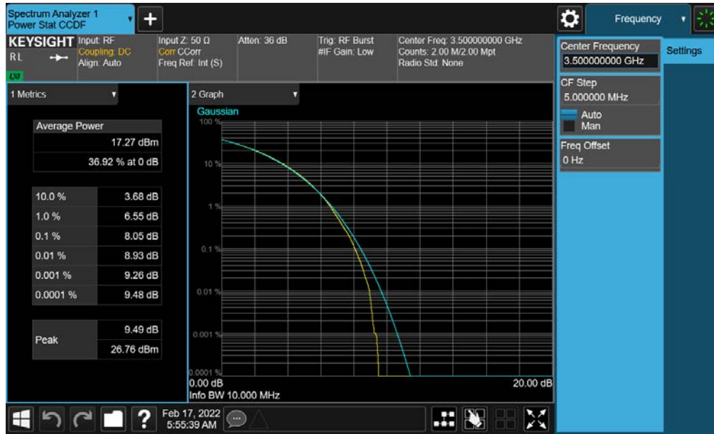
Plot 7-201. PAR Plot (NR Band n77 - 10MHz CP-OFDM 256-QAM - Full RB- DoD-Band - Ant G - SRS 1)
