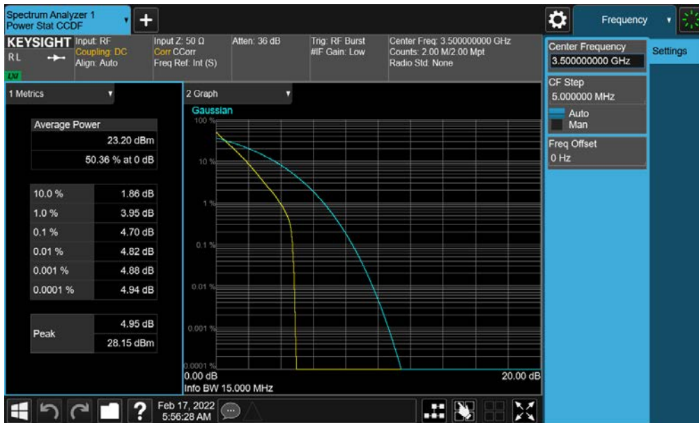
Plot 7-196. PAR Plot (NR Band n77 - 15MHz DFT-s-OFDM BPSK - Full RB- DoD-Band - Ant G - SRS 1)
