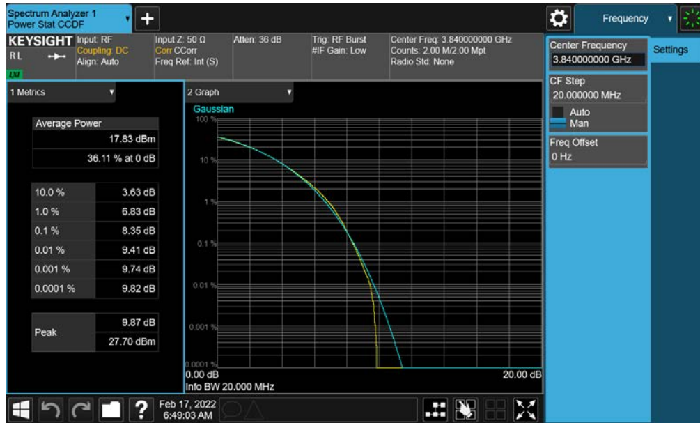
Plot 7-162. PAR Plot (NR Band n77 - 20MHz CP-OFDM 256-QAM - Full RB- C-Band - Ant G - SRS 1)
