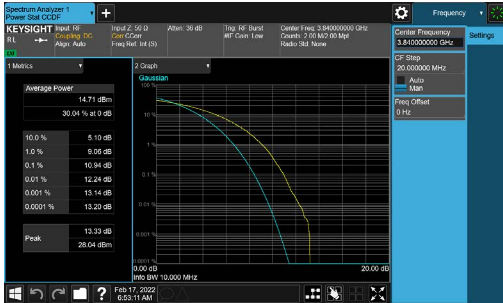
Plot 7-168. PAR Plot (NR Band n77 - 10MHz CP-OFDM 256-QAM - Full RB- C-Band - Ant G - SRS 1)
