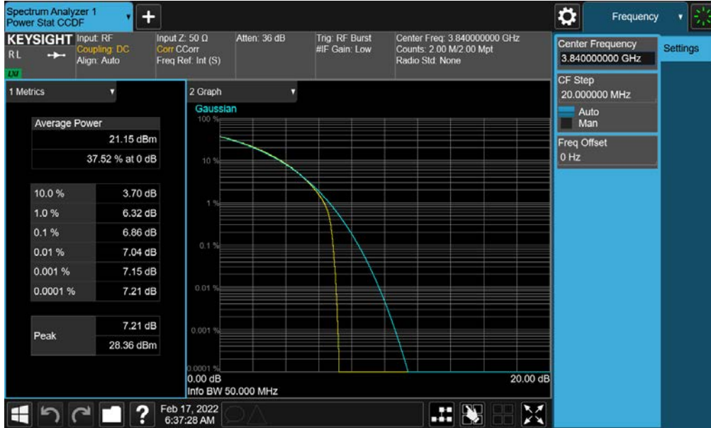
Plot 7-152. PAR Plot (NR Band n77 - 50MHz CP-OFDM QPSK - Full RB- C-Band - Ant G - SRS 1)
