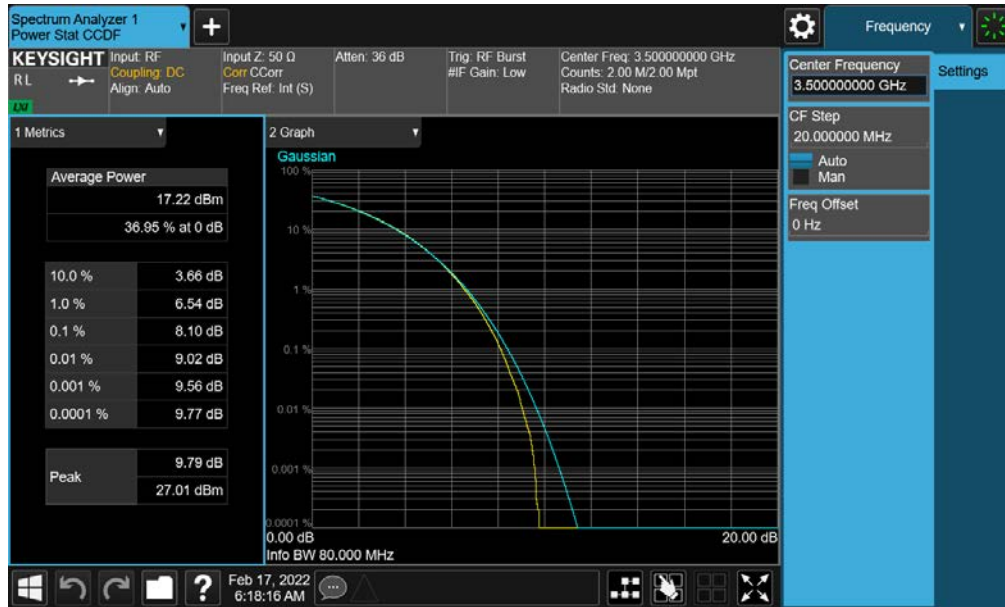
Plot 7-177. PAR Plot (NR Band n77 - 80MHz CP-OFDM 256-QAM - Full RB- DoD-Band - Ant G - SRS 1)
