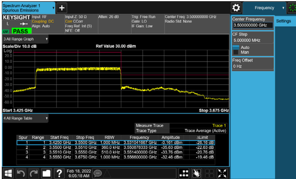
Plot 7-131. Upper ACP Plot (NR Band n77 - 100MHz CP-OFDM-QPSK – Full RB – DoD-Band - Ant C - SRS 2)
