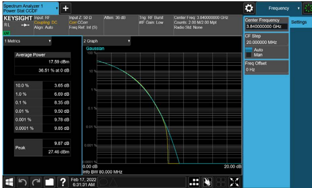
Plot 7-144. PAR Plot (NR Band n77 - 80MHz CP-OFDM 256-QAM - Full RB- C-Band - Ant G - SRS 1)
