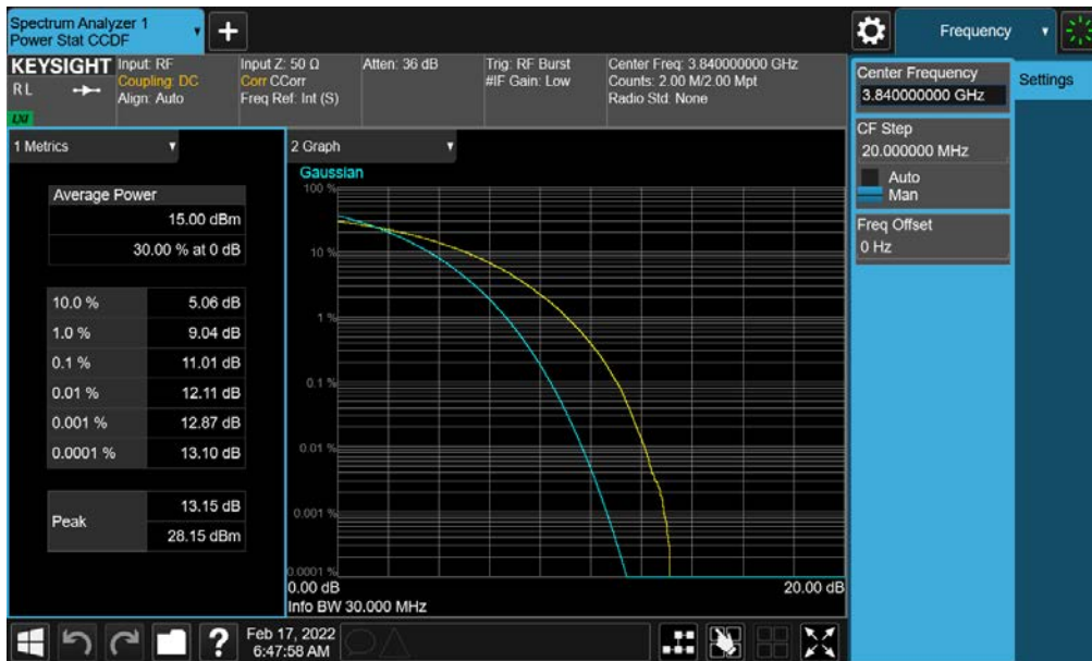
Plot 7-159. PAR Plot (NR Band n77 - 30MHz CP-OFDM 256-QAM - Full RB- C-Band - Ant G - SRS 1)
