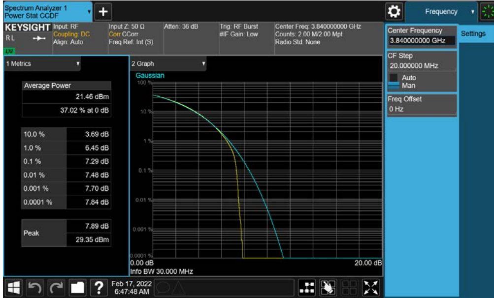
Plot 7-158. PAR Plot (NR Band n77 - 30MHz CP-OFDM QPSK - Full RB- C-Band - Ant G - SRS 1)
