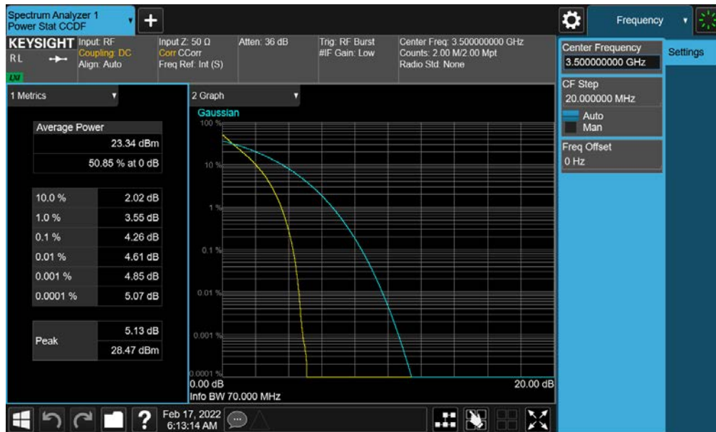
Plot 7-178. PAR Plot (NR Band n77 - 70MHz DFT-s-OFDM BPSK - Full RB- DoD-Band - Ant G - SRS 1)
