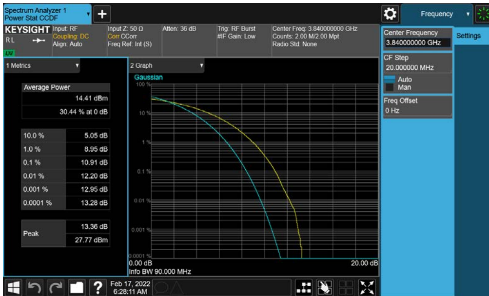
Plot 7-141. PAR Plot (NR Band n77 - 90MHz CP-OFDM 256-QAM - Full RB- C-Band - Ant G - SRS 1)
