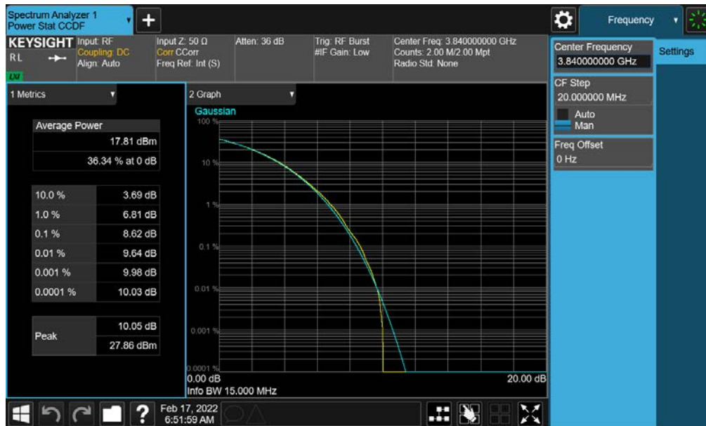
Plot 7-165. PAR Plot (NR Band n77 - 15MHz CP-OFDM 256-QAM - Full RB- C-Band - Ant G - SRS 1)
