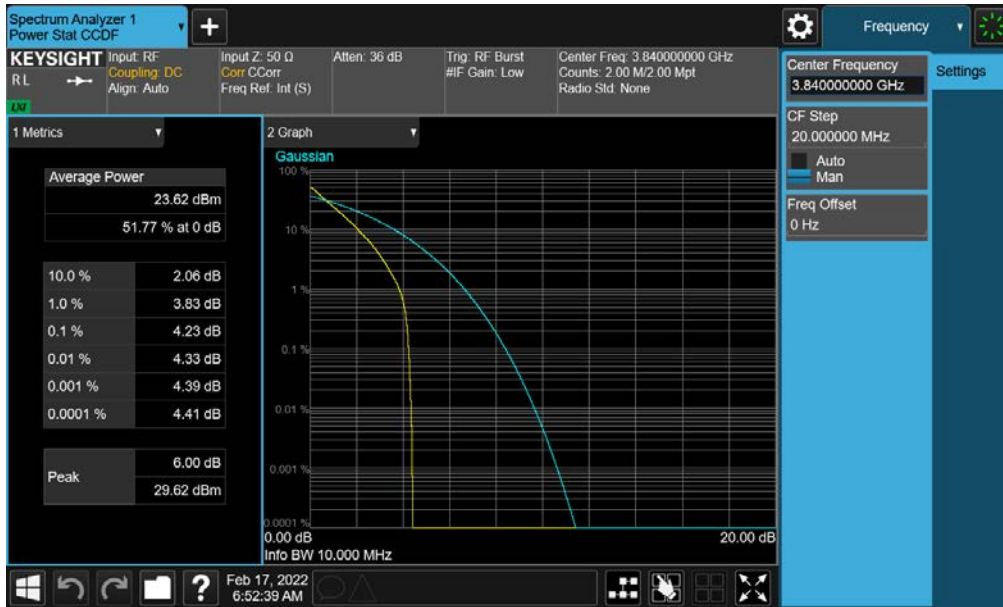
Plot 7-166. PAR Plot (NR Band n77 - 10MHz DFT-s-OFDM BPSK - Full RB- C-Band - Ant G - SRS 1)
