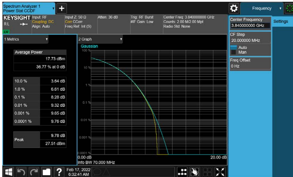
Plot 7-147. PAR Plot (NR Band n77 - 70MHz CP-OFDM 256-QAM - Full RB- C-Band - Ant G - SRS 1)
