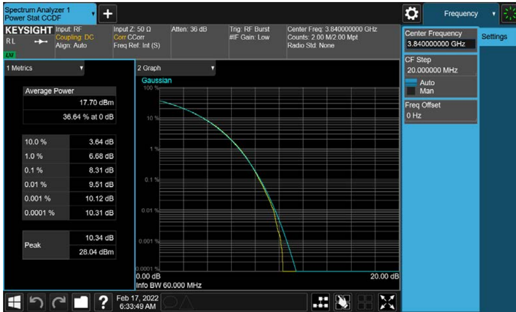
Plot 7-150. PAR Plot (NR Band n77 - 60MHz CP-OFDM 256-QAM - Full RB- C-Band - Ant G - SRS 1)
