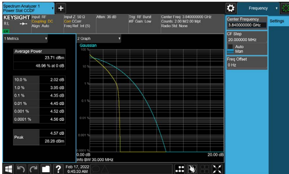
Plot 7-157. PAR Plot (NR Band n77 - 30MHz DFT-s-OFDM BPSK - Full RB- C-Band - Ant G - SRS 1)
