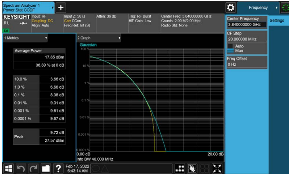
Plot 7-156. PAR Plot (NR Band n77 - 40MHz CP-OFDM 256-QAM - Full RB- C-Band - Ant G - SRS 1)
