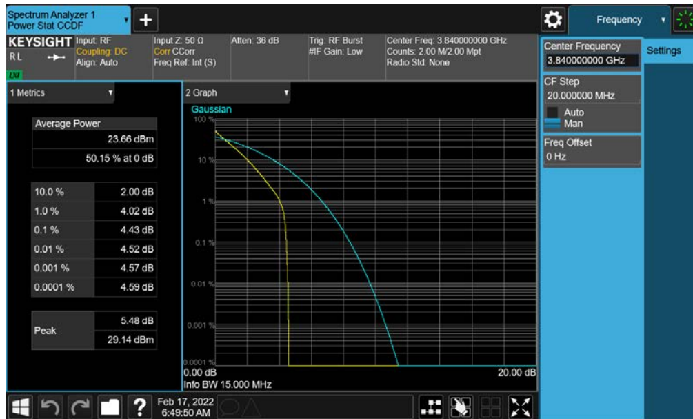
Plot 7-163. PAR Plot (NR Band n77 - 15MHz DFT-s-OFDM BPSK - Full RB- C-Band - Ant G - SRS 1)
