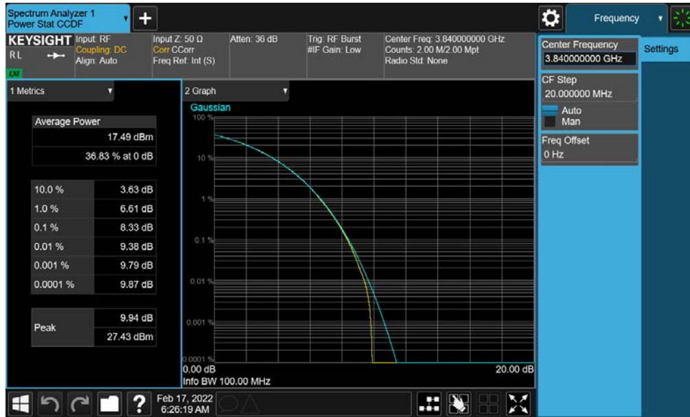
Plot 7-138. PAR Plot (NR Band n77 - 100MHz CP-OFDM 256-QAM - Full RB- C-Band - Ant G - SRS 1)
