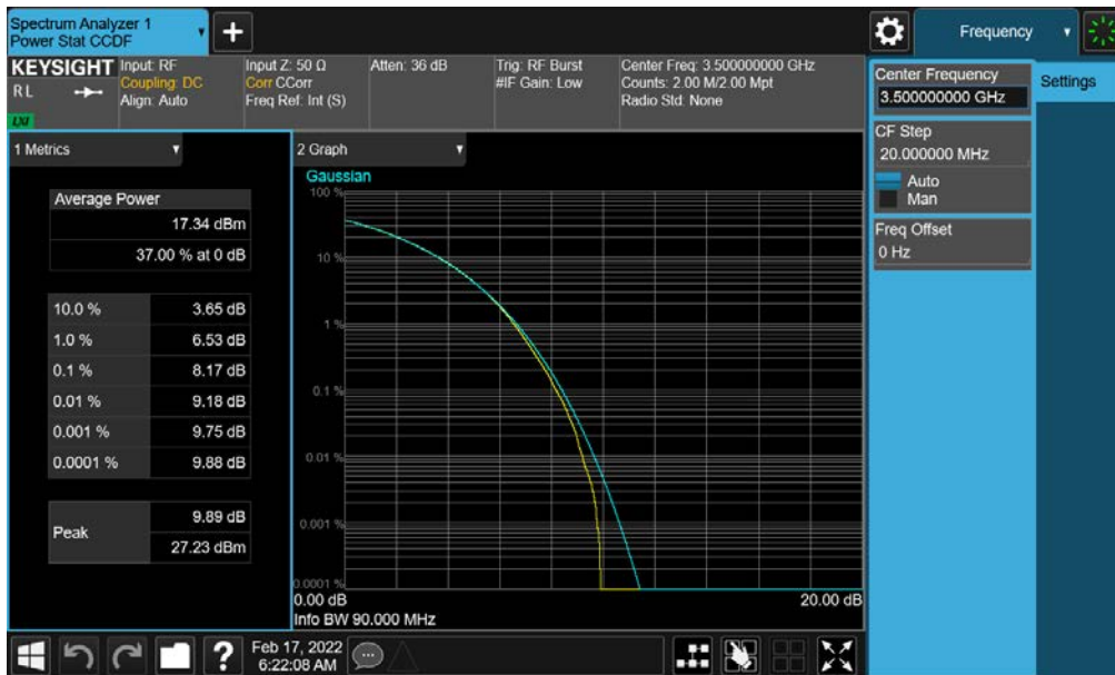
Plot 7-174. PAR Plot (NR Band n77 - 90MHz CP-OFDM 256-QAM - Full RB- DoD-Band - Ant G - SRS 1)
