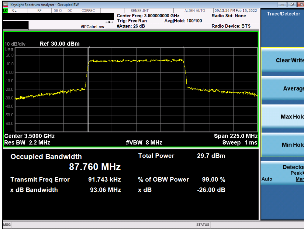
Plot 7-46. Occupied Bandwidth Plot (NR Band n77 - 90MHz QPSK - Full RB - Ant G - SRS1)
