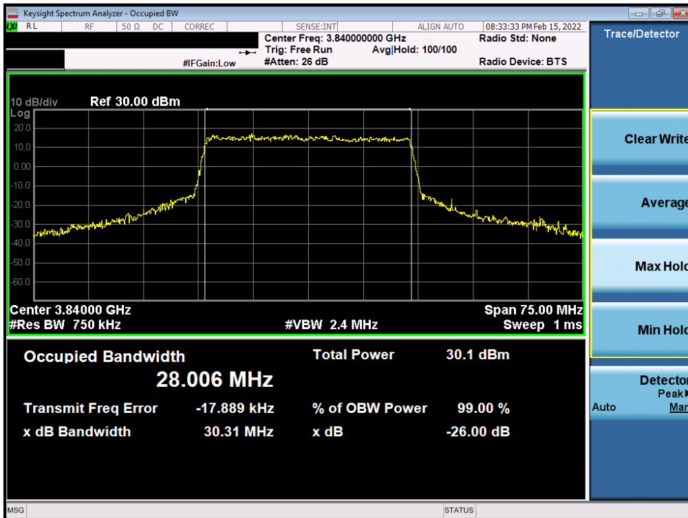
Plot 7-32. Occupied Bandwidth Plot (NR Band n77 - 30MHz 16-QAM - Full RB - Ant G - SRS1)
