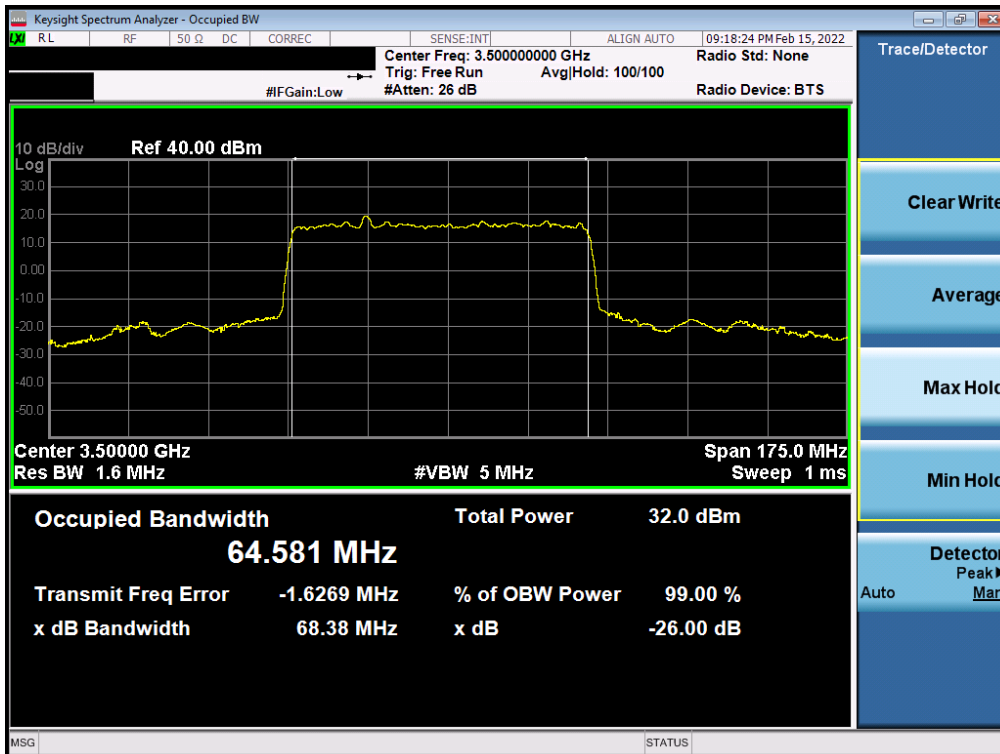
Plot 7-51. Occupied Bandwidth Plot (NR Band n77 - 70MHz \pi/2 BPSK - Full RB - Ant G - SRS1)
