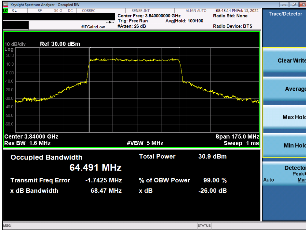
Plot 7-19. Occupied Bandwidth Plot (NR Band n77 - 70MHz QPSK - Full RB - Ant G - SRS1)
