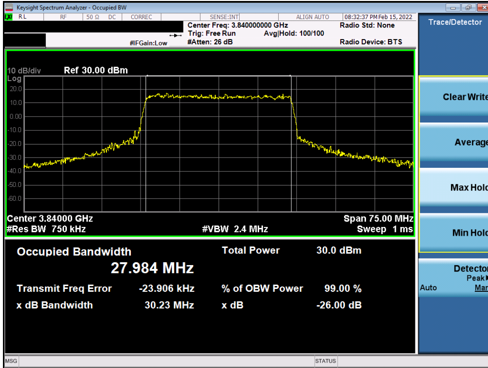
Plot 7-31. Occupied Bandwidth Plot (NR Band n77 - 30MHz QPSK - Full RB - Ant G - SRS1)
