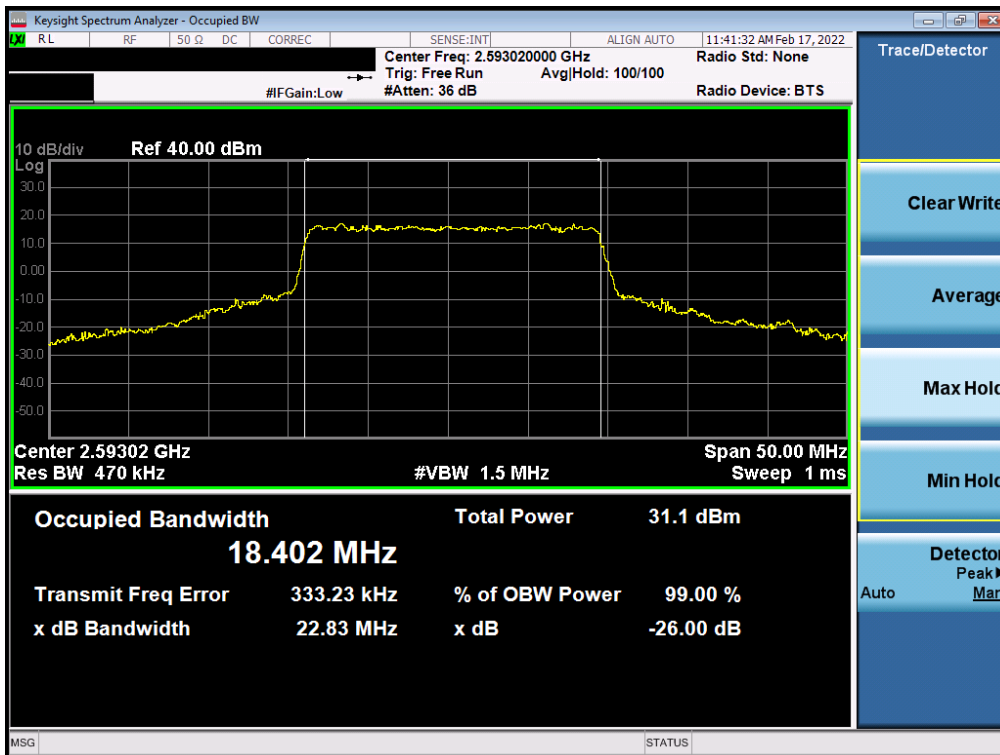
Plot 7-28. Occupied Bandwidth Plot (NR Band n41 - 20MHz 16-QAM - Full RB – Ant F)
