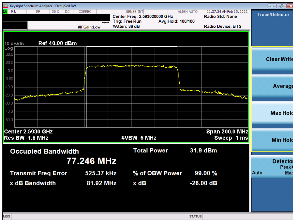
Plot 7-12. Occupied Bandwidth Plot (NR Band n41 - 80MHz QPSK - Full RB - Ant F)
