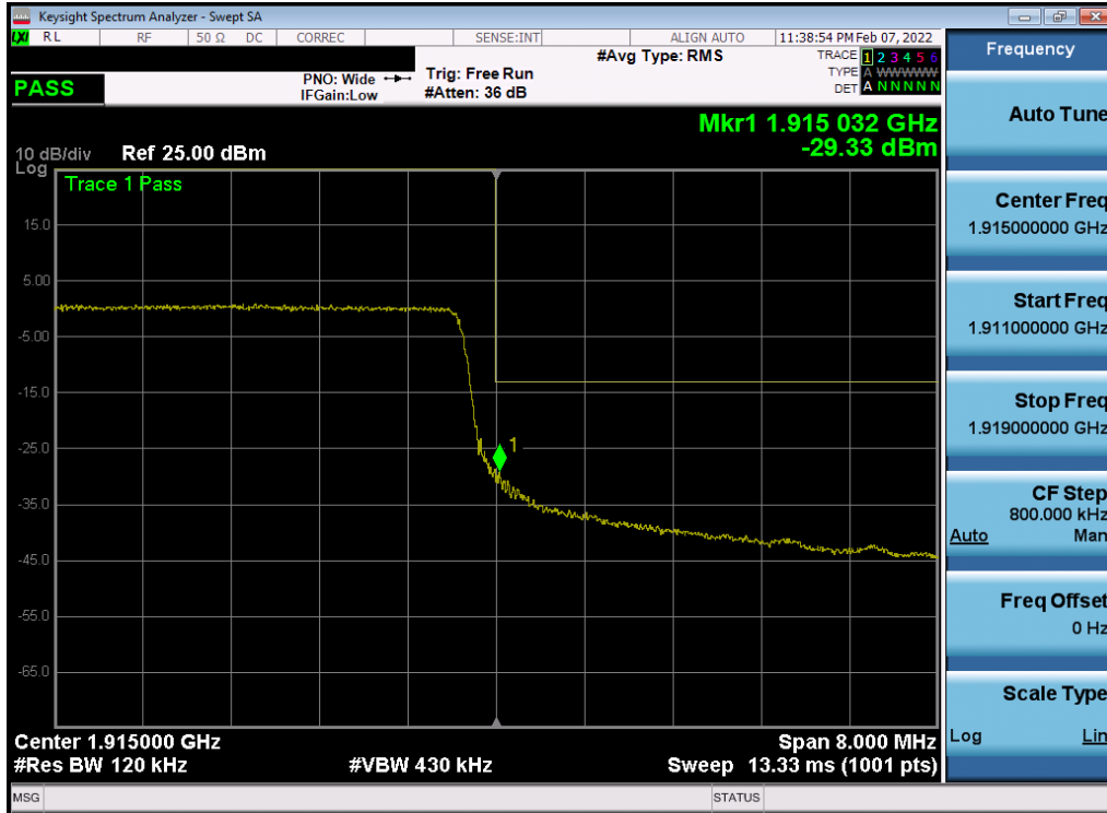
Plot 7-38. Upper Band Edge Plot (NR Band n25 - 10MHz QPSK – Full RB)
