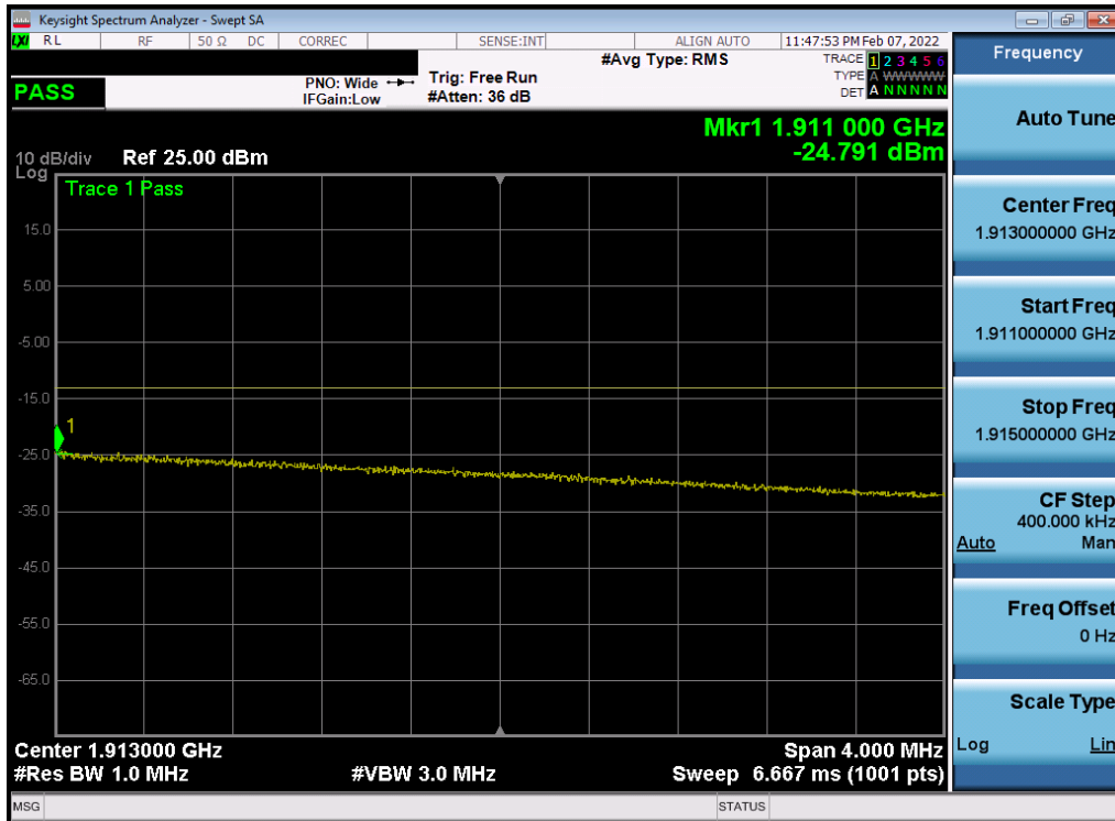
Plot 7-25. Extended Upper Band Edge Plot (NR Band n2 - 20MHz QPSK – Full RB)
