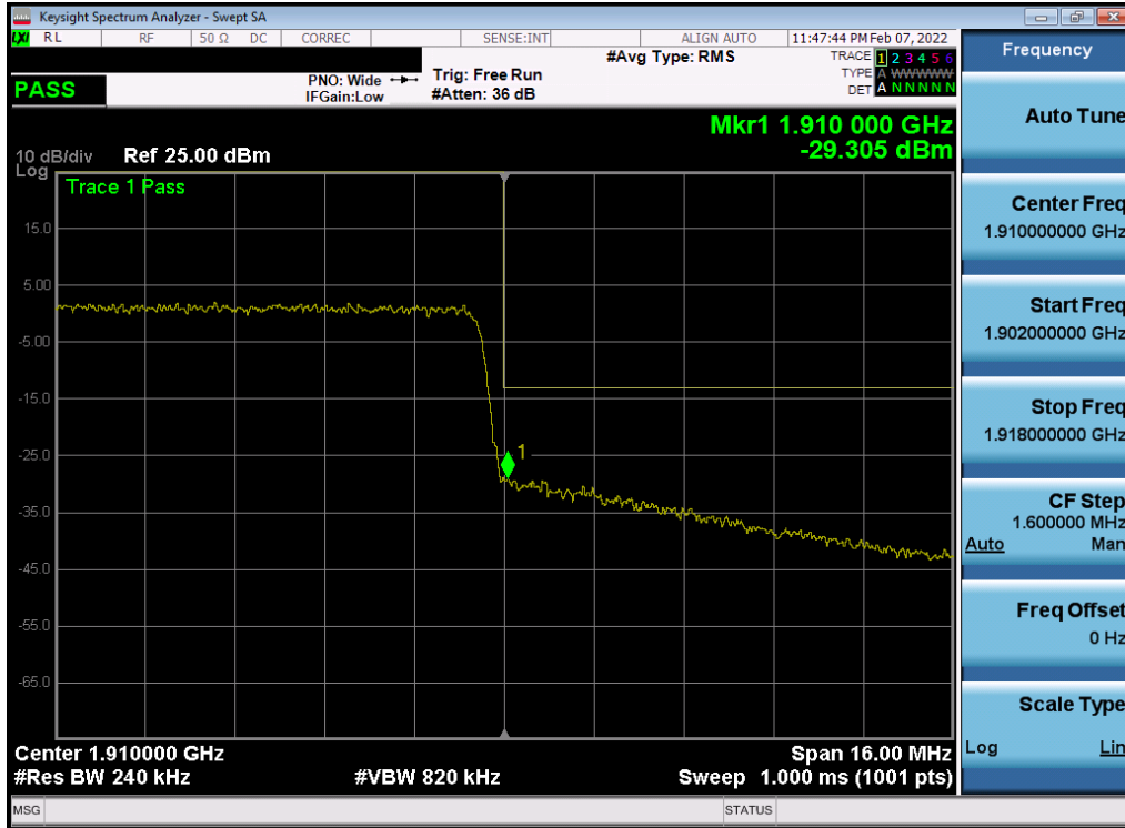
Plot 7-24. Upper Band Edge Plot (NR Band n2 - 20MHz QPSK – Full RB)
