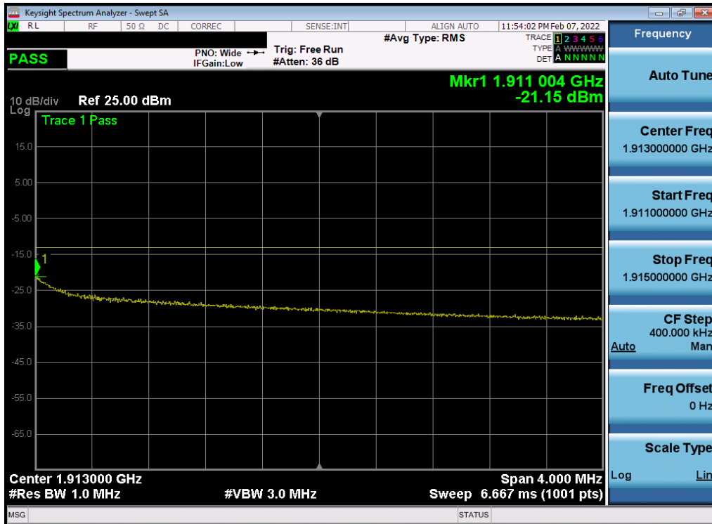
Plot 7-37. Extended Upper Band Edge Plot (NR Band n2 - 10MHz QPSK – Full RB)
