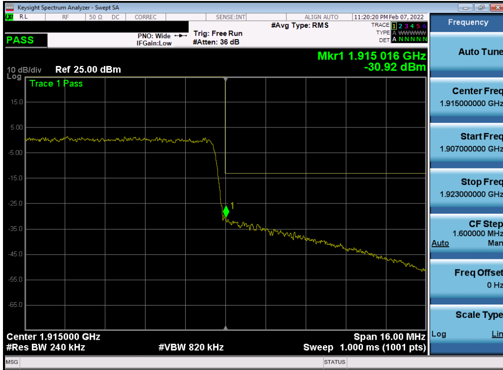
Plot 7-26. Upper Band Edge Plot (NR Band n25 - 20MHz QPSK – Full RB)
