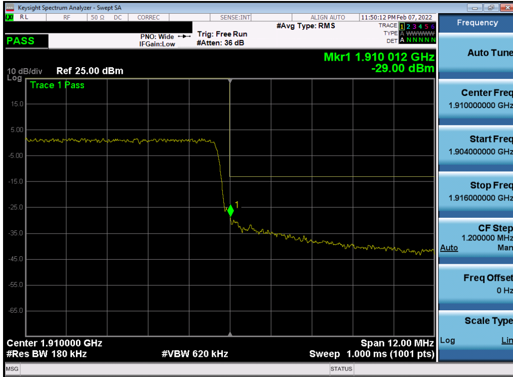
Plot 7-30. Upper Band Edge Plot (NR Band n2 - 15MHz QPSK – Full RB)
