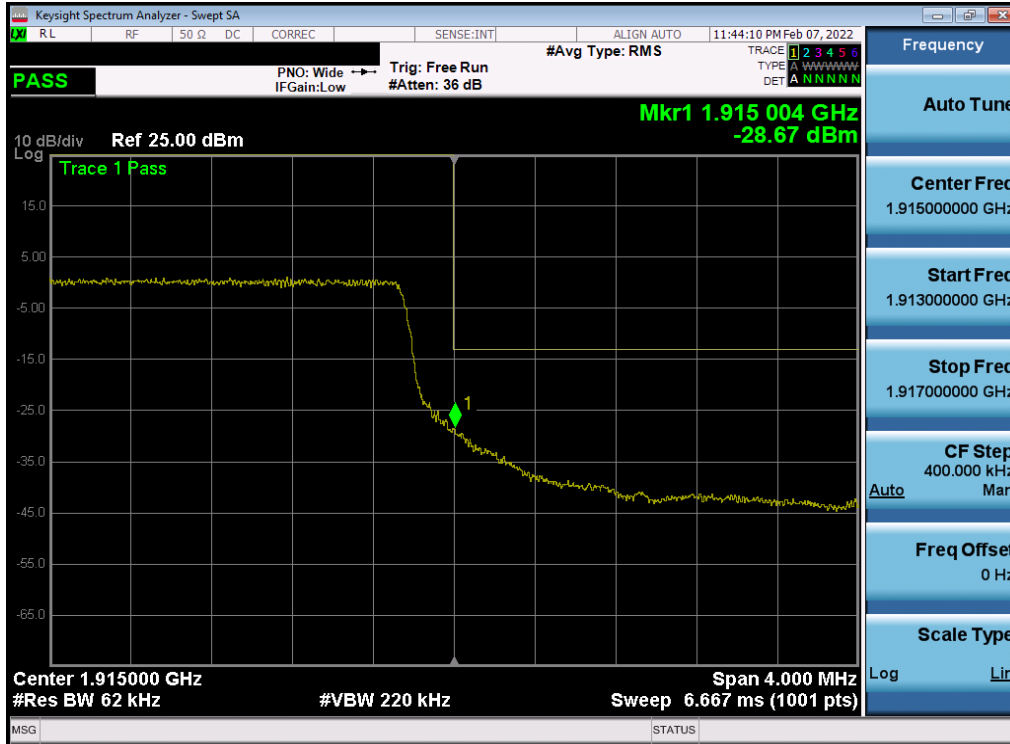
Plot 7-44. Upper Band Edge Plot (NR Band n25 – 5MHz QPSK – Full RB)
