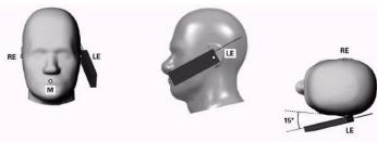
Figure 6-2 Front, Side and Top View of Ear/15° Tilt
