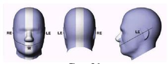
Figure 5-2 Front, back and side view of SAM Twin Phantom
