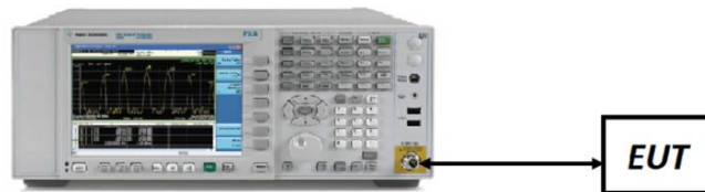
Figure 7-4. Test Instrument & Measurement Setup
