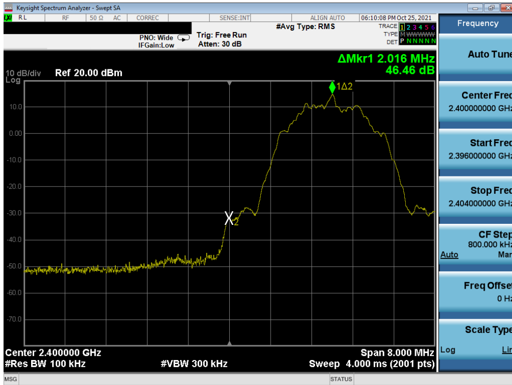
Plot 7-37. Band Edge Plot (Bluetooth (LE), 2Mbps – Ch. 0)
