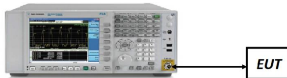
Figure 7-1. Test Instrument & Measurement Setup
