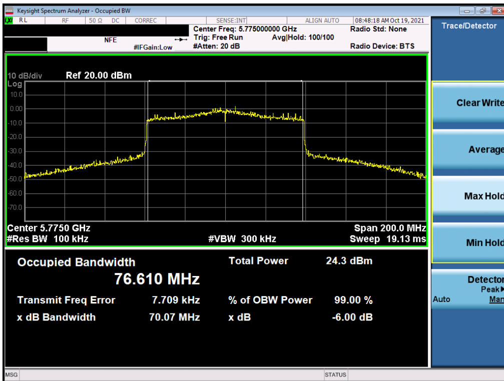
Plot 7-146. 6dB Bandwidth Plot SISO ANT2 (80MHz BW 802.11ax (UNII Band 3) – Ch. 155)
