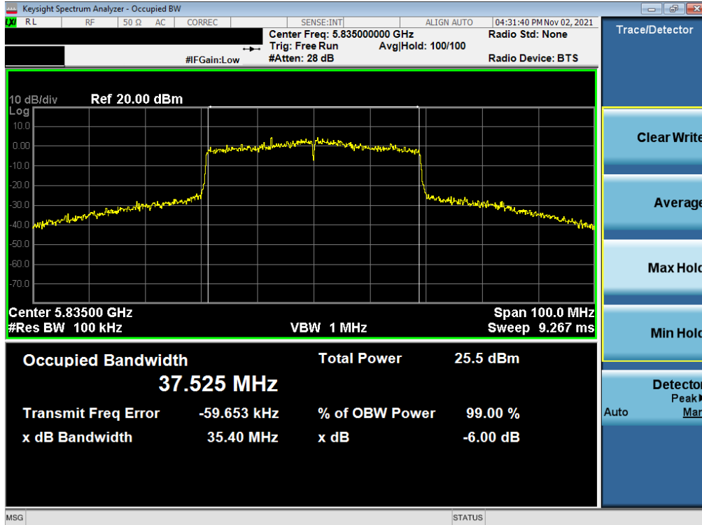
Plot 7-156. 6dB Bandwidth Plot SISO ANT2 (40MHz BW 802.11n (UNII Band 3/4) – Ch. 167)
