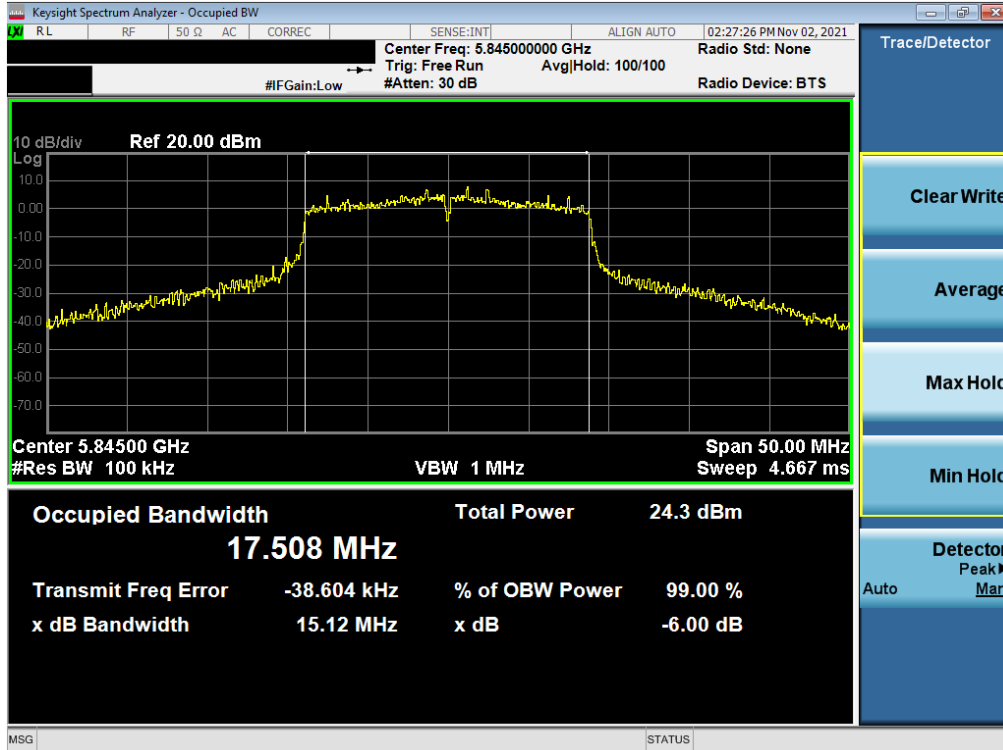
Plot 7-150. 6dB Bandwidth Plot SISO ANT2 (20MHz BW 802.11n (UNII Band 3/4) – Ch. 169)
