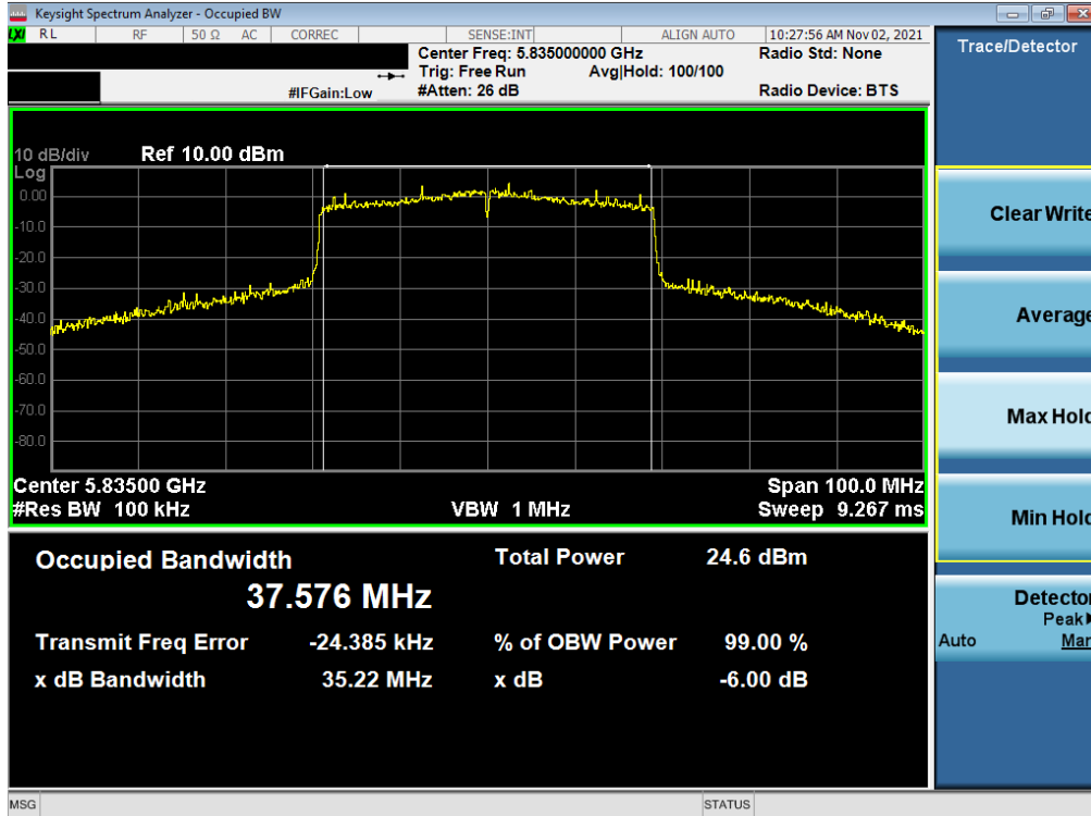
Plot 7-129. 6dB Bandwidth Plot SISO ANT1 (40MHz BW 802.11ax (UNII Band 3/4) – Ch. 167)
