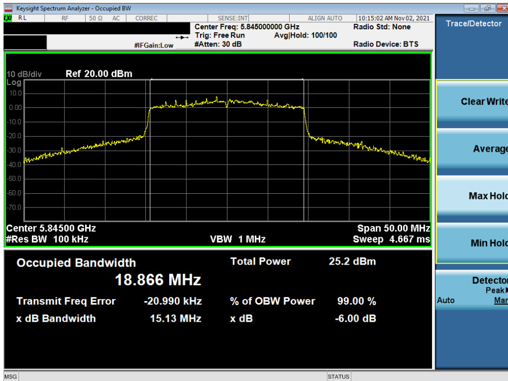
Plot 7-124. 6dB Bandwidth Plot SISO ANT1 (20MHz BW 802.11ax (UNII Band 3/4) – Ch. 169)
