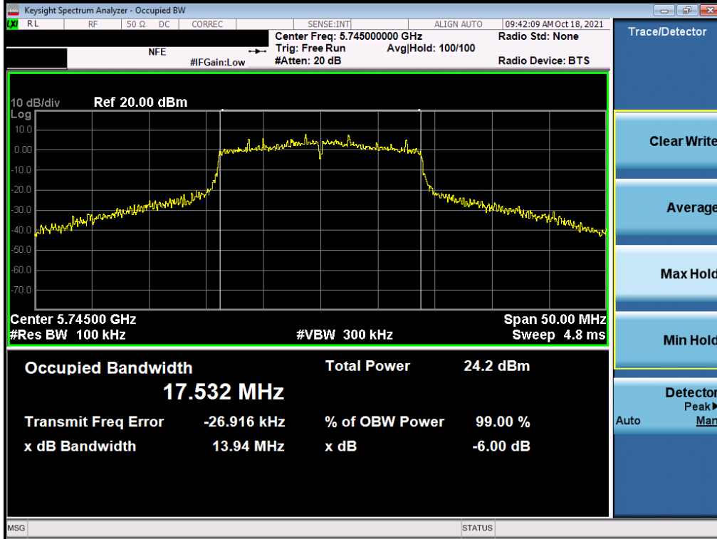
Plot 7-135. 6dB Bandwidth Plot SISO ANT2 (20MHz BW 802.11n (UNII Band 3) – Ch. 149)
