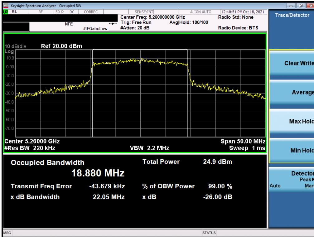
Plot 7-73. 26dB Bandwidth Plot SISO ANT2 (20MHz BW 802.11ax (UNII Band 2A) – Ch. 52)
