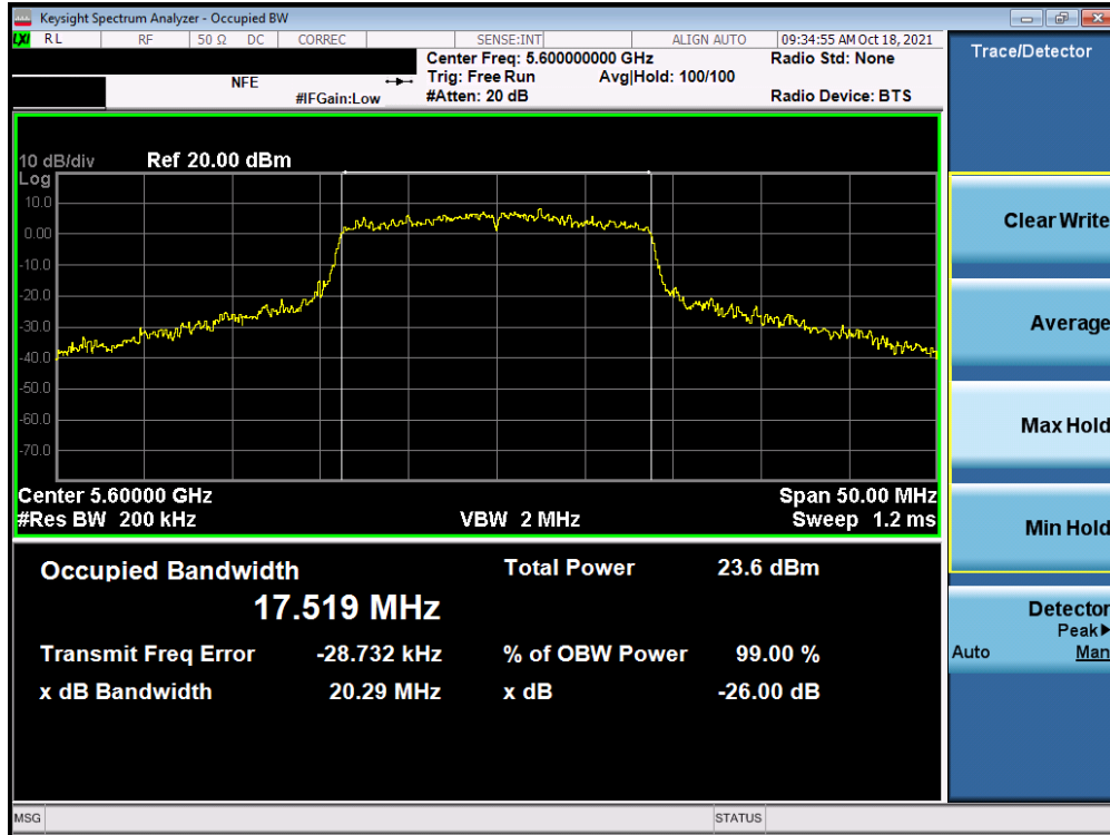
Plot 7-35. 26dB Bandwidth Plot SISO ANT1 (20MHz BW 802.11n (UNII Band 2C) – Ch. 120)
