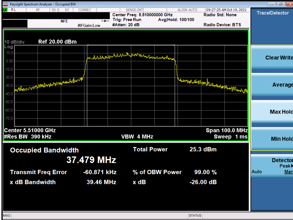
Plot 7-43. 26dB Bandwidth Plot SISO ANT1 (40MHz BW 802.11ax (UNII Band 2C) – Ch. 102)
