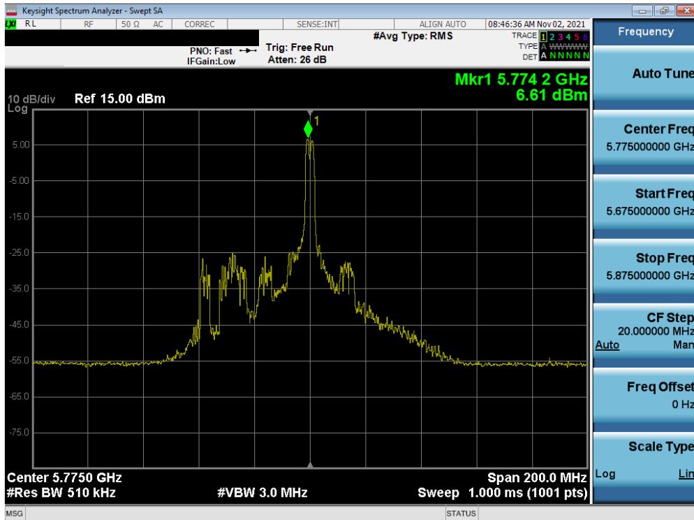
Plot 7-159. Power Spectral Density Plot SISO ANT1 (80MHz BW 802.11ax – 26 Tones (UNII Band 3) – Ch. 155)
