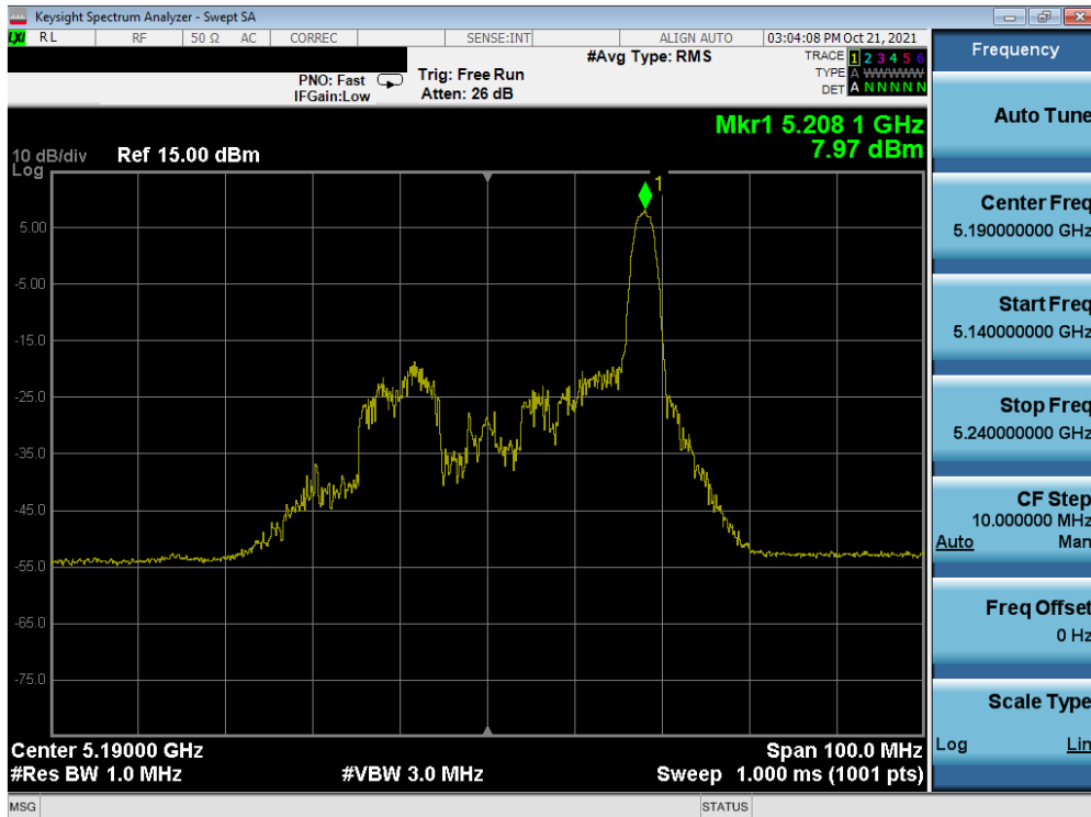
Plot 7-136. Power Spectral Density Plot SISO ANT1 (40MHz BW 802.11ax – 26 Tones (UNII Band 1) – Ch. 38)
