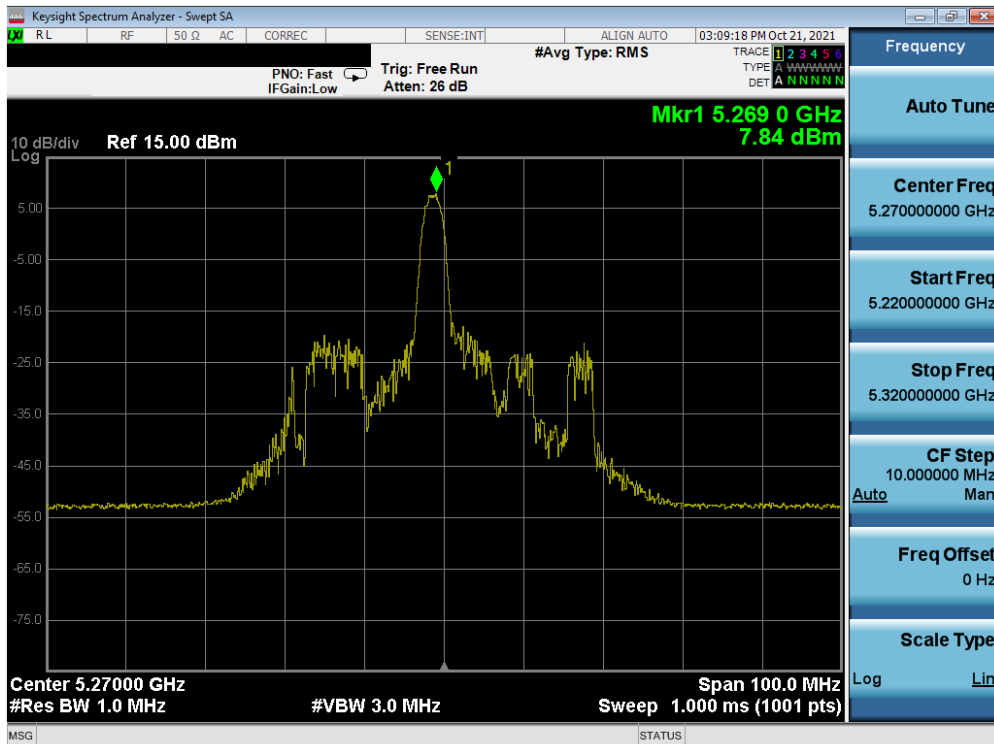
Plot 7-142. Power Spectral Density Plot SISO ANT1 (40MHz BW 802.11ax – 26 Tones (UNII Band 2A) – Ch. 54)
