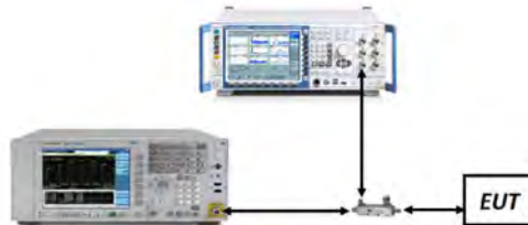
Figure 7-4. Test Instrument & Measurement Setup
