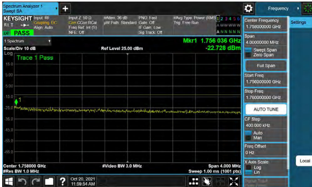
Plot 7-93. Upper Extended Band Edge Plot (LTE Band 4 - 10MHz QPSK – Full RB)
