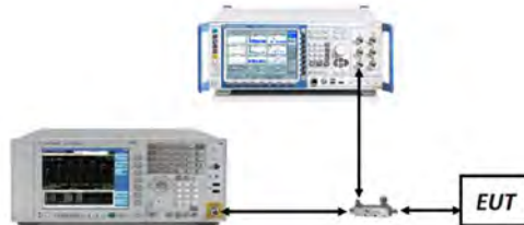
Figure 7-2. Test Instrument & Measurement Setup
