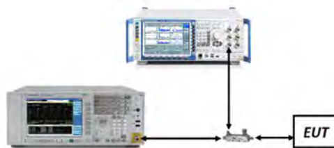
Figure 7-1. Test Instrument & Measurement Setup
