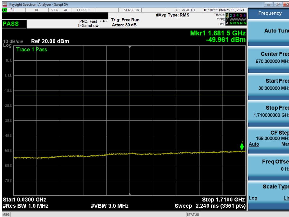
Plot 7-37. Conducted Spurious Plot (NR Band n66 - 20MHz - 1 RB - Mid Channel – ANT F)
