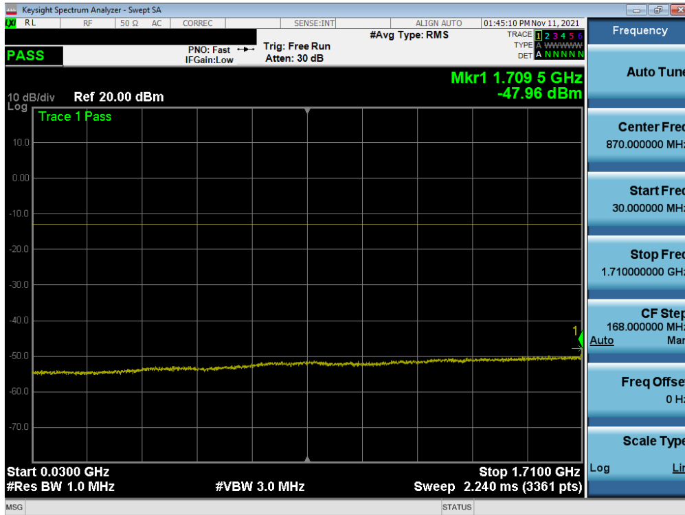
Plot 7-34. Conducted Spurious Plot (NR Band n66 -20MHz - 1 RB - Low Channel – ANT F)
