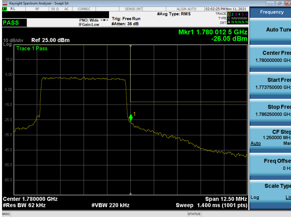
Plot 7-76. Upper Band Edge Plot (NR Band n66 – 5.0MHz - Full RB – ANT F)
