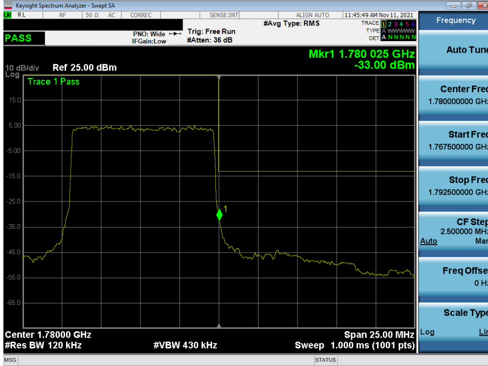
Plot 7-56. Upper Band Edge Plot (NR Band n66 – 10.0MHz - Full RB – ANT A)
