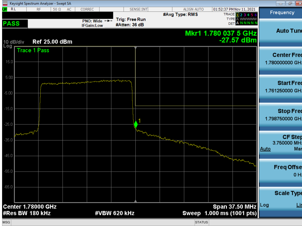
Plot 7-68. Upper Band Edge Plot (NR Band n66 – 15.0MHz - Full RB – ANT F)
