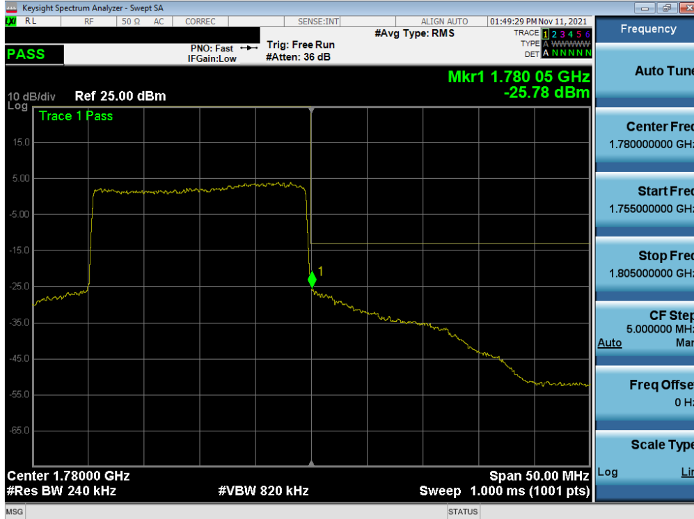
Plot 7-64. Upper Band Edge Plot (NR Band n66 – 20.0MHz - Full RB – ANT F)
