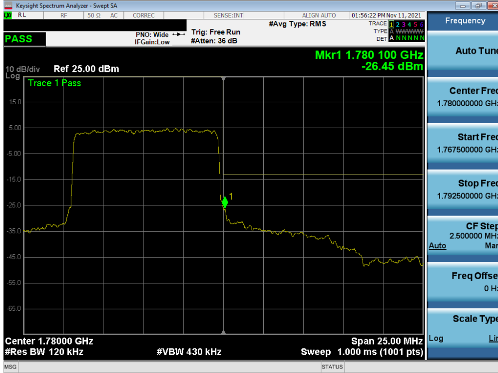
Plot 7-72. Upper Band Edge Plot (NR Band n66 – 10.0MHz - Full RB – ANT F)
