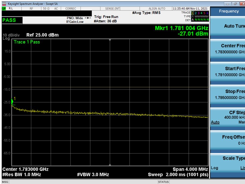
Plot 7-49. Upper Extended Band Edge Plot (NR Band n66 – 20.0MHz - Full RB – ANT A)
