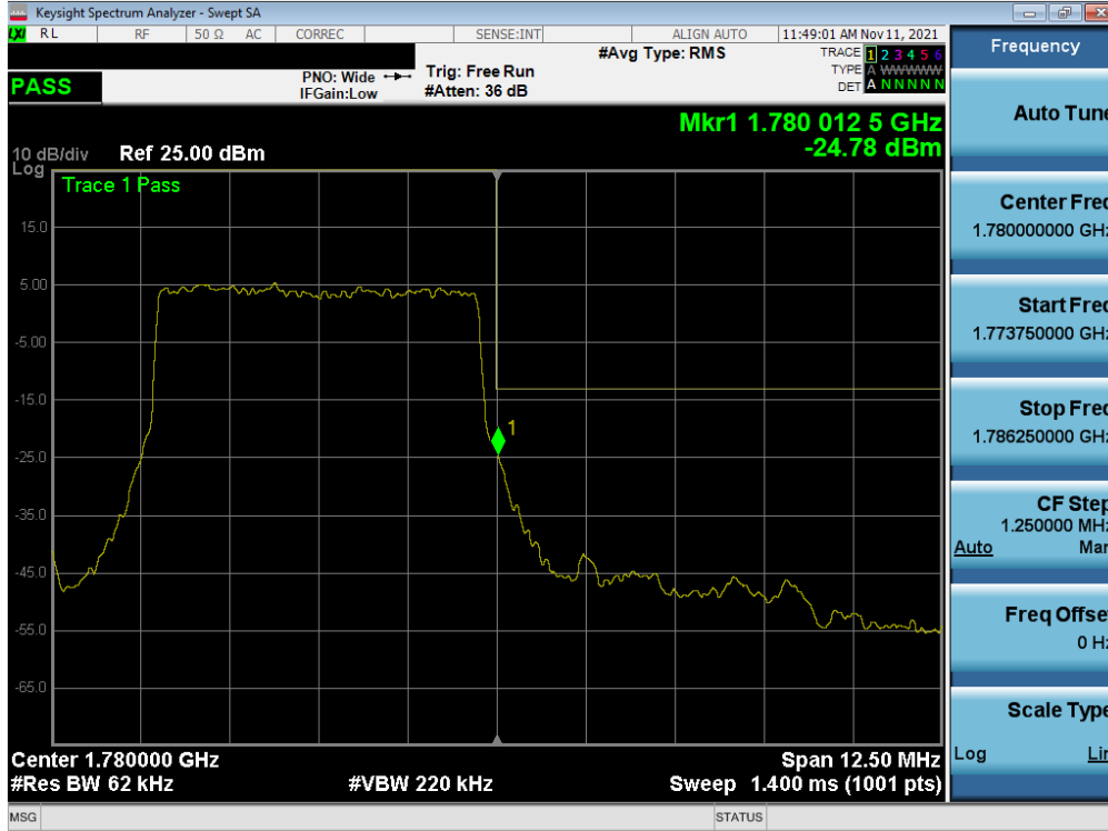
Plot 7-60. Upper Band Edge Plot (NR Band n66 – 5.0MHz - Full RB – ANT A)
