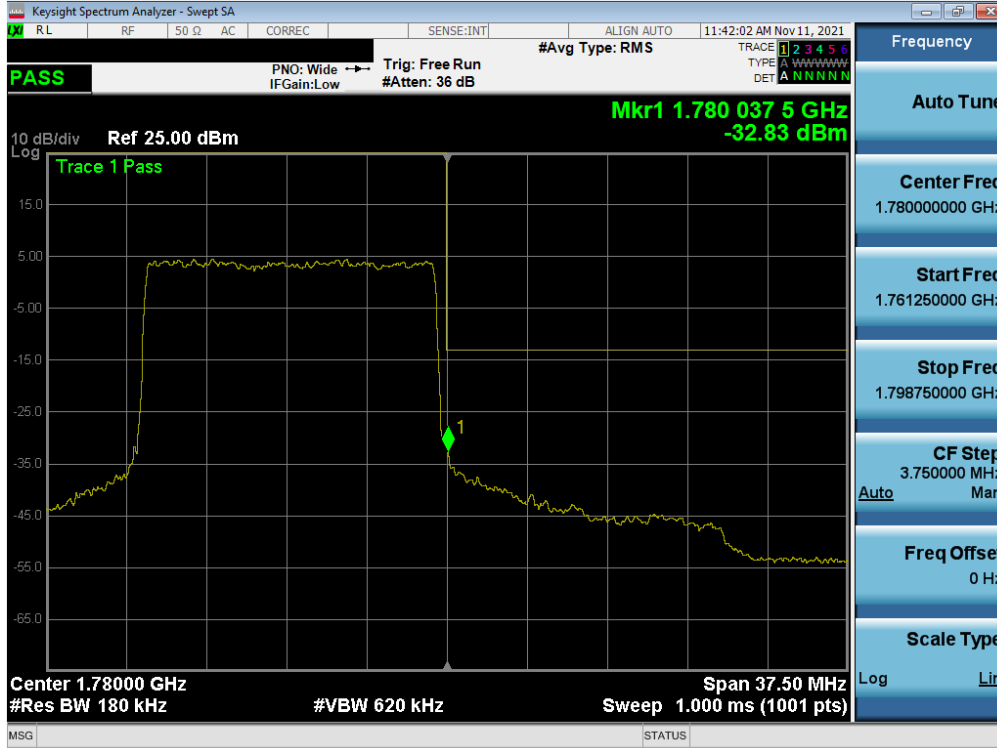
Plot 7-52. Upper Band Edge Plot (NR Band n66 – 15.0MHz - Full RB – ANT A)
