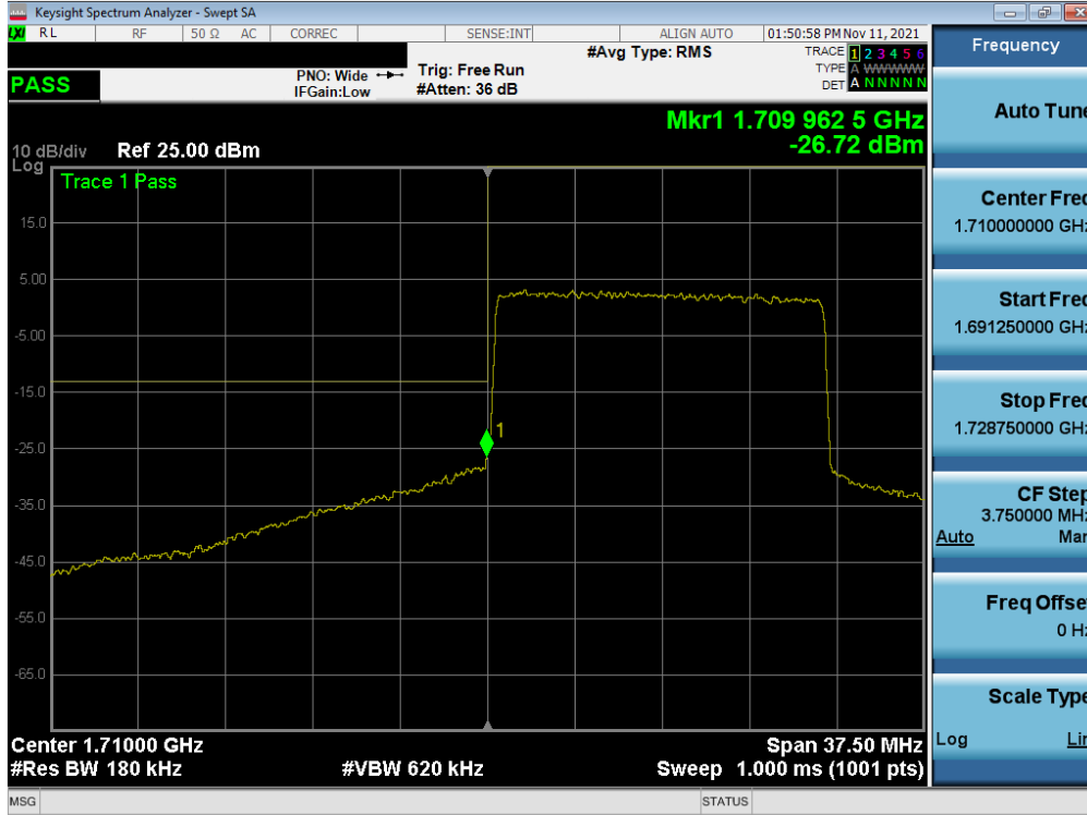
Plot 7-66. Lower Band Edge Plot (NR Band n66 – 15.0MHz - Full RB – ANT F)
