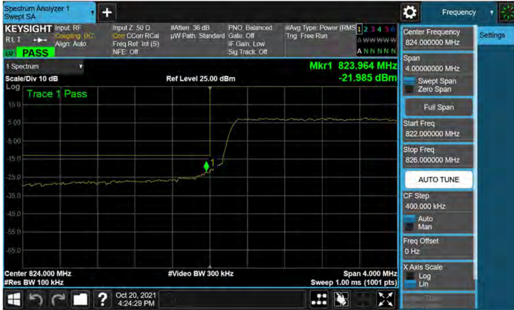
Plot 7-45. Lower Band Edge Plot (LTE Band 26/5 - 5MHz QPSK – Full RB)
