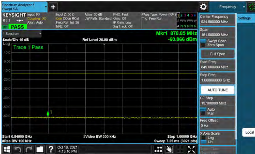
Plot 7-33. Conducted Spurious Plot (WCDMA Ch. 4132)
