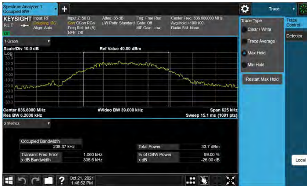
Plot 7-12. Occupied Bandwidth Plot (EDGE, Ch. 190)
