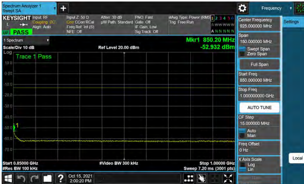
Plot 7-21. Conducted Spurious Plot (LTE Band 26/5 - 10MHz QPSK - 1 RB - High Channe)
