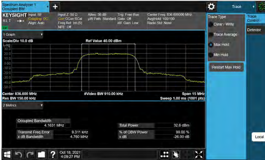
Plot 7-13. Occupied Bandwidth Plot (WCDMA, Ch. 4183)
