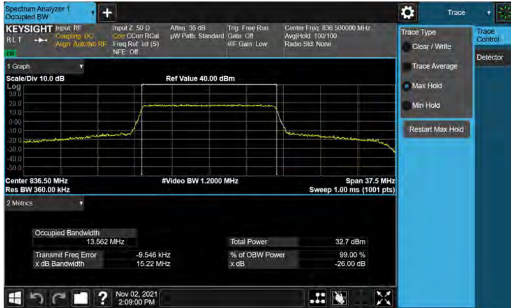
Plot 7-1. Occupied Bandwidth Plot (LTE Band 26 - 15MHz QPSK - Full RB)
