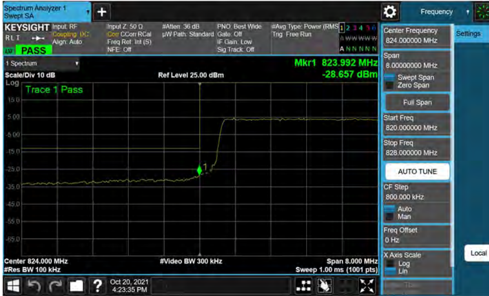
Plot 7-43. Lower Band Edge Plot (LTE Band 26/5 - 10MHz QPSK – Full RB)
