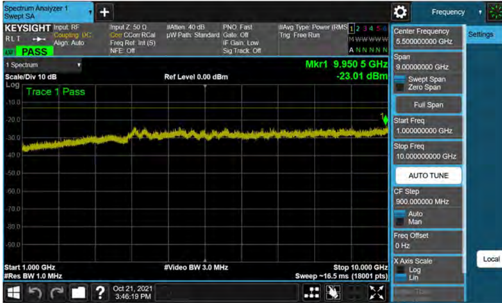
Plot 7-25. Conducted Spurious Plot (GPRS Ch. 128)
