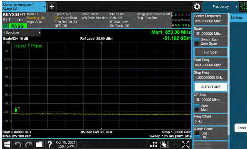
Plot 7-18. Conducted Spurious Plot (LTE Band 26/5 - 10MHz QPSK - 1 RB - Mid Channel)
