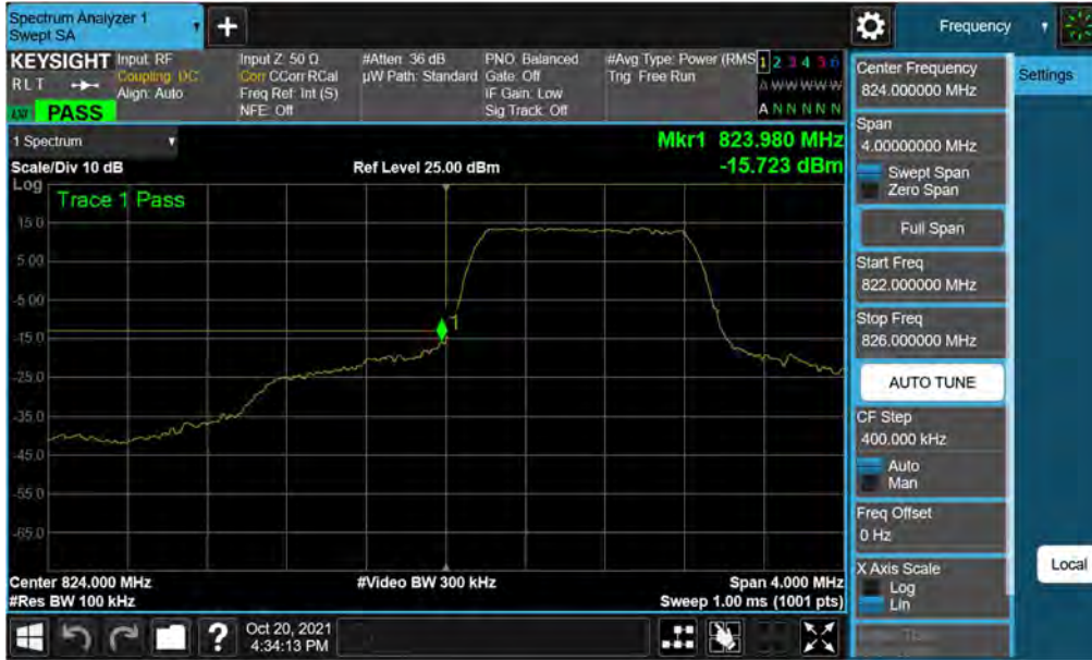
Plot 7-49. Lower Band Edge Plot (LTE Band 26/5 – 1.4MHz QPSK – Full RB)
