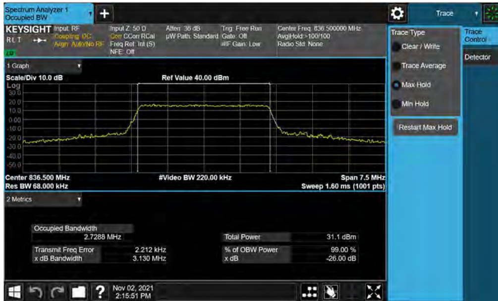
Plot 7-8. Occupied Bandwidth Plot (LTE Band 26/5 - 3MHz 16-QAM - Full RB)
