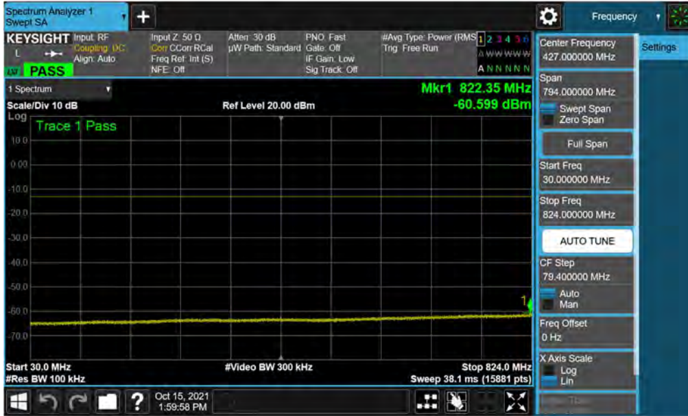
Plot 7-20. Conducted Spurious Plot (LTE Band 26/5 - 10MHz QPSK - 1 RB - High Channe)
