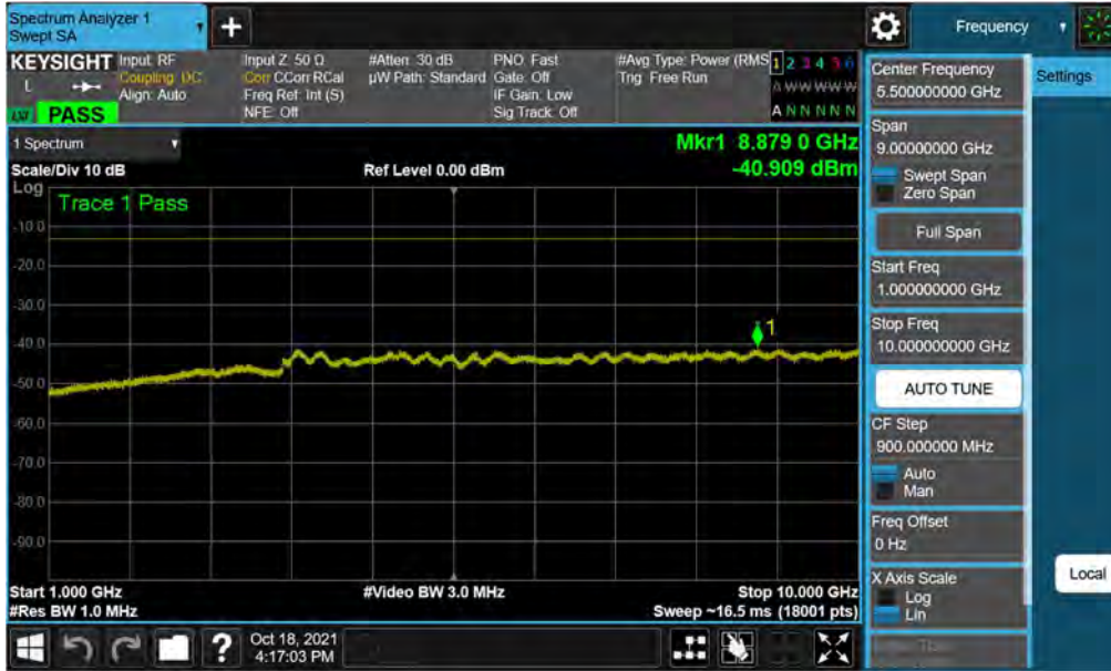
Plot 7-40. Conducted Spurious Plot (WCDMA Ch. 4233)
