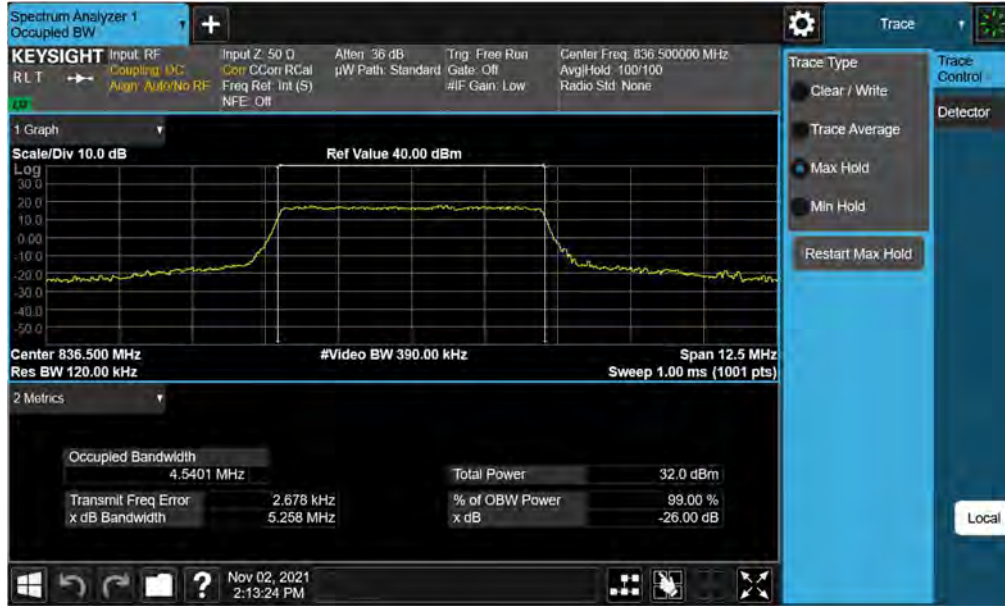
Plot 7-5. Occupied Bandwidth Plot (LTE Band 26/5 - 5MHz QPSK - Full RB)
