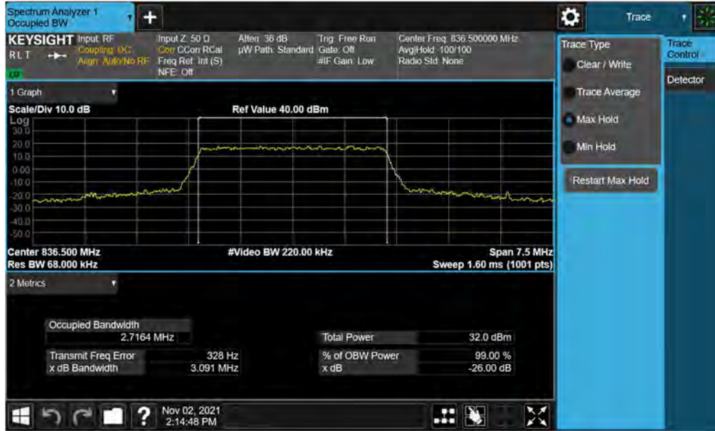
Plot 7-7. Occupied Bandwidth Plot (LTE Band 26/5 - 3MHz QPSK - Full RB)
