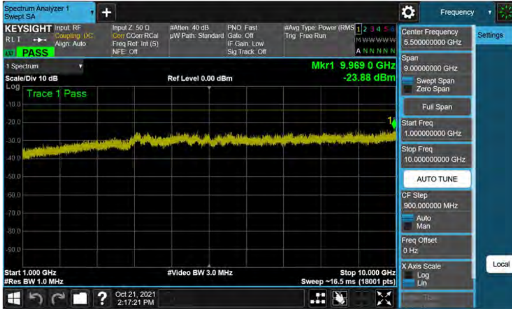
Plot 7-31. Conducted Spurious Plot (GPRS Ch. 251)
