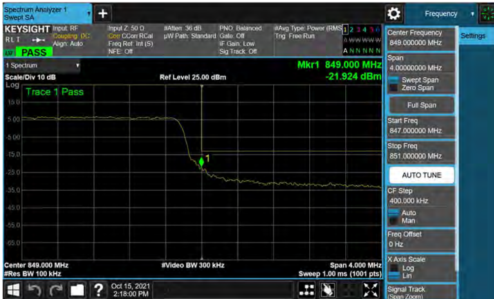
Plot 7-46. Upper Band Edge Plot (LTE Band 26/5 - 5MHz QPSK – Full RB)
