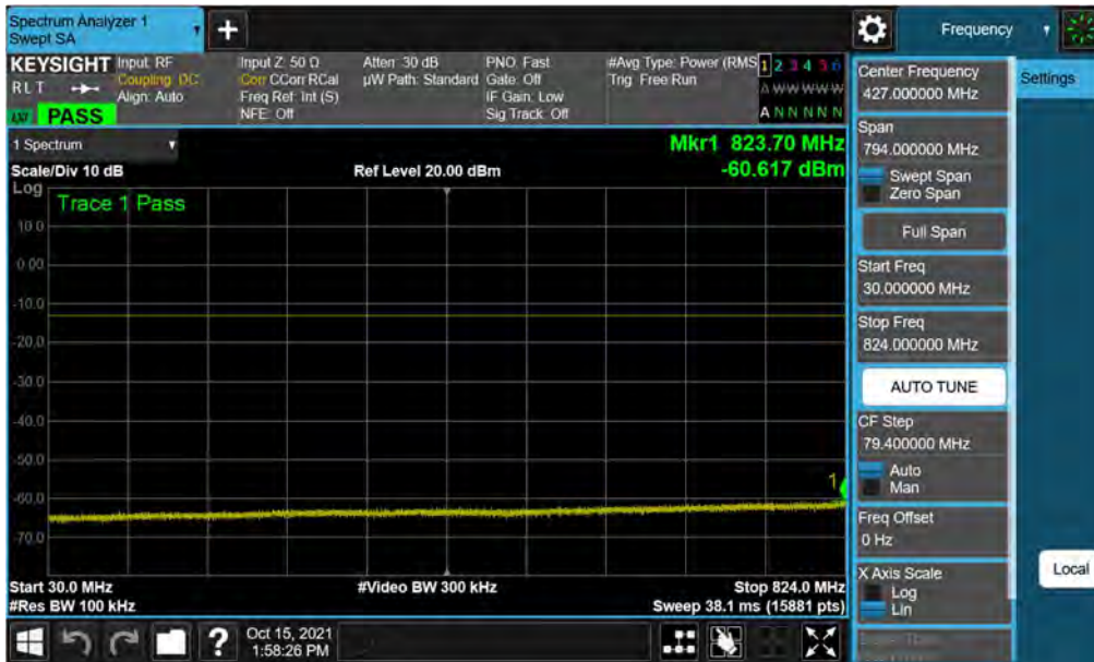
Plot 7-17. Conducted Spurious Plot (LTE Band 26/5 - 10MHz QPSK - 1 RB - Mid Channel)
