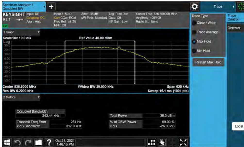
Plot 7-11. Occupied Bandwidth Plot (GPRS, Ch. 190)
