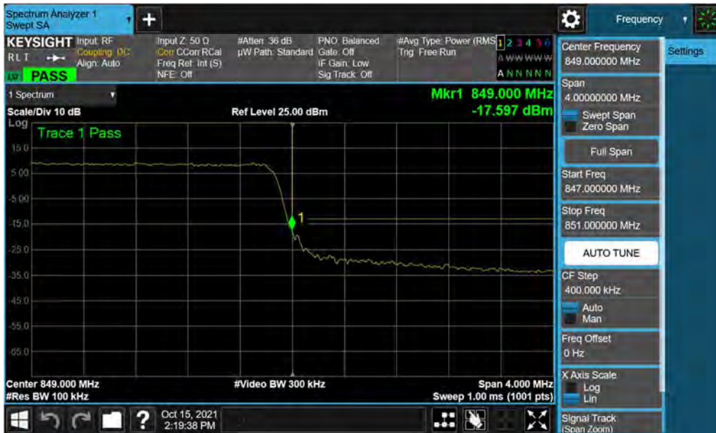
Plot 7-48. Upper Band Edge Plot (LTE Band 26/5 - 3MHz QPSK – Full RB)
