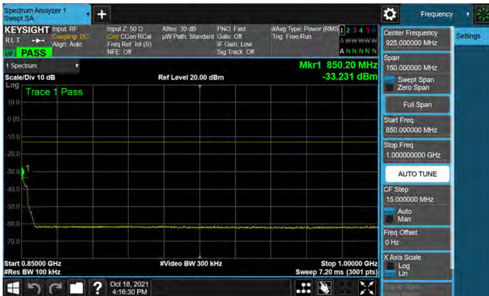
Plot 7-39. Conducted Spurious Plot (WCDMA Ch. 4233)
