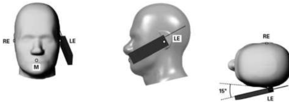
Figure 8.5. Tilt 15° position of the wireless device
