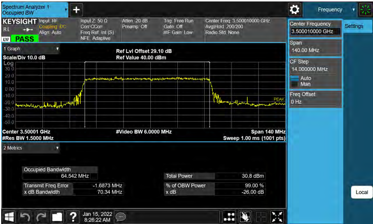
Sub6 n77. Occupied Bandwidth Plot (70 M BW Ch.633334 BPSK )
