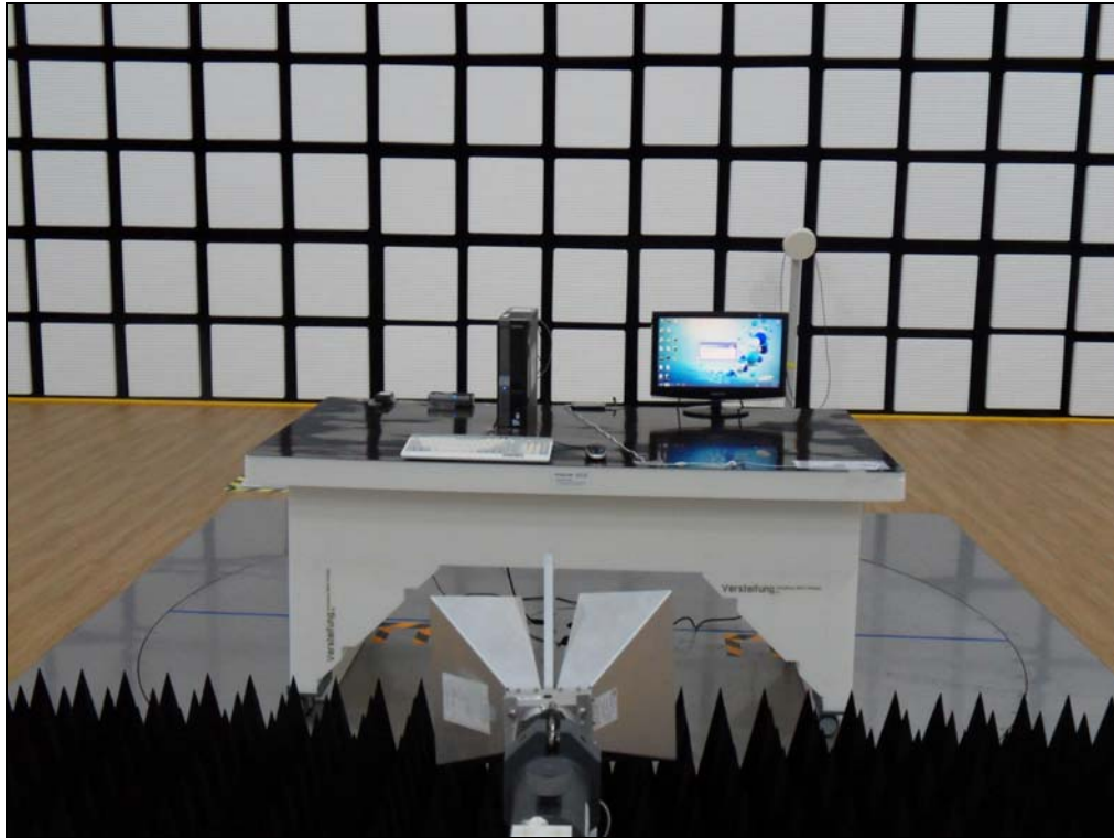
[ Radiated Disturbance for Above 1 GHz – Front ]
