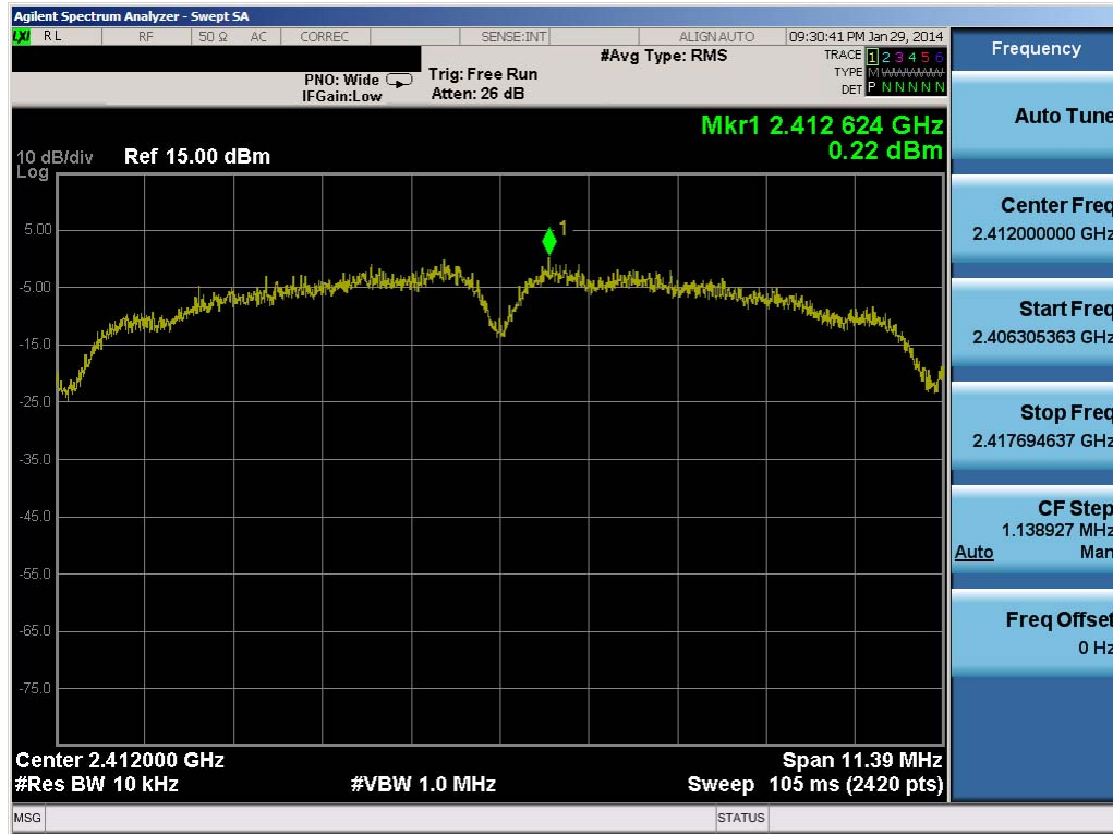
Plot 6-10. Power Spectral Density Plot (802.11b – Ch. 1)
