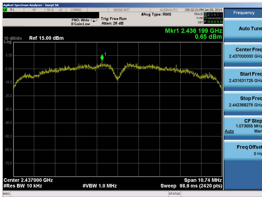
Plot 6-11. Power Spectral Density Plot (802.11b – Ch. 6)
