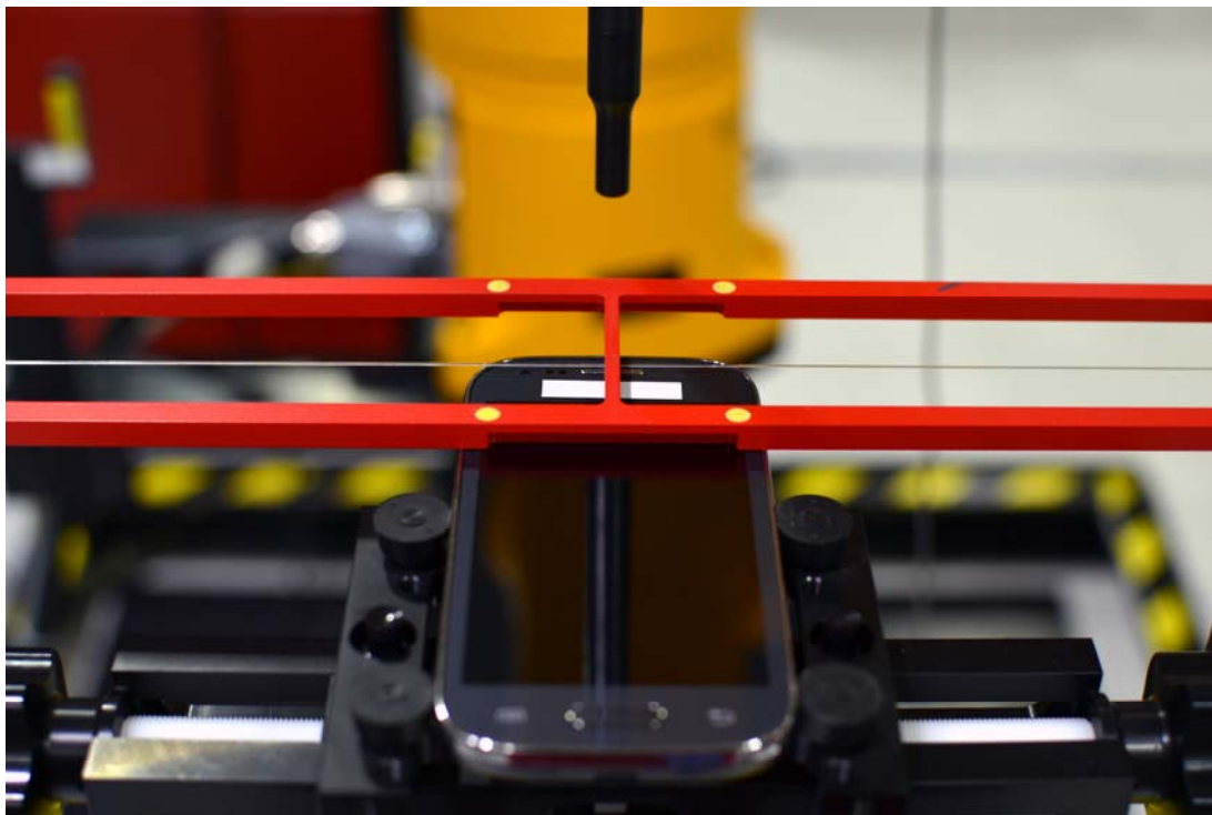
Figure 18-1 Ear Reference Point HAC Phantom Alignment
