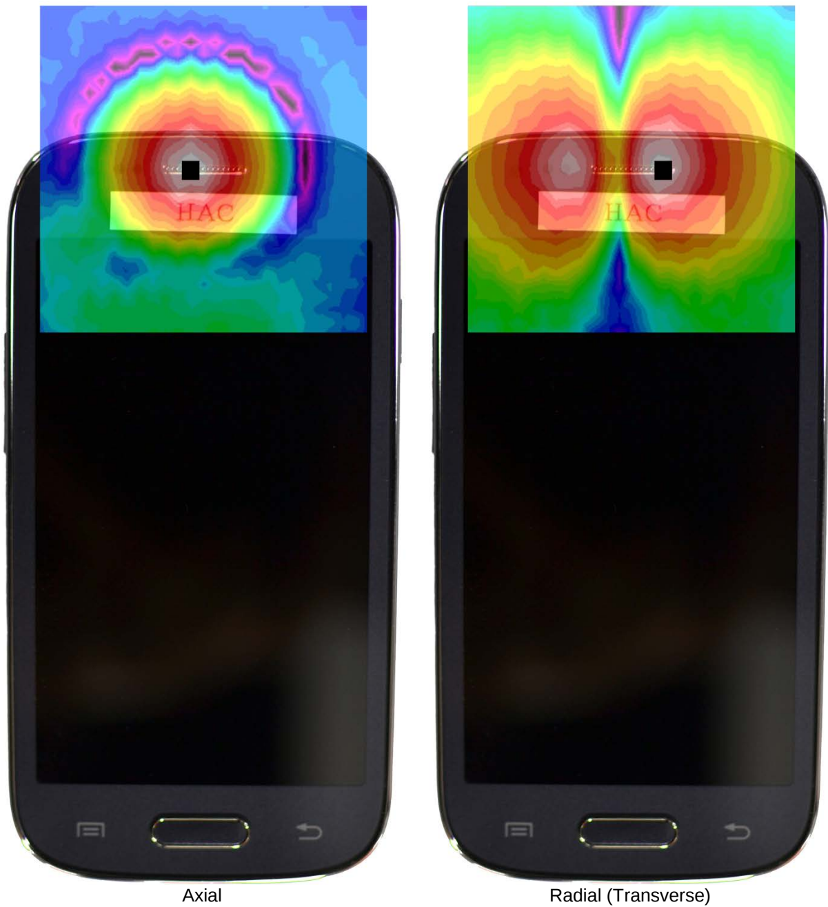
Figure 13-3 T-Coil Scan Overlay Magnetic Field Distributions
