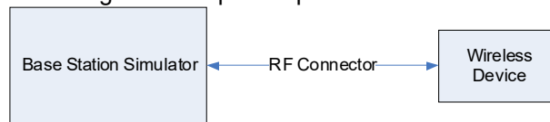
Figure 9-2 Power Measurement Setup
