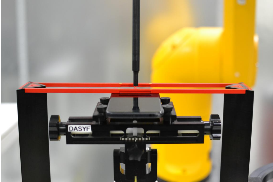
Figure 17-1 Ear Reference Point HAC Phantom Alignment
