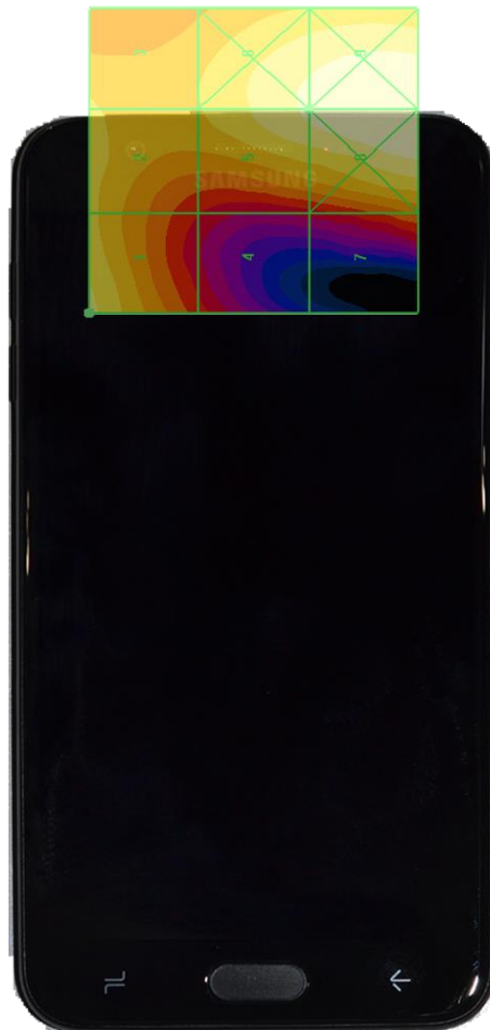
Figure 17-4 E-Field WD Scan overlay
