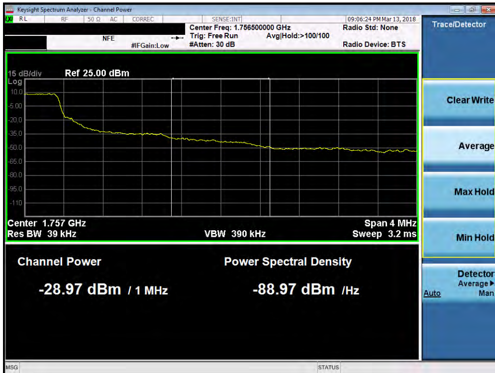
Plot 7-123. Upper Extended Band Edge Plot (Band 4 - 1.4MHz QPSK - Full RB Configuration)
