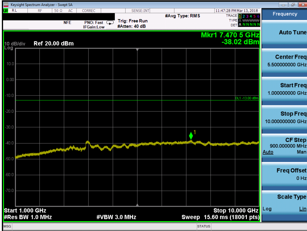
Plot 7-66. Conducted Spurious Plot (Band 12 - 3.0MHz QPSK - RB Size 1, RB Offset 0 - High Channel)
