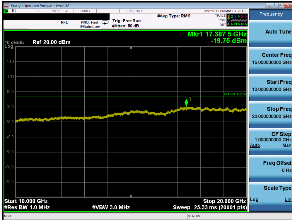
Plot 7-84. Conducted Spurious Plot (Band 66/4 - 20.0MHz QPSK - RB Size 1, RB Offset 0 - High Channel)
