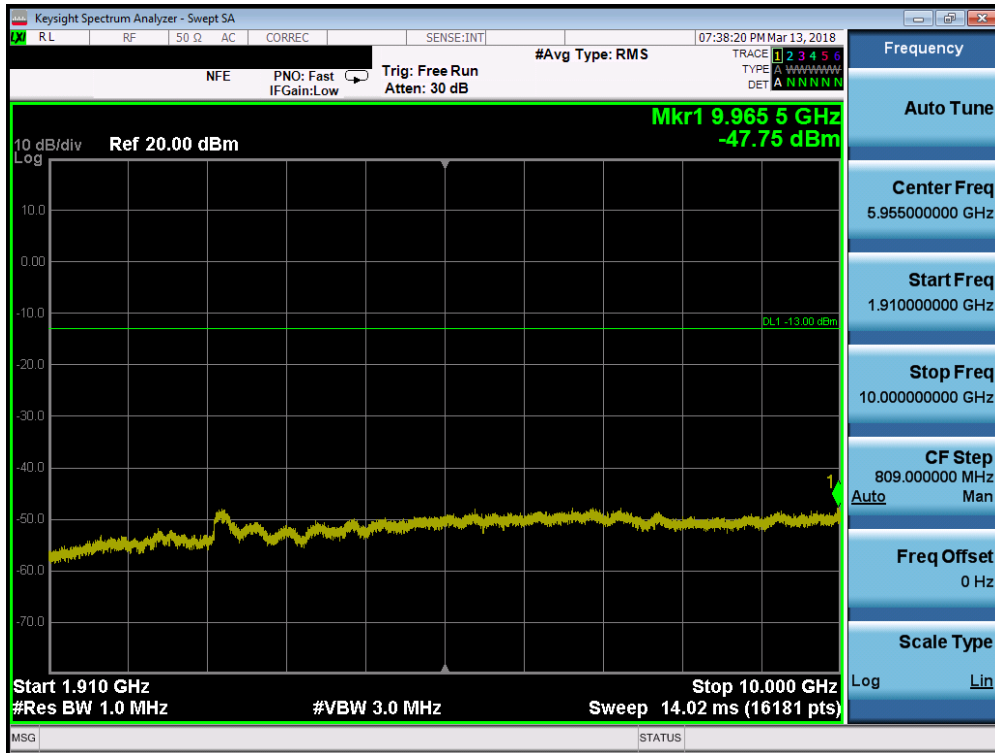
Plot 7-86. Conducted Spurious Plot (Band 2 - 5.0MHz QPSK - RB Size 1, RB Offset 0 - Low Channel)
