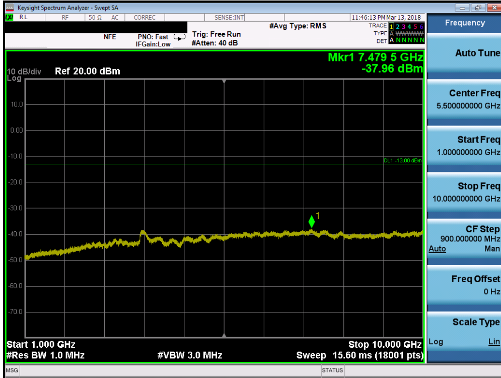
Plot 7-60. Conducted Spurious Plot (Band 12 - 3.0MHz QPSK - RB Size 1, RB Offset 0 - Low Channel)
