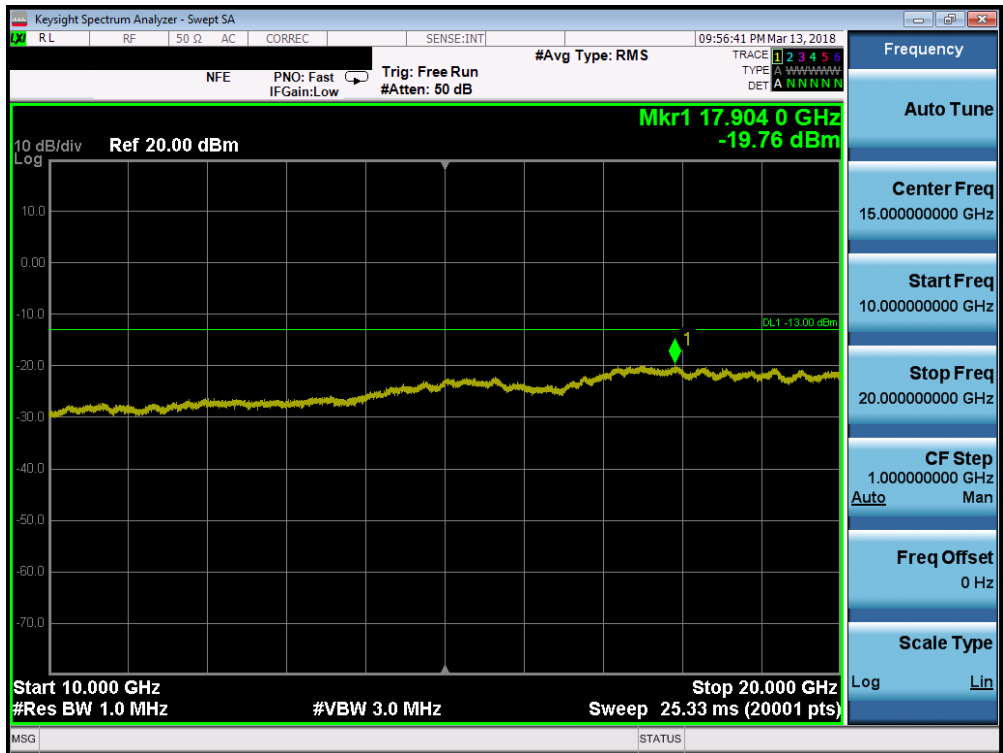
Plot 7-81. Conducted Spurious Plot (Band 66/4 - 20.0MHz QPSK - RB Size 1, RB Offset 0 - Mid Channel)
