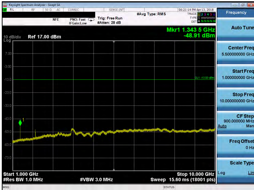
Plot 7-54. Conducted Spurious Plot (Band 71 - 20.0MHz QPSK - RB Size 1, RB Offset 0 - Mid Channel)
