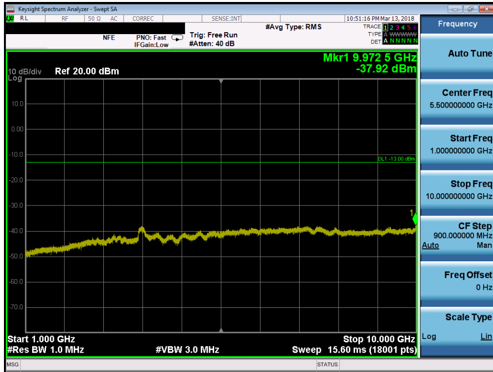
Plot 7-75. Conducted Spurious Plot (Band 5 - 3.0MHz QPSK - RB Size 1, RB Offset 0 - High Channel)
