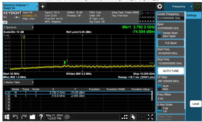
Sub6 n26. Conducted Spurious (164300 ch\_5 MHz\_ BPSK\_RB 1\_1)
