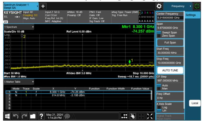
Sub6 n26. Conducted Spurious (163300 ch\_5 MHz\_ BPSK\_RB 1\_1)
