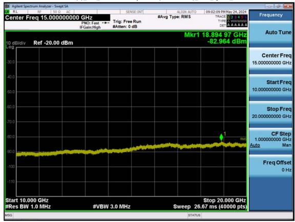
LTE B25(2)\_5 M\_Conducted Spurious(10 G-26.5 G)\_Low\_QPSK\_1RB
