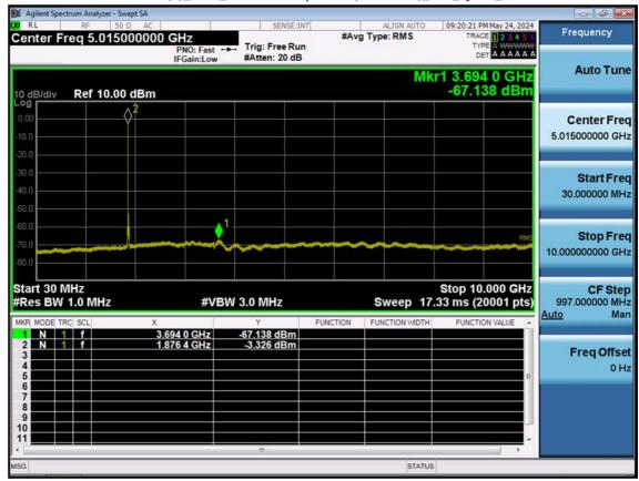
LTE B25(2)\_15 M\_Conducted Spurious(30 M-10 G)\_Mid\_QPSK\_1RB
