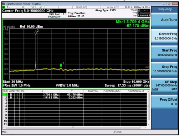
LTE B25(2)\_15 M\_Conducted Spurious(30 M-10 G)\_High\_QPSK\_1RB
