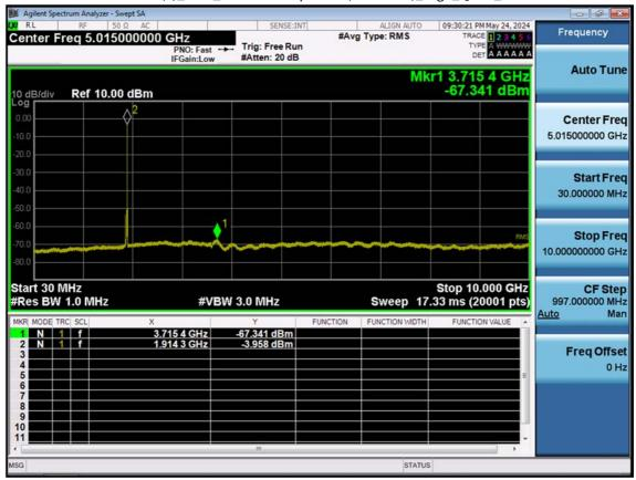
LTE B25(2)\_20 M\_Conducted Spurious(30 M-10 G)\_High\_QPSK\_1RB
