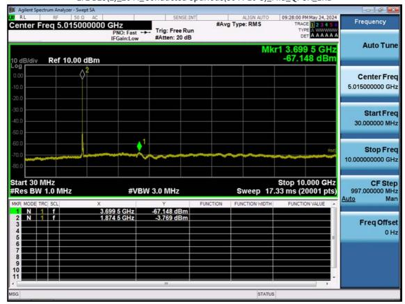
LTE B25(2)\_20 M\_Conducted Spurious(30 M-10 G)\_Mid\_QPSK\_1RB
