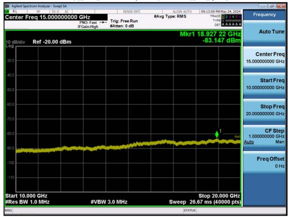
LTE B25(2)\_10 M\_Conducted Spurious(10 G-26.5 G)\_Mid\_QPSK\_1RB
