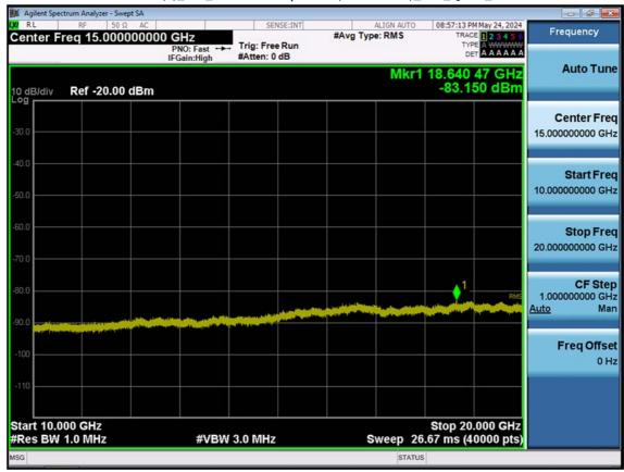
LTE B25(2)\_3 M\_Conducted Spurious(10 G-26.5 G)\_Mid\_QPSK\_1RB
