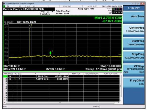
LTE B25(2)\_5 M\_Conducted Spurious(30 M-10 G)\_Mid\_QPSK\_1RB
