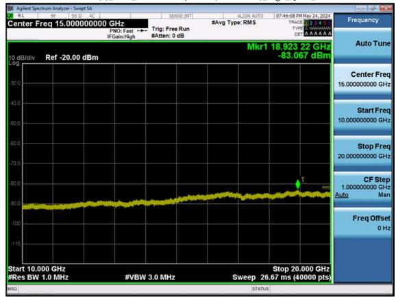
LTE B25(2)\_1.4M\_Conducted Spurious(10 G-26.5 G)\_High\_QPSK\_1RB
