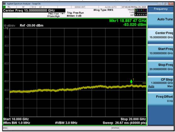
LTE B25(2)\_1.4M\_Conducted Spurious(10 G-26.5 G)\_Low\_QPSK\_1RB
