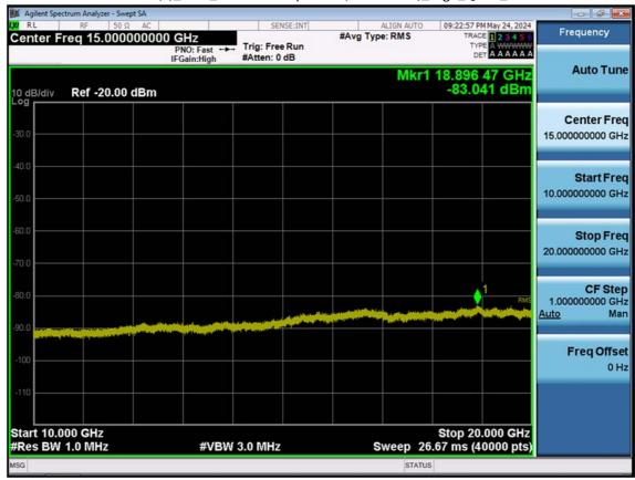
LTE B25(2)\_15 M\_Conducted Spurious(10 G-26.5 G)\_High\_QPSK\_1RB
