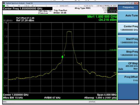
LTE B25(2)\_1.4M\_Band Edge\_Low\_QPSK\_1RB
