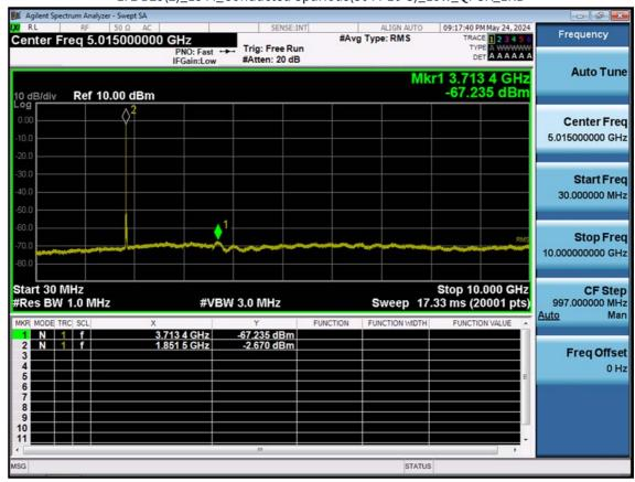
LTE B25(2)\_15 M\_Conducted Spurious(30 M-10 G)\_Low\_QPSK\_1RB
