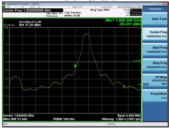
LTE B25(2)\_5 M\_Band Edge\_Low\_QPSK\_1RB
