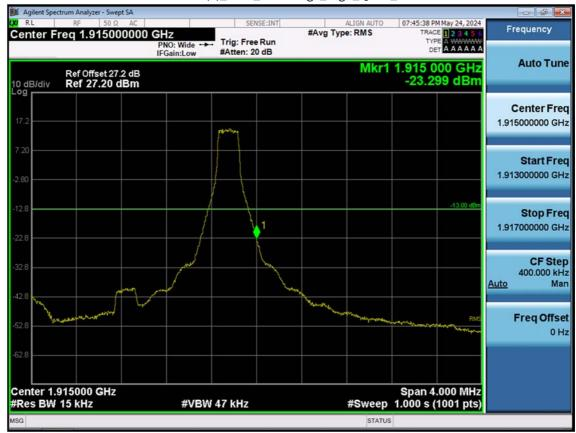
LTE B25(2)\_1.4M\_Band Edge\_High\_QPSK\_1RB
