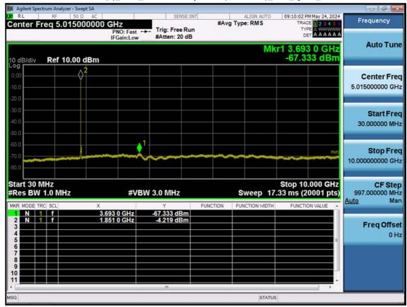
LTE B25(2)\_10 M\_Conducted Spurious(30 M-10 G)\_Low\_QPSK\_1RB
