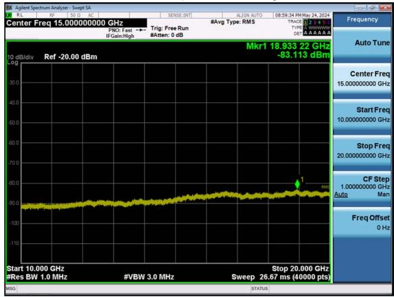
LTE B25(2)\_3 M\_Conducted Spurious(10 G-26.5 G)\_High\_QPSK\_1RB
