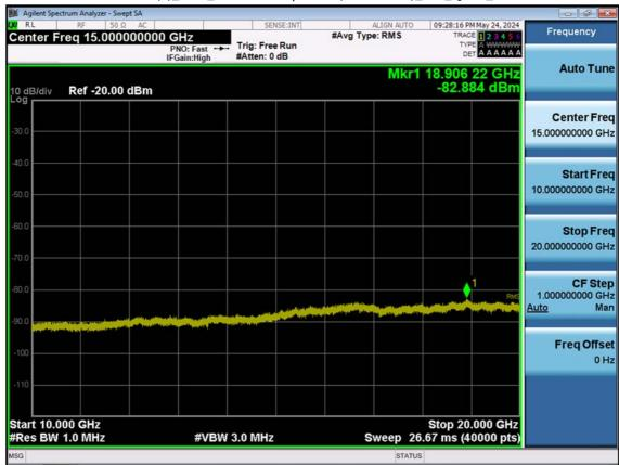
LTE B25(2)\_20 M\_Conducted Spurious(10 G-26.5 G)\_Mid\_QPSK\_1RB
