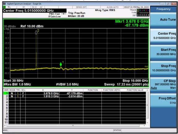
LTE B25(2)\_5 M\_Conducted Spurious(30 M-10 G)\_High\_QPSK\_1RB
