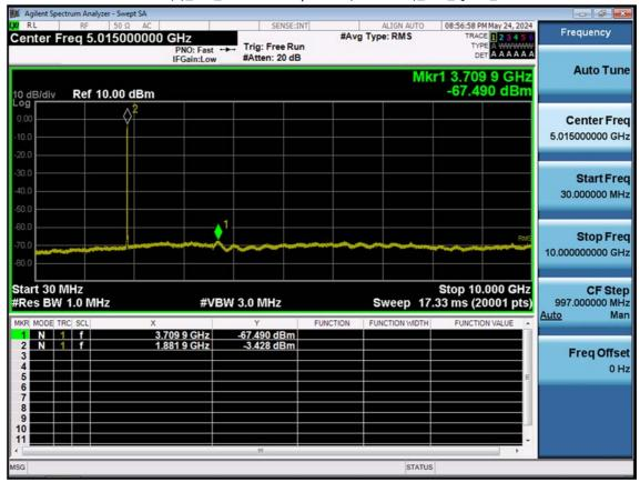
LTE B25(2)\_3 M\_Conducted Spurious(30 M-10 G)\_Mid\_QPSK\_1RB
