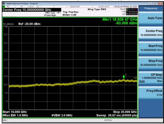
LTE B25(2)\_15 M\_Conducted Spurious(10 G-26.5 G)\_Mid\_QPSK\_1RB
