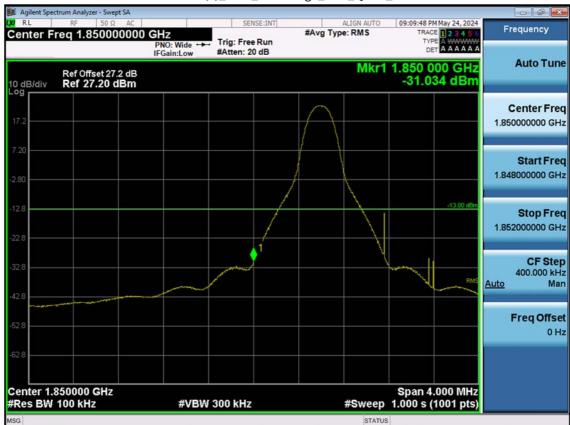
LTE B25(2)\_10 M\_Band Edge\_Low\_QPSK\_1RB
