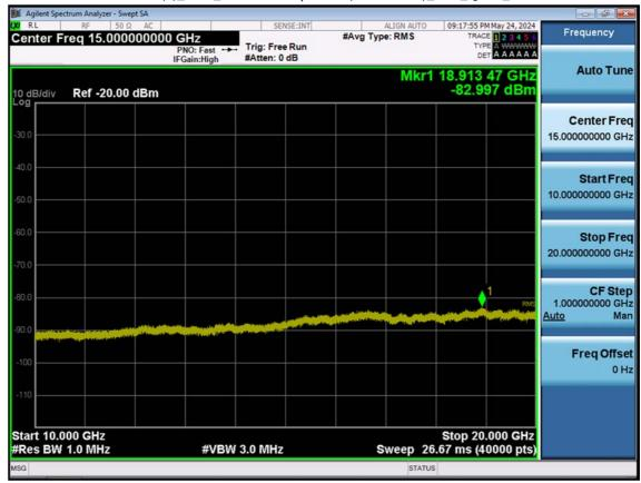
LTE B25(2)\_15 M\_Conducted Spurious(10 G-26.5 G)\_Low\_QPSK\_1RB
