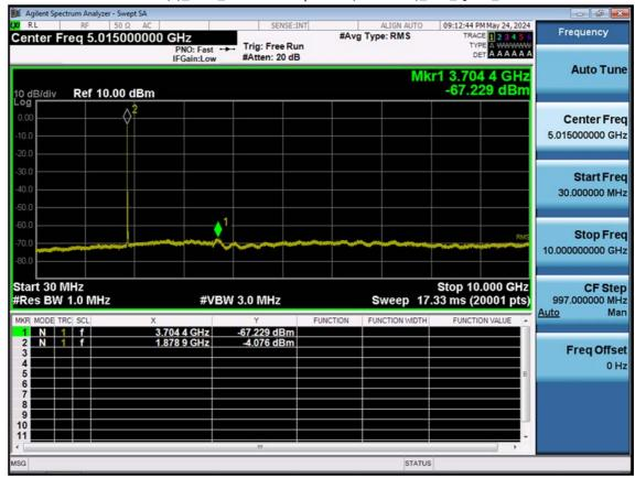
LTE B25(2)\_10 M\_Conducted Spurious(30 M-10 G)\_Mid\_QPSK\_1RB
