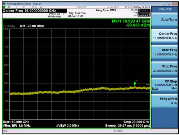
LTE B25(2)\_1.4M\_Conducted Spurious(10 G-26.5 G)\_Mid\_QPSK\_1RB
