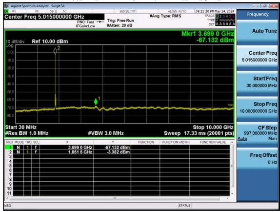
LTE B25(2)\_20 M\_Conducted Spurious(30 M-10 G)\_Low\_QPSK\_1RB
