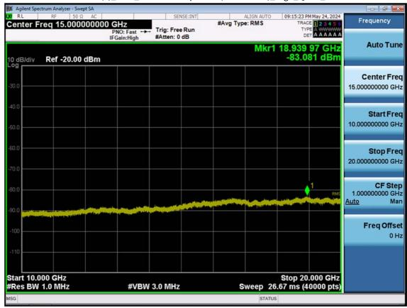
LTE B25(2)\_10 M\_Conducted Spurious(10 G-26.5 G)\_High\_QPSK\_1RB
