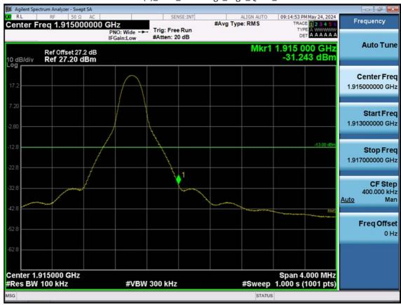
LTE B25(2)\_10 M\_Band Edge\_High\_QPSK\_1RB
