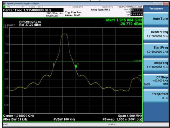
LTE B25(2)\_5 M\_Band Edge\_High\_QPSK\_1RB
