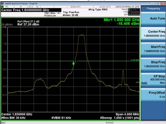
LTE B25(2)\_3 M\_Band Edge\_Low\_QPSK\_1RB
