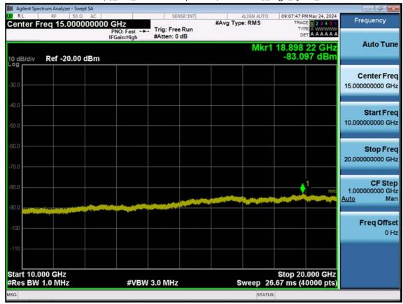
LTE B25(2)\_5 M\_Conducted Spurious(10 G-26.5 G)\_High\_QPSK\_1RB
