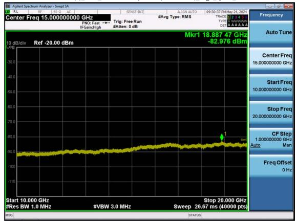
LTE B25(2)\_20 M\_Conducted Spurious(10 G-26.5 G)\_High\_QPSK\_1RB
