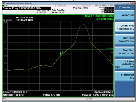
LTE B25(2)\_15 M\_Band Edge\_Low\_QPSK\_1RB
