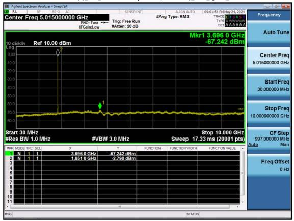
LTE B25(2)\_5 M\_Conducted Spurious(30 M-10 G)\_Low\_QPSK\_1RB
