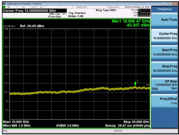
LTE B25(2)\_3 M\_Conducted Spurious(10 G-26.5 G)\_Low\_QPSK\_1RB
