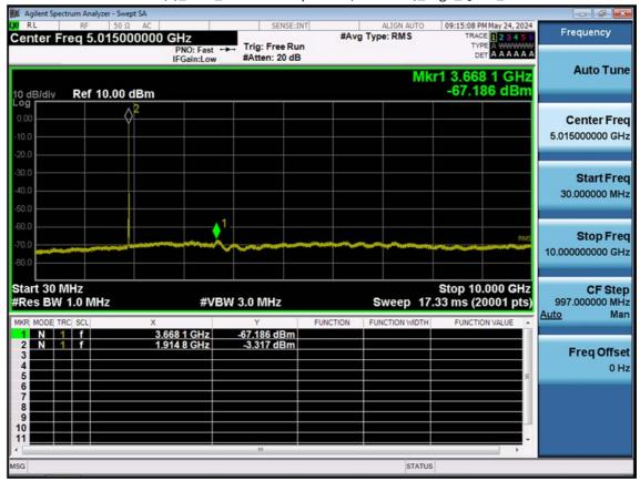
LTE B25(2)\_10 M\_Conducted Spurious(30 M-10 G)\_High\_QPSK\_1RB
