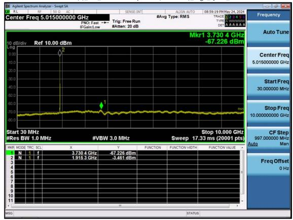
LTE B25(2)\_3 M\_Conducted Spurious(30 M-10 G)\_High\_QPSK\_1RB
