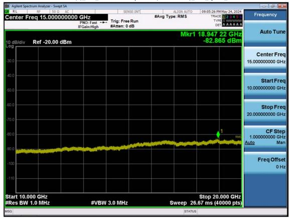
LTE B25(2)\_5 M\_Conducted Spurious(10 G-26.5 G)\_Mid\_QPSK\_1RB
