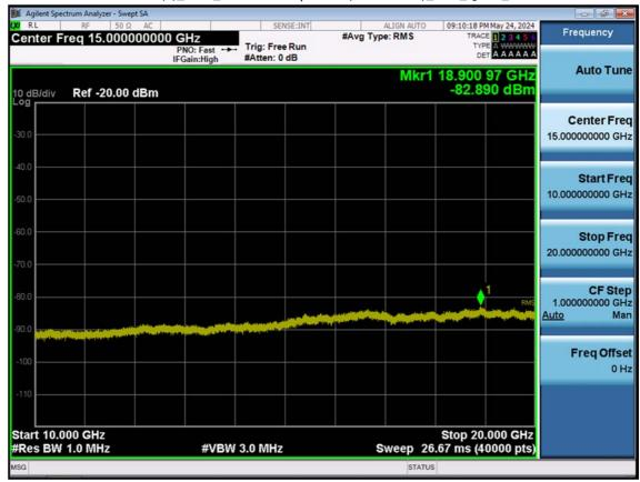
LTE B25(2)\_10 M\_Conducted Spurious(10 G-26.5 G)\_Low\_QPSK\_1RB
