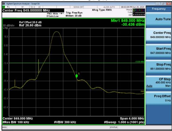
LTE B5\_10 M\_Band Edge\_High\_QPSK\_1RB
