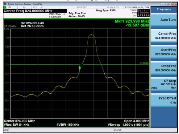
LTE B5\_5 M\_Band Edge\_Low\_QPSK\_1RB
