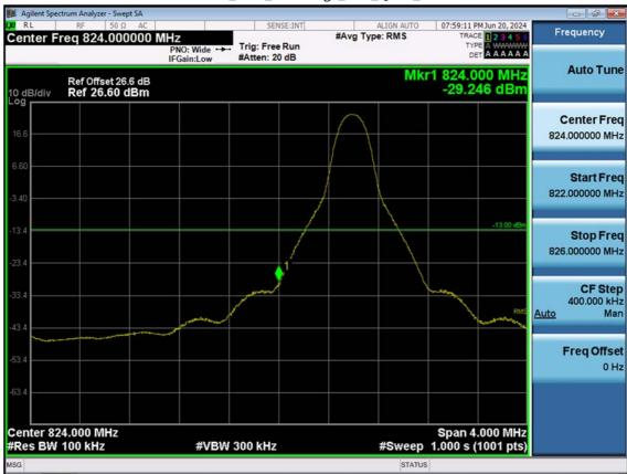
LTE B5\_10 M\_Band Edge\_Low\_QPSK\_1RB
