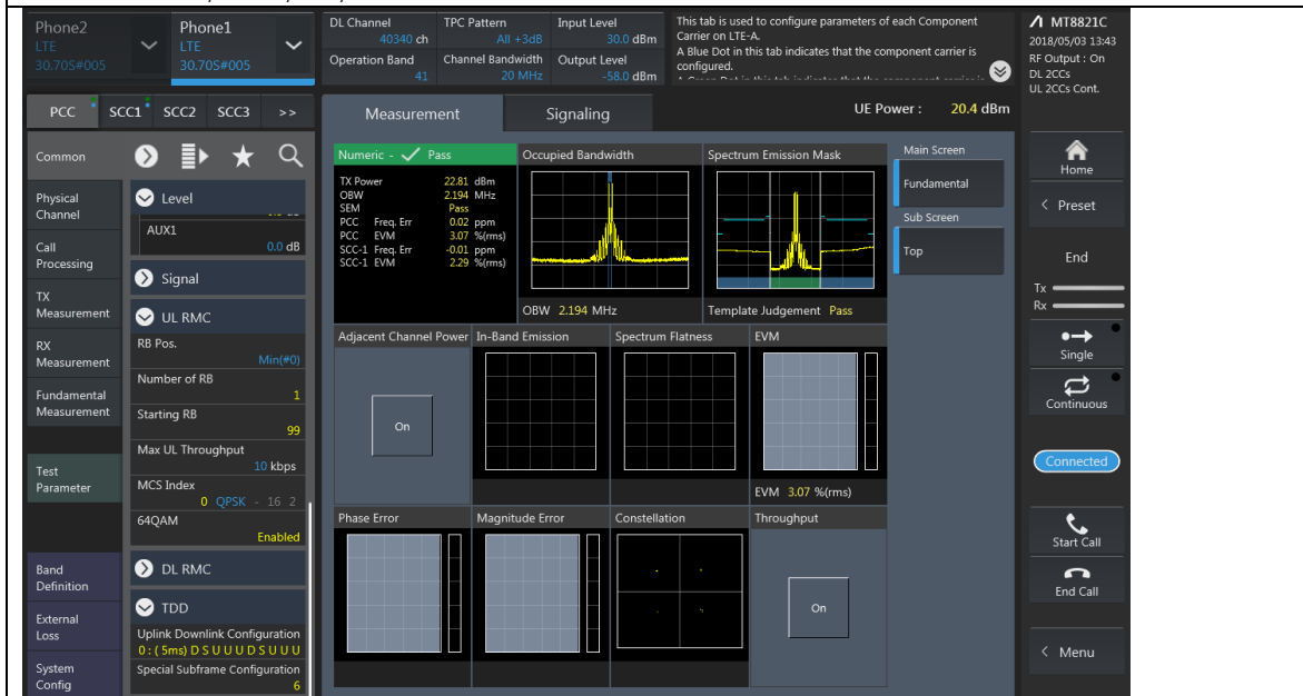
Call 5: Set to RB, offset, BW, modulation and Max Power conditions of PCC required test channel.
