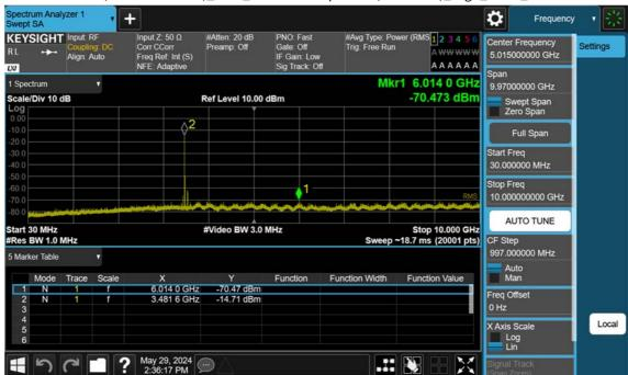
n77(3450~3550 MHz)\_70 M\_Conducted Spurious(30 M-10 G)\_High\_BPSK\_1RB
