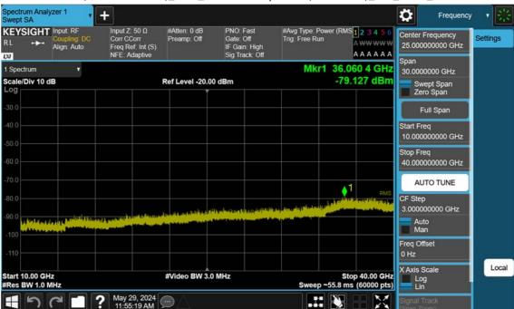
n77(3450~3550 MHz)\_10 M\_Conducted Spurious(Above10 G)\_Mid\_BPSK\_1RB
