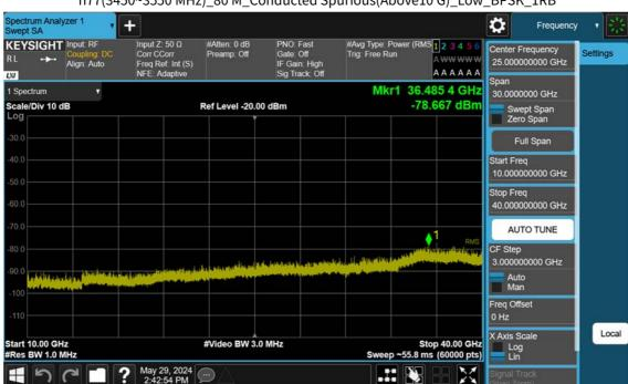
n77(3450~3550 MHz)\_80 M\_Conducted Spurious(Above10 G)\_Low\_BPSK\_1RB
