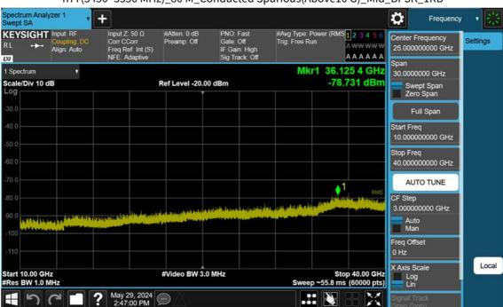
n77(3450~3550 MHz)\_80 M\_Conducted Spurious(Above10 G)\_Mid\_BPSK\_1RB
