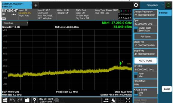
n77(3450~3550 MHz)\_70 M\_Conducted Spurious(Above10 G)\_High\_BPSK\_1RB
