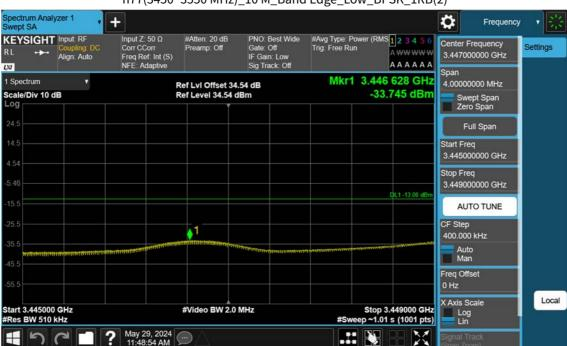
n77(3450~3550 MHz)\_10 M\_Band Edge\_Low\_BPSK\_1RB(2)
