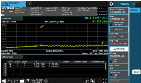
n77(3450~3550 MHz)\_90 M\_Conducted Spurious(30 M-10 G)\_Mid\_BPSK\_1RB
