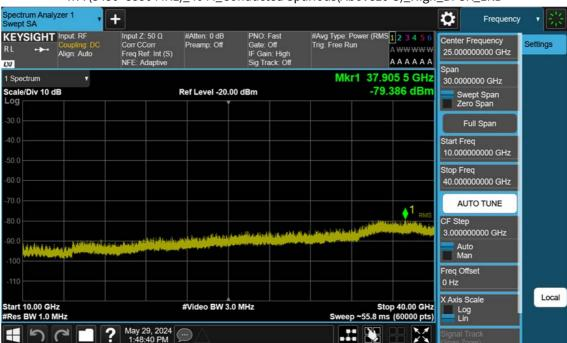
n77(3450~3550 MHz)\_40 M\_Conducted Spurious(Above10 G)\_High\_BPSK\_1RB
