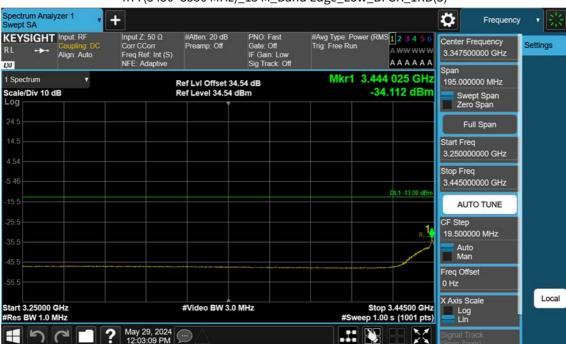
n77(3450~3550 MHz)\_15 M\_Band Edge\_Low\_BPSK\_1RB(3)
