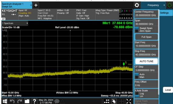
n77(3450~3550 MHz)\_60 M\_Conducted Spurious(Above10 G)\_Mid\_BPSK\_1RB
