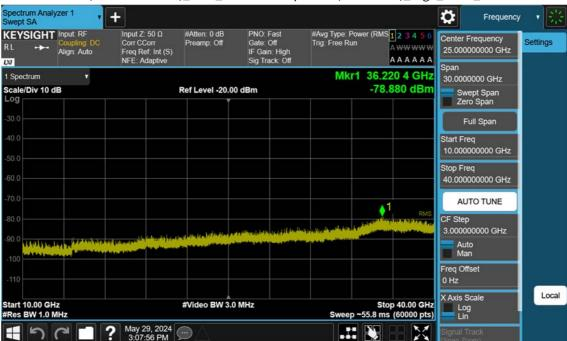
n77(3450~3550 MHz)\_90 M\_Conducted Spurious(Above10 G)\_High\_BPSK\_1RB
