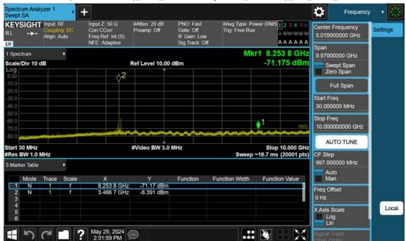
n77(3450~3550 MHz)\_70 M\_Conducted Spurious(30 M-10 G)\_Mid\_BPSK\_1RB
