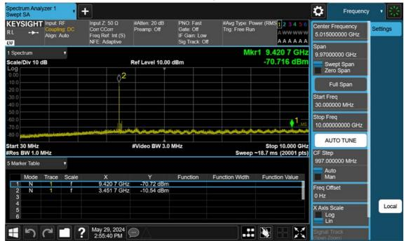
n77(3450~3550 MHz)\_90 M\_Conducted Spurious(30 M-10 G)\_Low\_BPSK\_1RB
