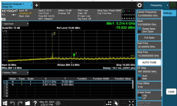
n77(3450~3550 MHz)\_50 M\_Conducted Spurious(30 M-10 G)\_High\_BPSK\_1RB
