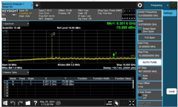
n77(3450~3550 MHz)\_60 M\_Conducted Spurious(30 M-10 G)\_Low\_BPSK\_1RB
