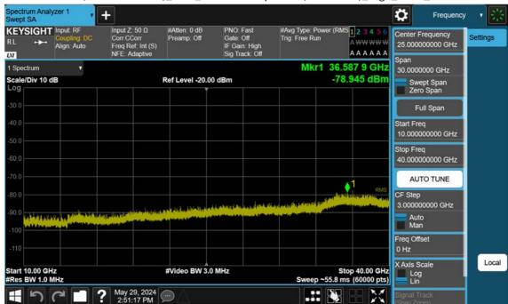
n77(3450~3550 MHz)\_80 M\_Conducted Spurious(Above10 G)\_High\_BPSK\_1RB
