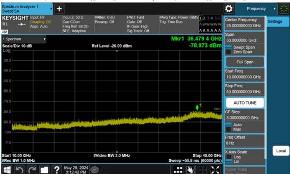
n77(3450~3550 MHz)\_100 M\_Conducted Spurious(Above10 G)\_Low\_BPSK\_1RB
