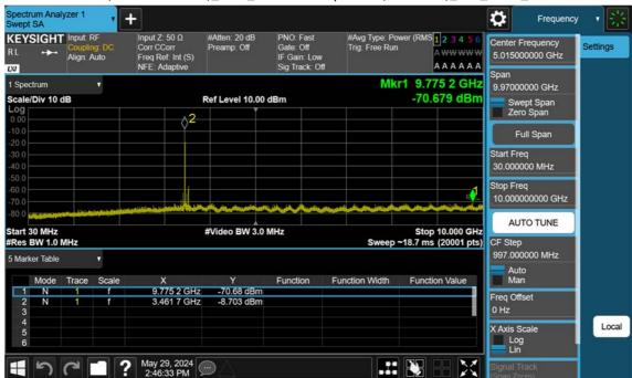
n77(3450~3550 MHz)\_80 M\_Conducted Spurious(30 M-10 G)\_Mid\_BPSK\_1RB
