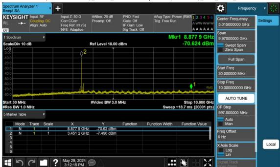
n77(3450~3550 MHz)\_100 M\_Conducted Spurious(30 M-10 G)\_Low\_BPSK\_1RB
