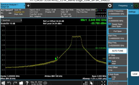
n77(3450~3550 MHz)\_15 M\_Band Edge\_Low\_BPSK\_1RB(1)
