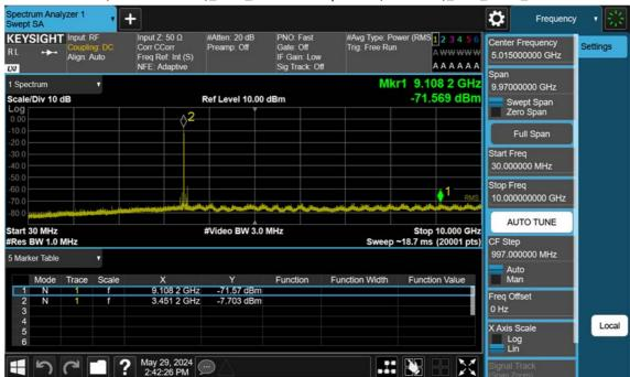
n77(3450~3550 MHz)\_80 M\_Conducted Spurious(30 M-10 G)\_Low\_BPSK\_1RB
