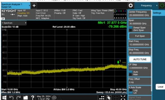
n77(3450~3550 MHz)\_25 M\_Conducted Spurious(Above10 G)\_Mid\_BPSK\_1RB
