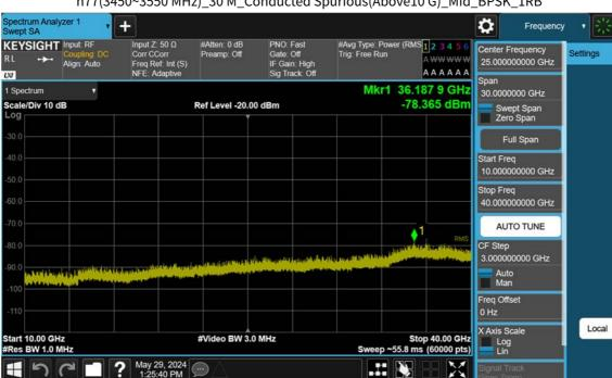
n77(3450~3550 MHz)\_30 M\_Conducted Spurious(Above10 G)\_Mid\_BPSK\_1RB
