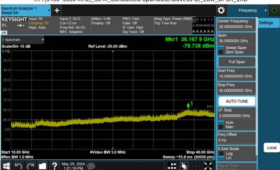
n77(3450~3550 MHz)\_30 M\_Conducted Spurious(Above10 G)\_Low\_BPSK\_1RB
