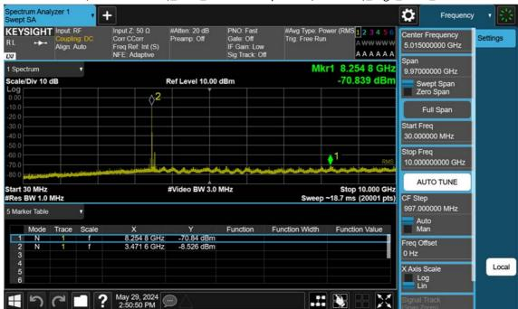
n77(3450~3550 MHz)\_80 M\_Conducted Spurious(30 M-10 G)\_High\_BPSK\_1RB
