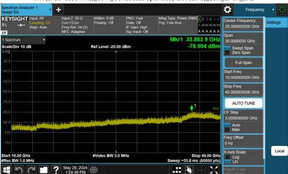
n77(3450~3550 MHz)\_50 M\_Conducted Spurious(Above10 G)\_Low\_BPSK\_1RB
