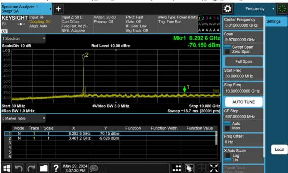
n77(3450~3550 MHz)\_90 M\_Conducted Spurious(30 M-10 G)\_High\_BPSK\_1RB
