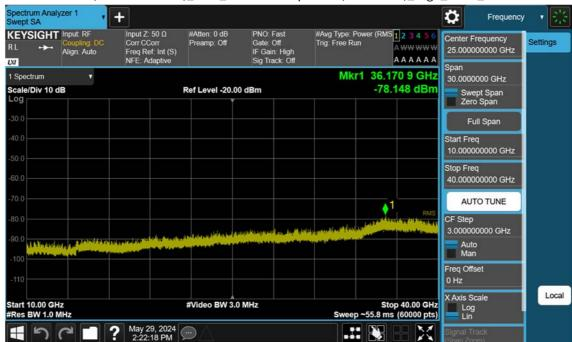
n77(3450~3550 MHz)\_60 M\_Conducted Spurious(Above10 G)\_High\_BPSK\_1RB
