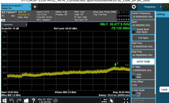
n77(3450~3550 MHz)\_40 M\_Conducted Spurious(Above10 G)\_Low\_BPSK\_1RB
