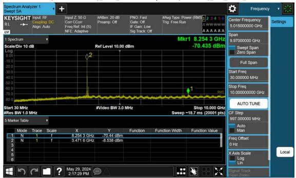
n77(3450~3550 MHz)\_60 M\_Conducted Spurious(30 M-10 G)\_Mid\_BPSK\_1RB
