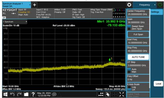
n77(3450~3550 MHz)\_15 M\_Conducted Spurious(Above10 G)\_Low\_BPSK\_1RB
