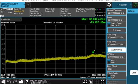
n77(3450~3550 MHz)\_60 M\_Conducted Spurious(Above10 G)\_Low\_BPSK\_1RB
