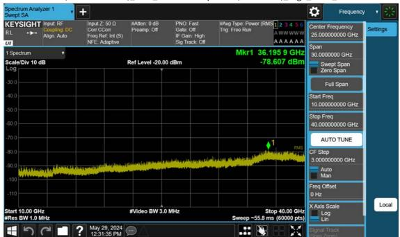
n77(3450~3550 MHz)\_15 M\_Conducted Spurious(Above10 G)\_High\_BPSK\_1RB
