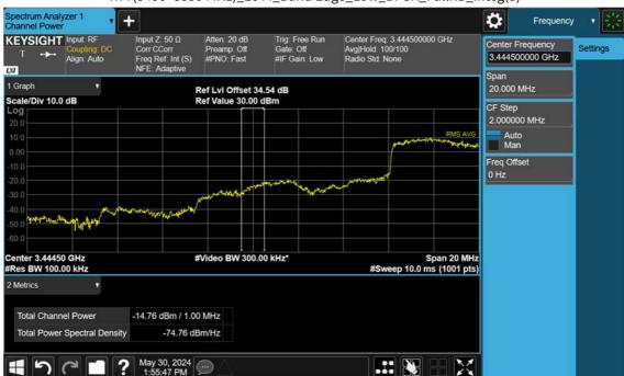
n77(3450~3550 MHz)\_10 M\_Band Edge\_Low\_BPSK\_FullRB\_integ(3)
