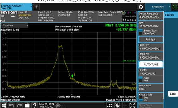
n77(3450~3550 MHz)\_10 M\_Band Edge\_High\_BPSK\_1RB(1)
