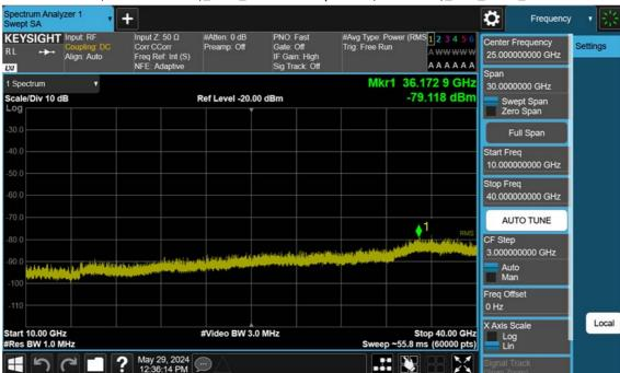
n77(3450~3550 MHz)\_20 M\_Conducted Spurious(Above10 G)\_Low\_BPSK\_1RB
