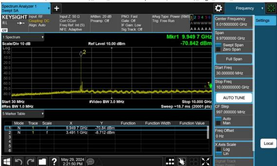
n77(3450~3550 MHz)\_60 M\_Conducted Spurious(30 M-10 G)\_High\_BPSK\_1RB
