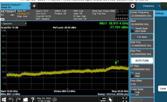
n77(3450~3550 MHz)\_10 M\_Conducted Spurious(Above10 G)\_Low\_BPSK\_1RB
