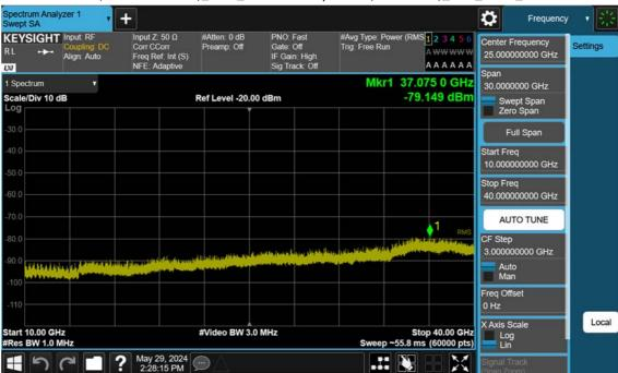
n77(3450~3550 MHz)\_70 M\_Conducted Spurious(Above10 G)\_Low\_BPSK\_1RB
