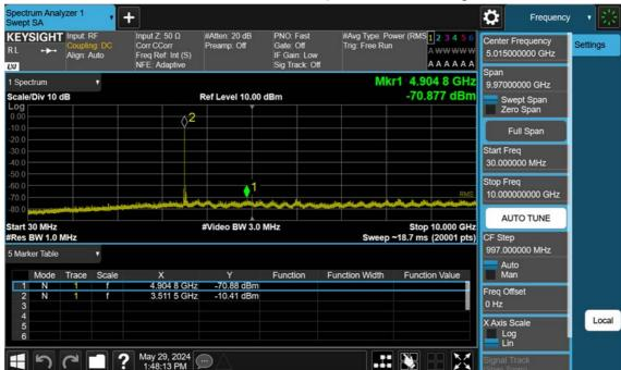
n77(3450~3550 MHz)\_40 M\_Conducted Spurious(30 M-10 G)\_High\_BPSK\_1RB
