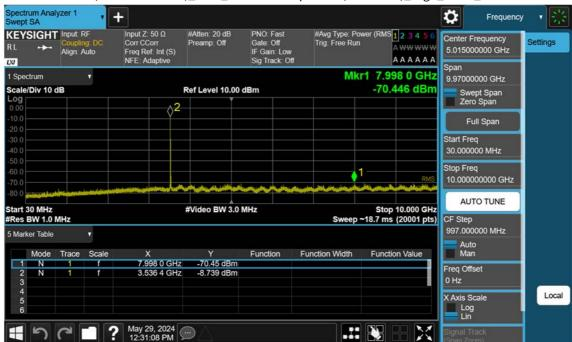
n77(3450~3550 MHz)\_15 M\_Conducted Spurious(30 M-10 G)\_High\_BPSK\_1RB
