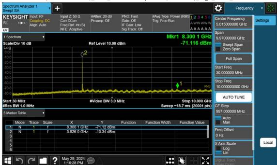
n77(3450~3550 MHz)\_25 M\_Conducted Spurious(30 M-10 G)\_High\_BPSK\_1RB
