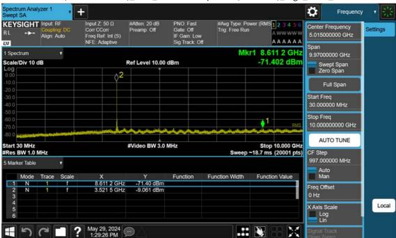
n77(3450~3550 MHz)\_30 M\_Conducted Spurious(30 M-10 G)\_High\_BPSK\_1RB
