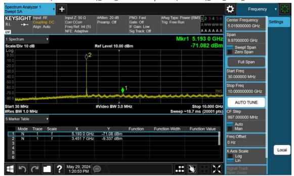
n77(3450~3550 MHz)\_30 M\_Conducted Spurious(30 M-10 G)\_Low\_BPSK\_1RB
