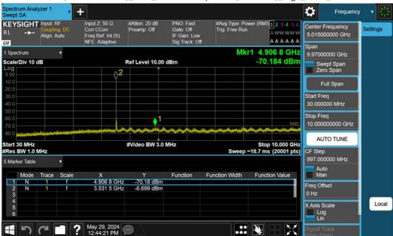
n77(3450~3550 MHz)\_20 M\_Conducted Spurious(30 M-10 G)\_High\_BPSK\_1RB
