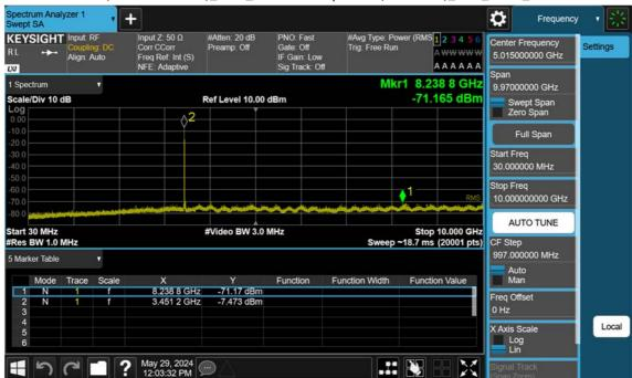
n77(3450~3550 MHz)\_15 M\_Conducted Spurious(30 M-10 G)\_Low\_BPSK\_1RB
