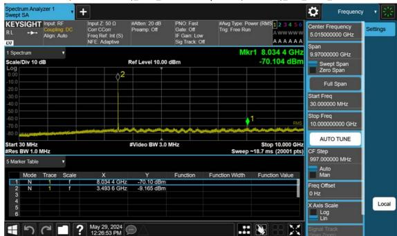
n77(3450~3550 MHz)\_15 M\_Conducted Spurious(30 M-10 G)\_Mid\_BPSK\_1RB
