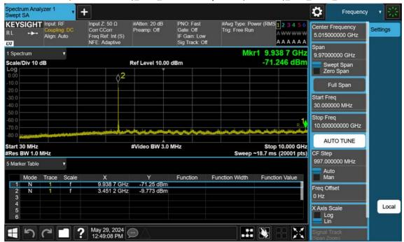
n77(3450~3550 MHz)\_25 M\_Conducted Spurious(30 M-10 G)\_Low\_BPSK\_1RB
