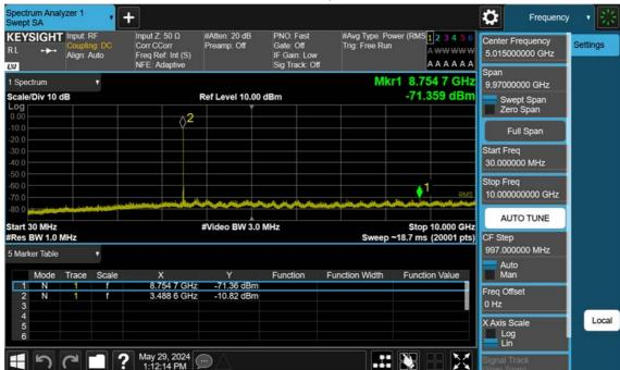
n77(3450~3550 MHz)\_25 M\_Conducted Spurious(30 M-10 G)\_Mid\_BPSK\_1RB
