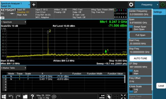
n77(3450~3550 MHz)\_50 M\_Conducted Spurious(30 M-10 G)\_Low\_BPSK\_1RB
