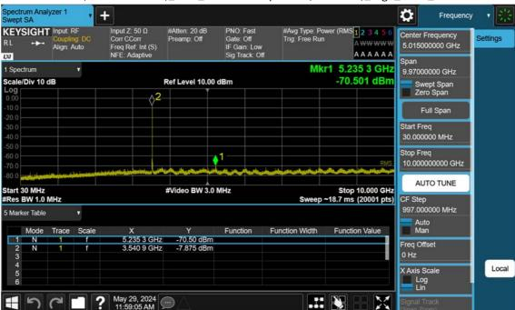
n77(3450~3550 MHz)\_10 M\_Conducted Spurious(30 M-10 G)\_High\_BPSK\_1RB
