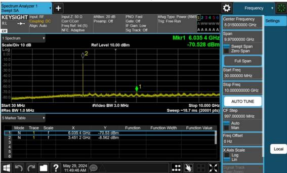
n77(3450~3550 MHz)\_10 M\_Conducted Spurious(30 M-10 G)\_Low\_BPSK\_1RB
