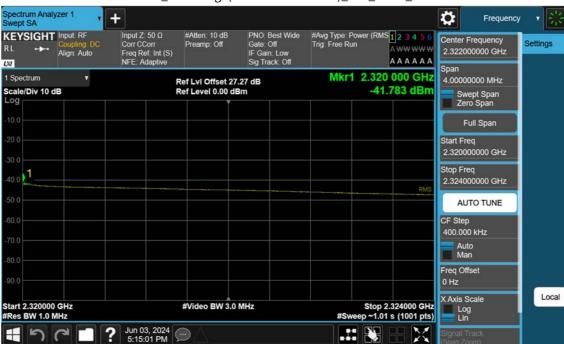
10 M\_Band Edge(2320MHz-2324MHz)\_Mid\_BPSK\_1RB
