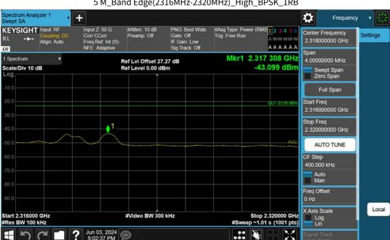
5 M\_Band Edge(2316MHz-2320MHz)\_High\_BPSK\_1RB
