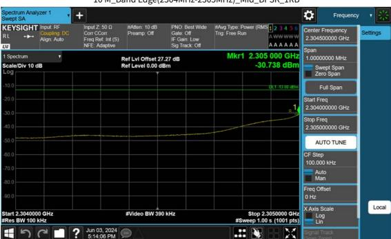
10 M\_Band Edge(2304MHz-2305MHz)\_Mid\_BPSK\_1RB
