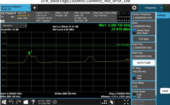
10 M\_Band Edge(2300MHz-2304MHz)\_Mid\_BPSK\_1RB
