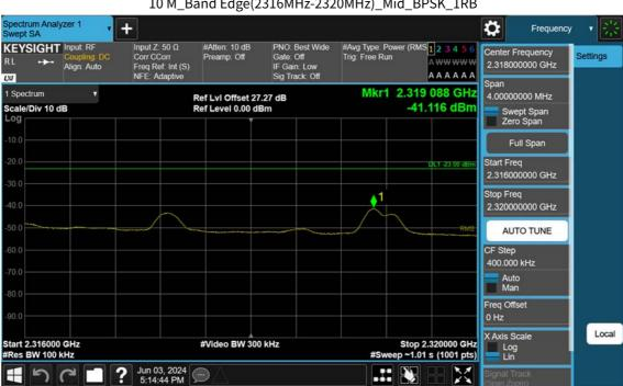
10 M\_Band Edge(2316MHz-2320MHz)\_Mid\_BPSK\_1RB
