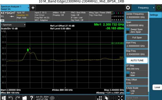
10 M\_Band Edge(2300MHz-2304MHz)\_Mid\_BPSK\_1RB
