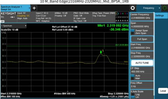
10 M\_Band Edge(2316MHz-2320MHz)\_Mid\_BPSK\_1RB
