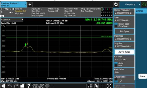
5 M\_Band Edge(2316MHz-2320MHz)\_High\_BPSK\_1RB
