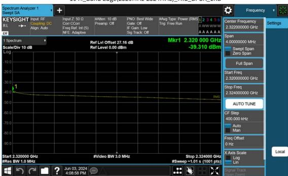
10 M\_Band Edge(2320MHz-2324MHz)\_Mid\_BPSK\_1RB
