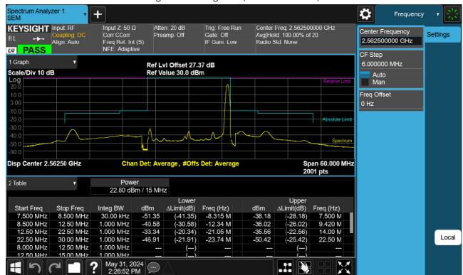
High Channel Edge Plot (15 MHz BPSK RB 1)
