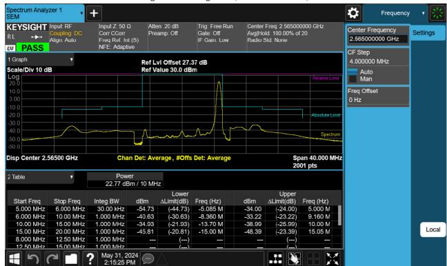
High Channel Edge Plot (10 MHz BPSK RB 1)
