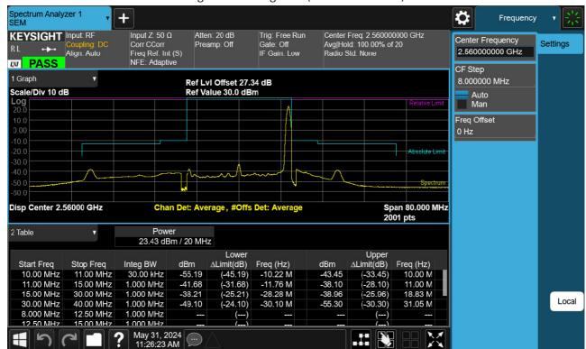
High Channel Edge Plot (20 MHz BPSK RB 1)
