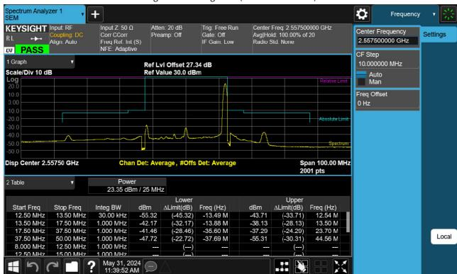
High Channel Edge Plot (25 MHz BPSK RB 1)
