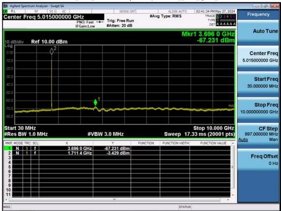
LTE B66\_10 M\_Conducted Spurious(30 M-10 G)\_Low\_QPSK\_1RB
