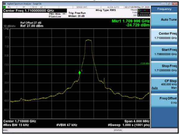
LTE B66\_1.4M\_Band Edge\_Low\_QPSK\_1RB
