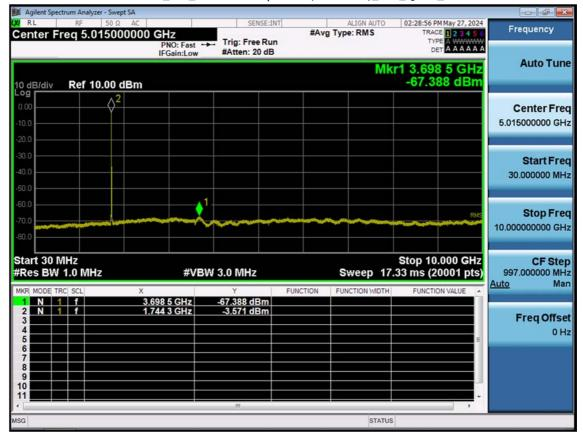
LTE B66\_3 M\_Conducted Spurious(30 M-10 G)\_Mid\_QPSK\_1RB
