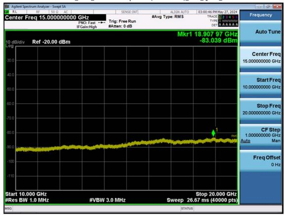
LTE B66\_20 M\_Conducted Spurious(10 G-26.5 G)\_Low\_QPSK\_1RB
