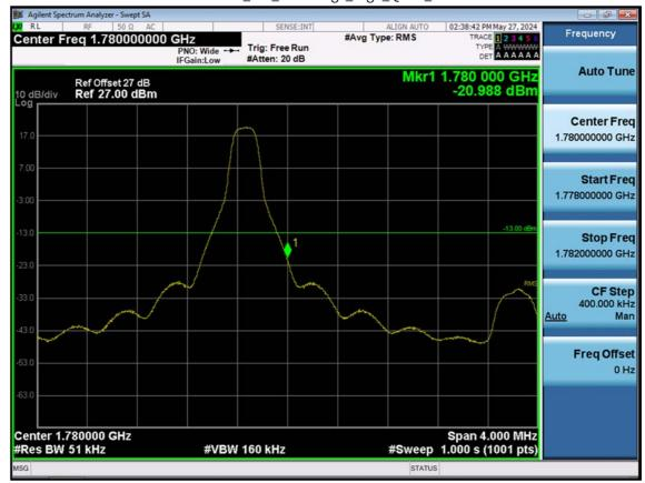
LTE B66\_5 M\_Band Edge\_High\_QPSK\_1RB
