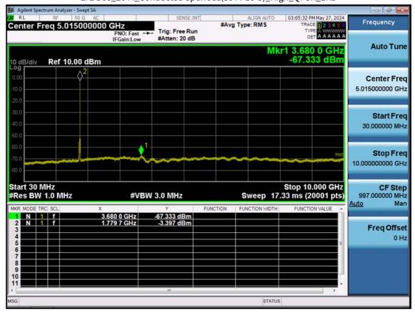
LTE B66\_20 M\_Conducted Spurious(30 M-10 G)\_High\_QPSK\_1RB
