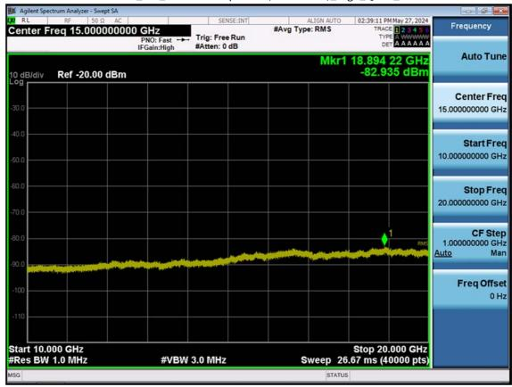
LTE B66\_5 M\_Conducted Spurious(10 G-26.5 G)\_High\_QPSK\_1RB
