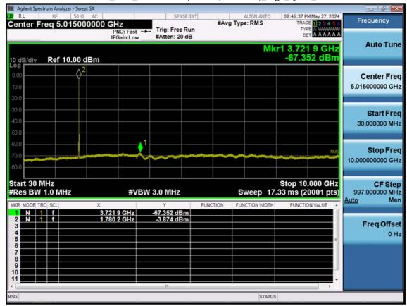
LTE B66\_10 M\_Conducted Spurious(30 M-10 G)\_High\_QPSK\_1RB
