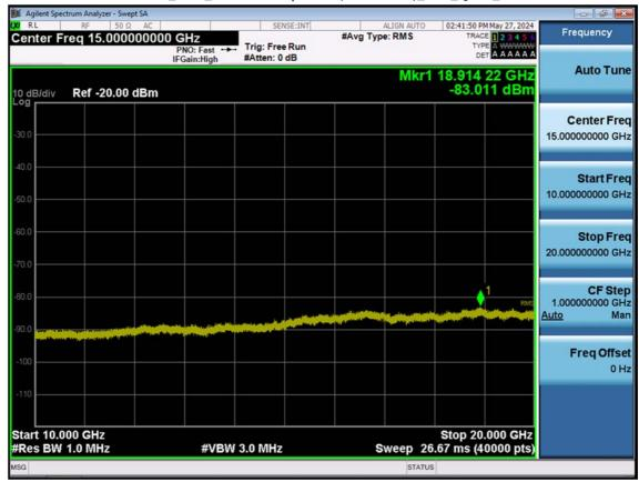
LTE B66\_10 M\_Conducted Spurious(10 G-26.5 G)\_Low\_QPSK\_1RB
