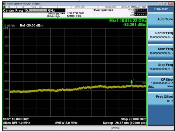
LTE B66\_5 M\_Conducted Spurious(10 G-26.5 G)\_Mid\_QPSK\_1RB
