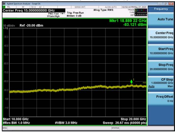
LTE B66\_15 M\_Conducted Spurious(10 G-26.5 G)\_Mid\_QPSK\_1RB
