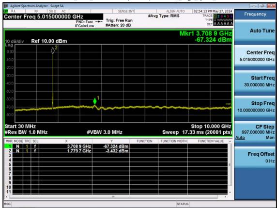
LTE B66\_15 M\_Conducted Spurious(30 M-10 G)\_High\_QPSK\_1RB
