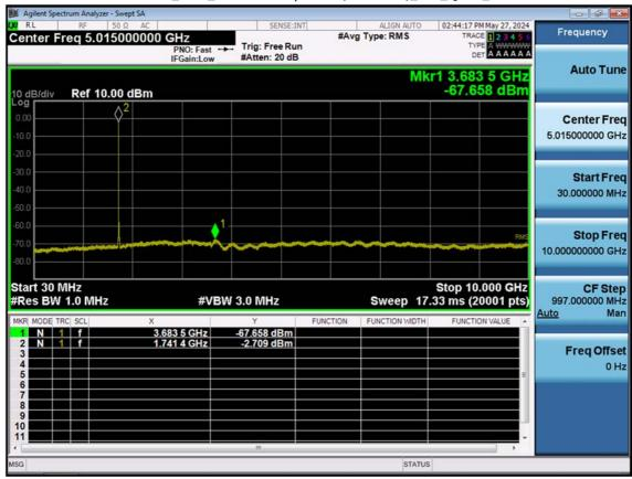
LTE B66\_10 M\_Conducted Spurious(30 M-10 G)\_Mid\_QPSK\_1RB
