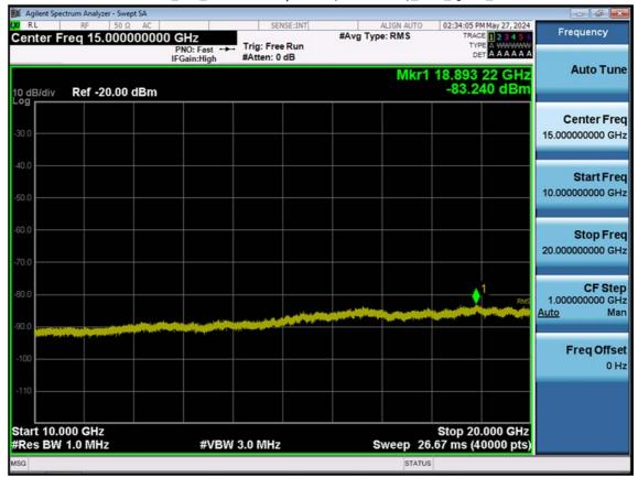
LTE B66\_5 M\_Conducted Spurious(10 G-26.5 G)\_Low\_QPSK\_1RB
