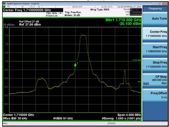
LTE B66\_3 M\_Band Edge\_Low\_QPSK\_1RB
