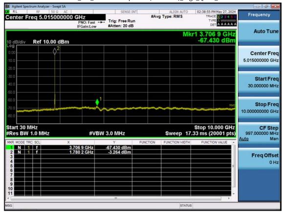
LTE B66\_5 M\_Conducted Spurious(30 M-10 G)\_High\_QPSK\_1RB
