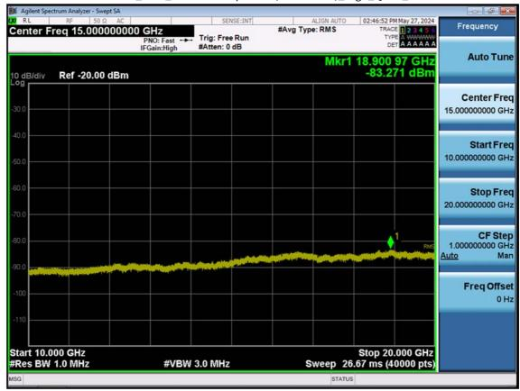
LTE B66\_10 M\_Conducted Spurious(10 G-26.5 G)\_High\_QPSK\_1RB
