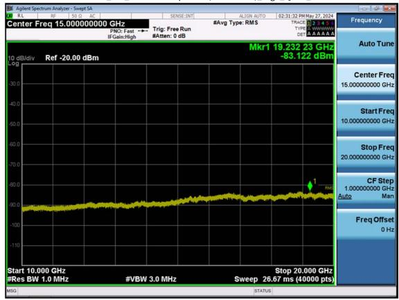
LTE B66\_3 M\_Conducted Spurious(10 G-26.5 G)\_High\_QPSK\_1RB
