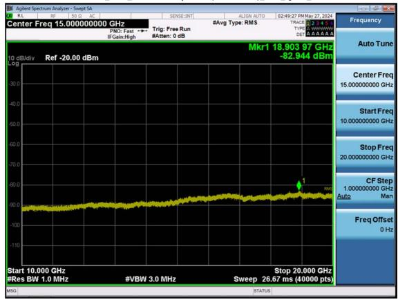
LTE B66\_15 M\_Conducted Spurious(10 G-26.5 G)\_Low\_QPSK\_1RB
