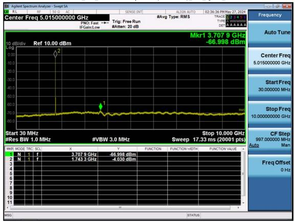
LTE B66\_5 M\_Conducted Spurious(30 M-10 G)\_Mid\_QPSK\_1RB
