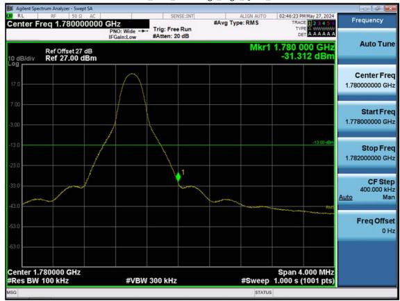
LTE B66\_10 M\_Band Edge\_High\_QPSK\_1RB
