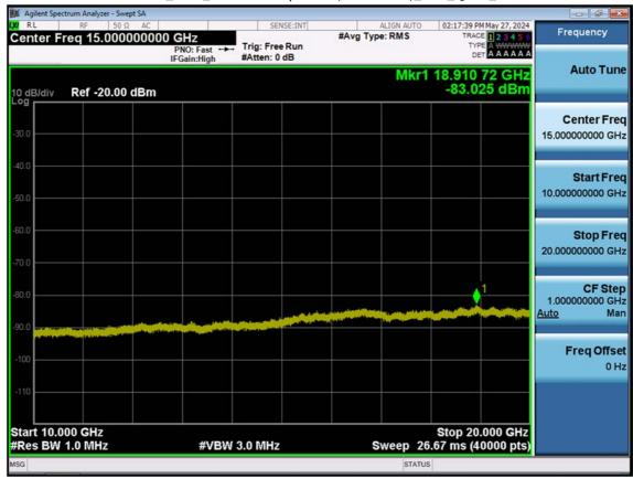
LTE B66\_1.4M\_Conducted Spurious(10 G-26.5 G)\_Low\_QPSK\_1RB
