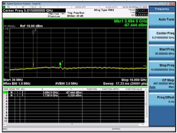
LTE B66\_15 M\_Conducted Spurious(30 M-10 G)\_Mid\_QPSK\_1RB
