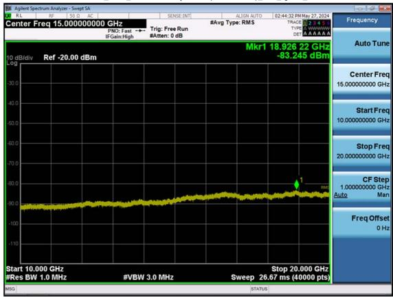
LTE B66\_10 M\_Conducted Spurious(10 G-26.5 G)\_Mid\_QPSK\_1RB
