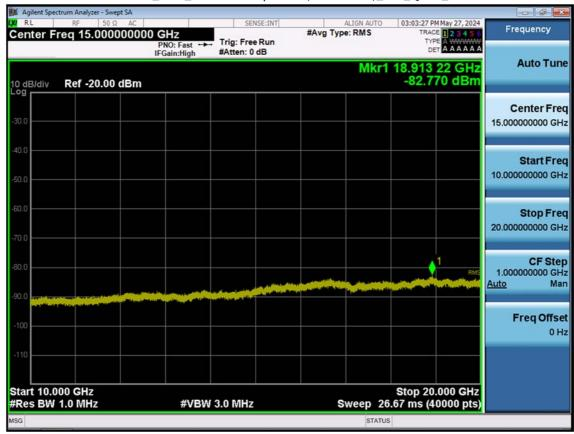
LTE B66\_20 M\_Conducted Spurious(10 G-26.5 G)\_Mid\_QPSK\_1RB
