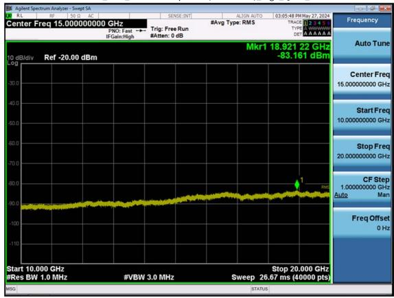
LTE B66\_20 M\_Conducted Spurious(10 G-26.5 G)\_High\_QPSK\_1RB
