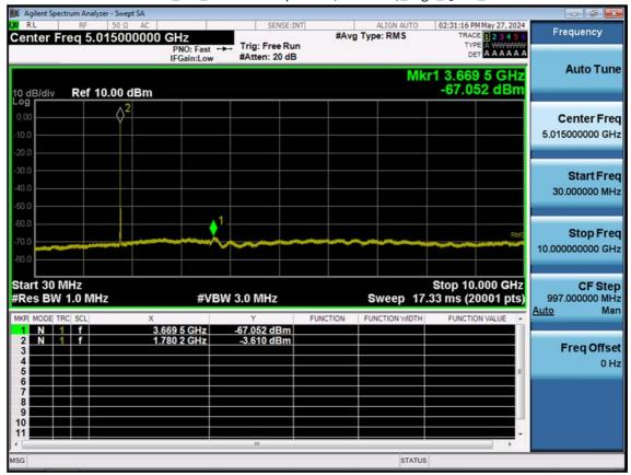
LTE B66\_3 M\_Conducted Spurious(30 M-10 G)\_High\_QPSK\_1RB
