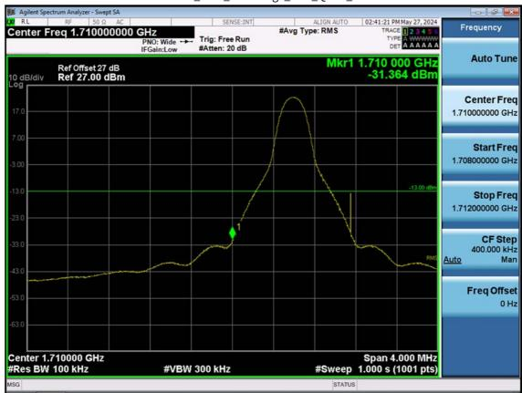
LTE B66\_10 M\_Band Edge\_Low\_QPSK\_1RB
