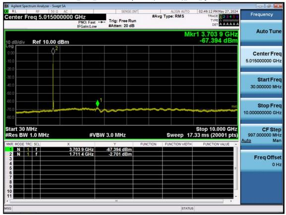
LTE B66\_15 M\_Conducted Spurious(30 M-10 G)\_Low\_QPSK\_1RB
