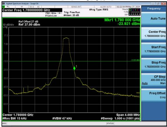
LTE B66\_1.4M\_Band Edge\_High\_QPSK\_1RB
