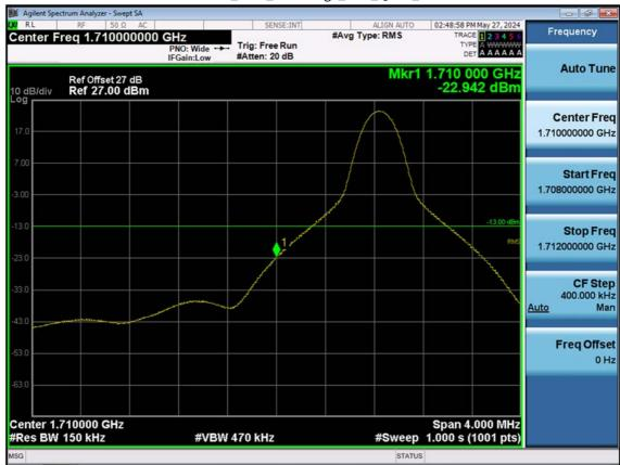
LTE B66\_15 M\_Band Edge\_Low\_QPSK\_1RB
