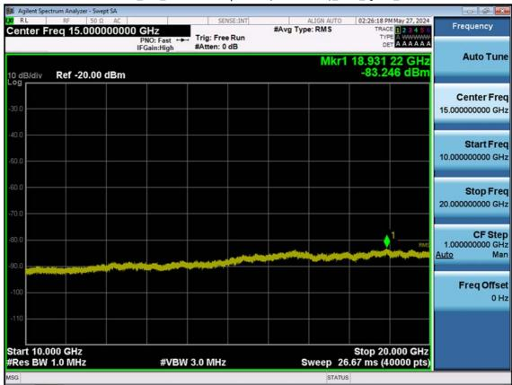
LTE B66\_3 M\_Conducted Spurious(10 G-26.5 G)\_Low\_QPSK\_1RB
