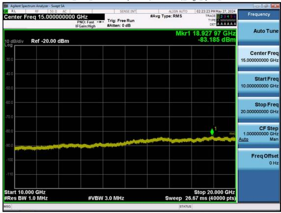
LTE B66\_1.4M\_Conducted Spurious(10 G-26.5 G)\_High\_QPSK\_1RB
