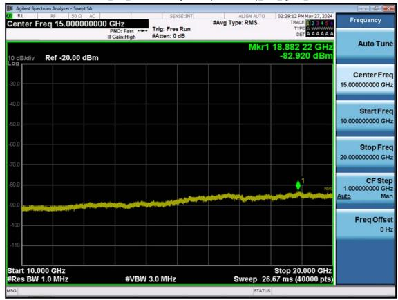
LTE B66\_3 M\_Conducted Spurious(10 G-26.5 G)\_Mid\_QPSK\_1RB
