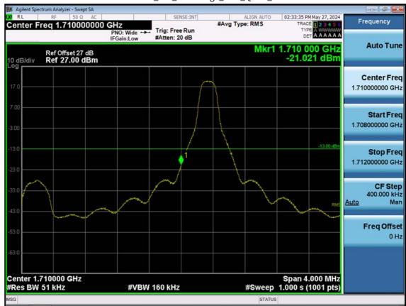
LTE B66\_5 M\_Band Edge\_Low\_QPSK\_1RB
