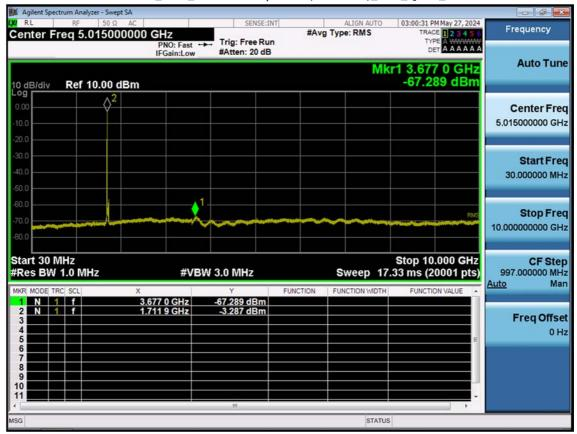
LTE B66\_20 M\_Conducted Spurious(30 M-10 G)\_Low\_QPSK\_1RB
