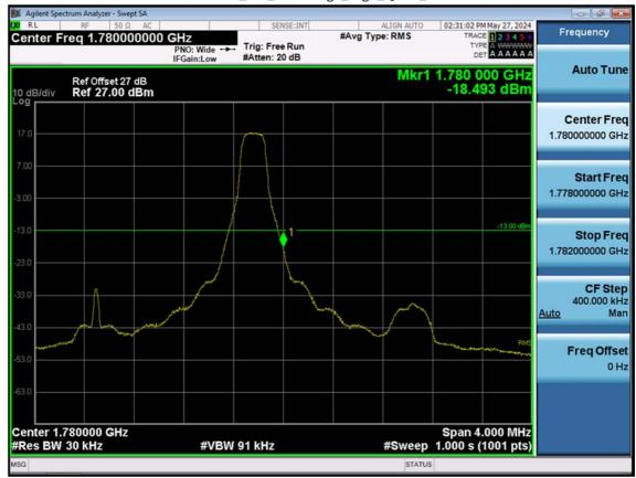
LTE B66\_3 M\_Band Edge\_High\_QPSK\_1RB
