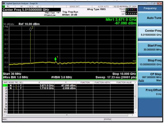
LTE B66\_5 M\_Conducted Spurious(30 M-10 G)\_Low\_QPSK\_1RB
