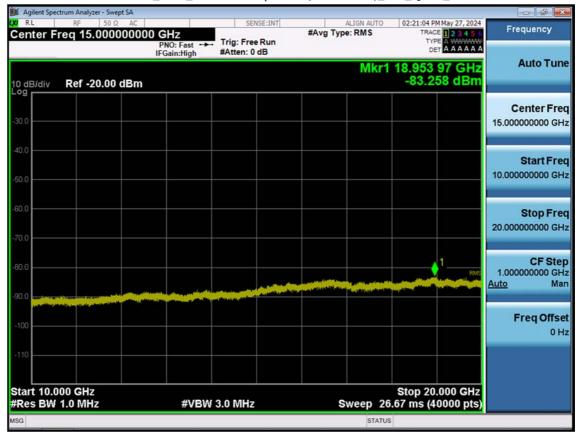
LTE B66\_1.4M\_Conducted Spurious(10 G-26.5 G)\_Mid\_QPSK\_1RB
