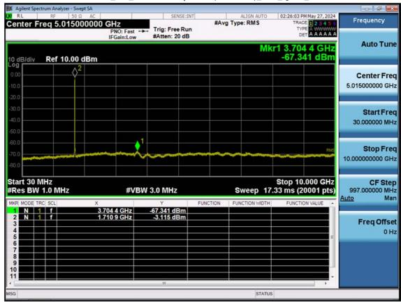
LTE B66\_3 M\_Conducted Spurious(30 M-10 G)\_Low\_QPSK\_1RB
