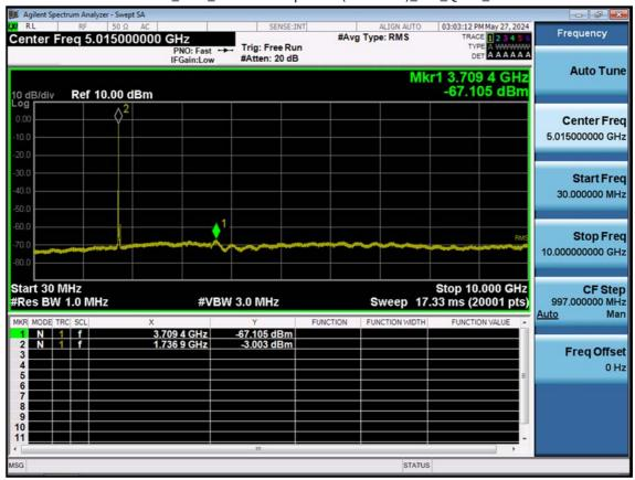
LTE B66\_20 M\_Conducted Spurious(30 M-10 G)\_Mid\_QPSK\_1RB
