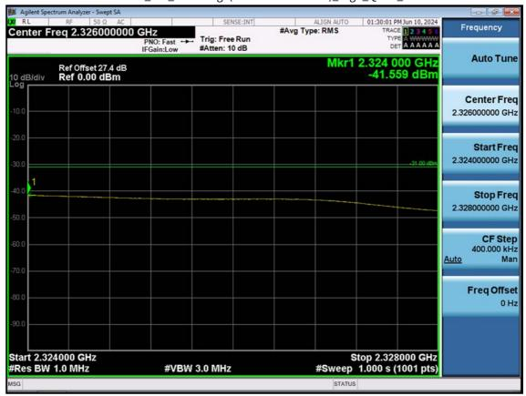
LTE B30\_5 M\_Band Edge(2324MHz-2328MHz)\_High\_QPSK\_1RB
