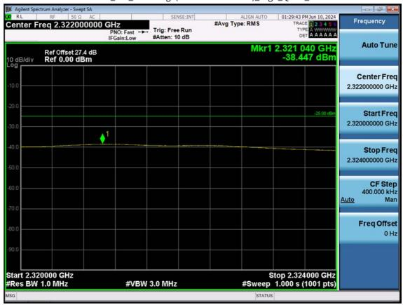
LTE B30\_5 M\_Band Edge(2320MHz-2324MHz)\_High\_QPSK\_1RB
