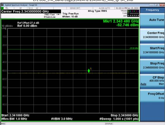
LTE B30\_5 M\_Band Edge(2341MHz-2345MHz)\_Mid\_QPSK\_1RB
