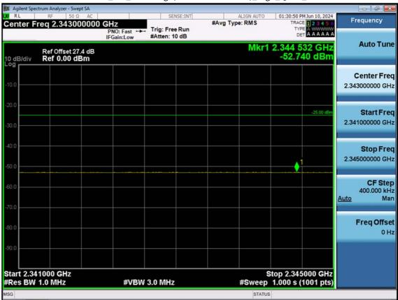
LTE B30\_5 M\_Band Edge(2341MHz-2345MHz)\_High\_QPSK\_1RB
