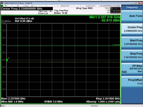
LTE B30\_10 M\_Band Edge(2337MHz-2341MHz)\_Low\_QPSK\_FullRB
