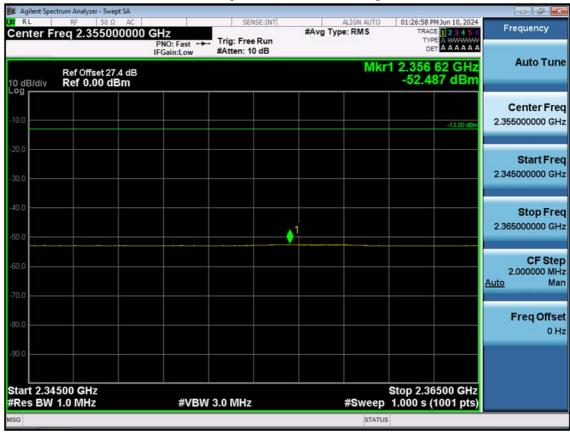
LTE B30\_5 M\_Band Edge(2345MHz-2365MHz)\_High\_QPSK\_FullRB
