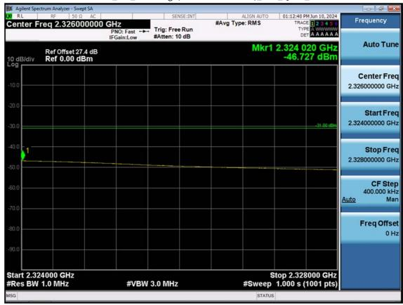
LTE B30\_5 M\_Band Edge(2324MHz-2328MHz)\_Low\_QPSK\_1RB
