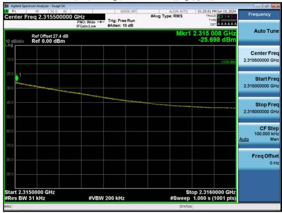
LTE B30\_5 M\_Band Edge(2315MHz-2316MHz)\_High\_QPSK\_FullRB
