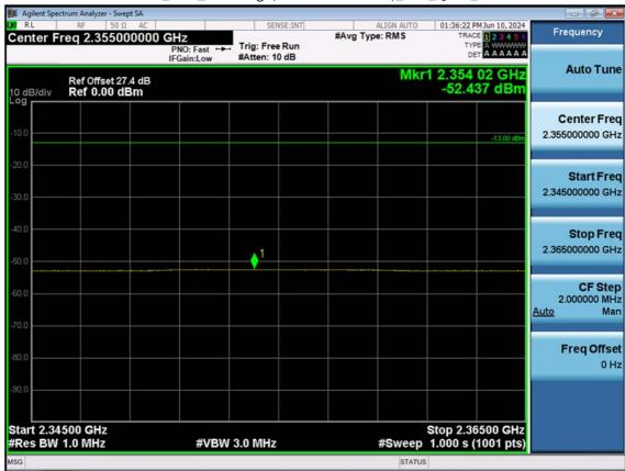
LTE B30\_10 M\_Band Edge(2345MHz-2365MHz)\_Low\_QPSK\_FullRB
