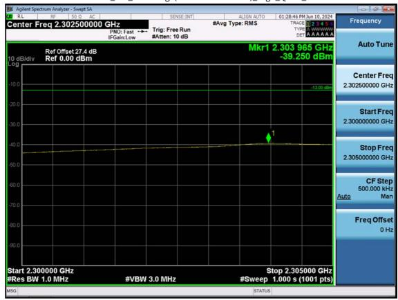
LTE B30\_5 M\_Band Edge(2300MHz-2305MHz)\_High\_QPSK\_1RB
