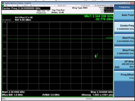
LTE B30\_10 M\_Band Edge(2341MHz-2345MHz)\_Low\_QPSK\_FullRB
