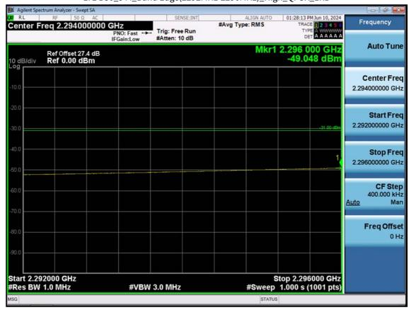
LTE B30\_5 M\_Band Edge(2292MHz-2296MHz)\_High\_QPSK\_1RB
