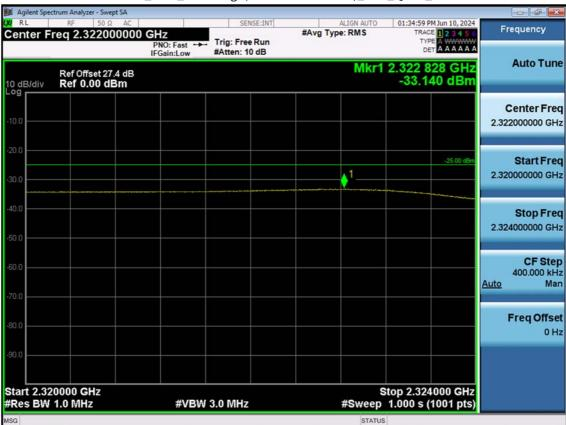
LTE B30\_10 M\_Band Edge(2320MHz-2324MHz)\_Low\_QPSK\_FullRB
