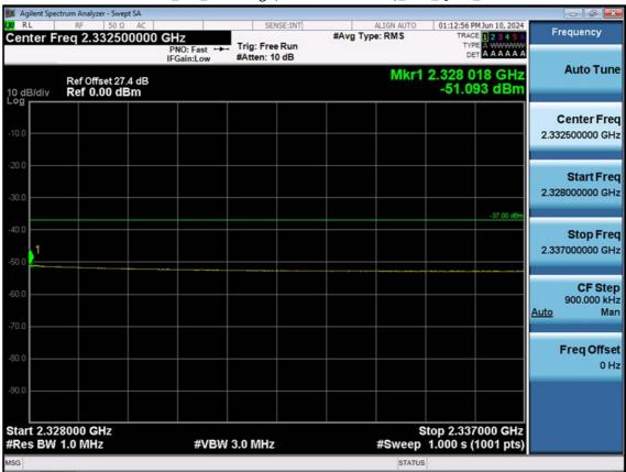
LTE B30\_5 M\_Band Edge(2328MHz-2337MHz)\_Low\_QPSK\_1RB
