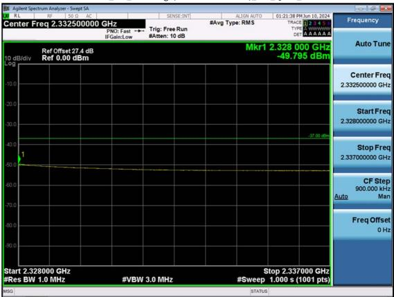
LTE B30\_5 M\_Band Edge(2328MHz-2337MHz)\_Mid\_QPSK\_1RB
