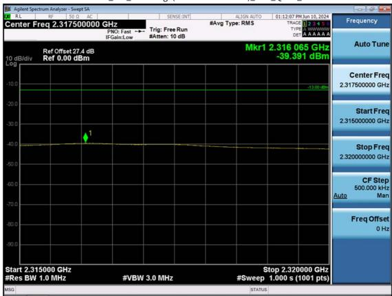
LTE B30\_5 M\_Band Edge(2315MHz-2320MHz)\_Low\_QPSK\_1RB
