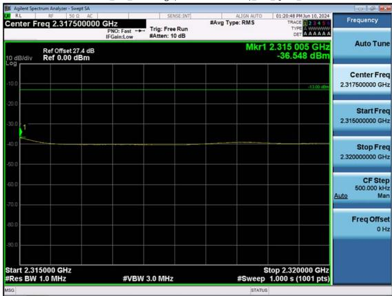
LTE B30\_5 M\_Band Edge(2315MHz-2320MHz)\_Mid\_QPSK\_1RB
