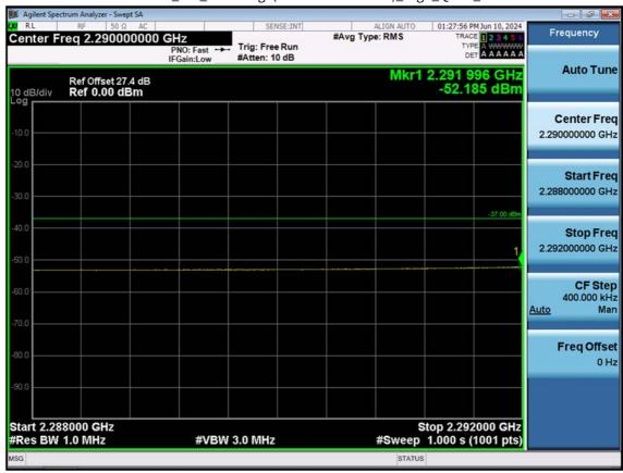
LTE B30\_5 M\_Band Edge(2288MHz-2292MHz)\_High\_QPSK\_1RB
