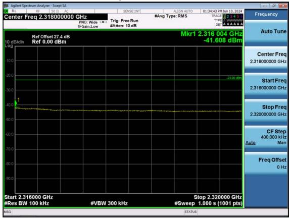
LTE B30\_10 M\_Band Edge(2316MHz-2320MHz)\_Low\_QPSK\_FullRB
