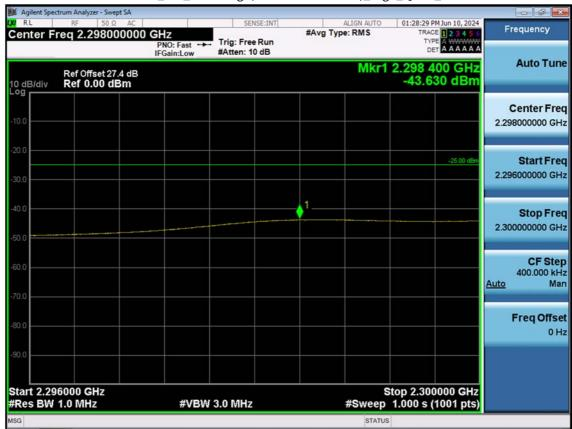
LTE B30\_5 M\_Band Edge(2296MHz-2300MHz)\_High\_QPSK\_1RB
