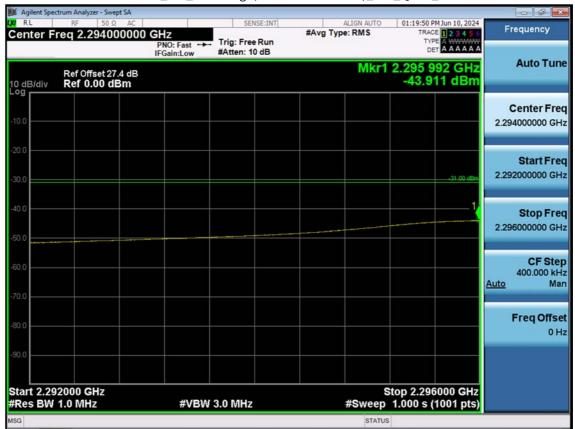
LTE B30\_5 M\_Band Edge(2292MHz-2296MHz)\_Mid\_QPSK\_1RB
