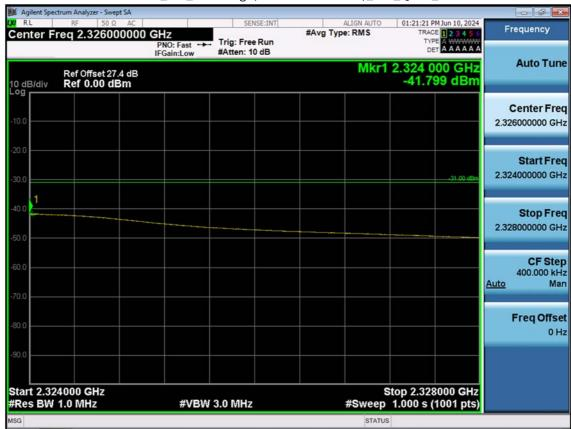
LTE B30\_5 M\_Band Edge(2324MHz-2328MHz)\_Mid\_QPSK\_1RB
