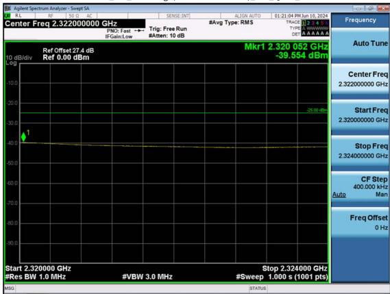
LTE B30\_5 M\_Band Edge(2320MHz-2324MHz)\_Mid\_QPSK\_1RB
