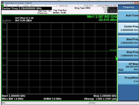
LTE B30\_5 M\_Band Edge(2280MHz-2288MHz)\_Mid\_QPSK\_1RB
