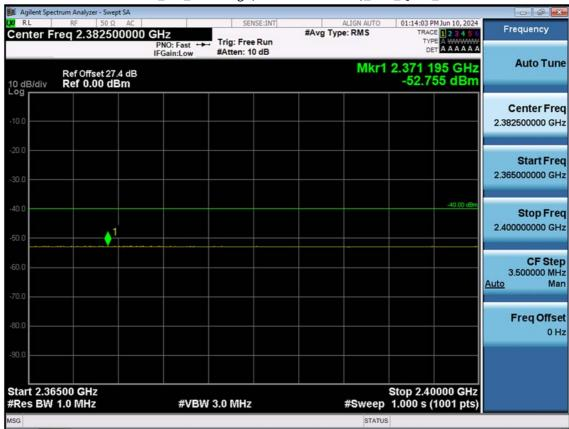
LTE B30\_5 M\_Band Edge(2365MHz-2400MHz)\_Low\_QPSK\_1RB
