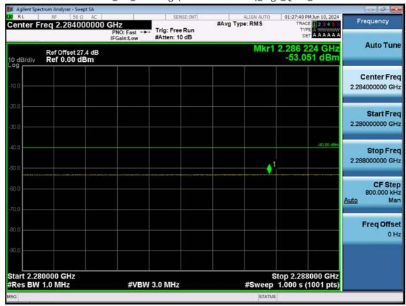
LTE B30\_5 M\_Band Edge(2280MHz-2288MHz)\_High\_QPSK\_1RB
