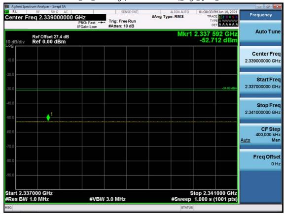
LTE B30\_5 M\_Band Edge(2337MHz-2341MHz)\_High\_QPSK\_1RB
