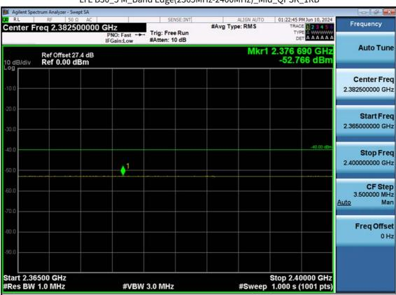
LTE B30\_5 M\_Band Edge(2365MHz-2400MHz)\_Mid\_QPSK\_1RB
