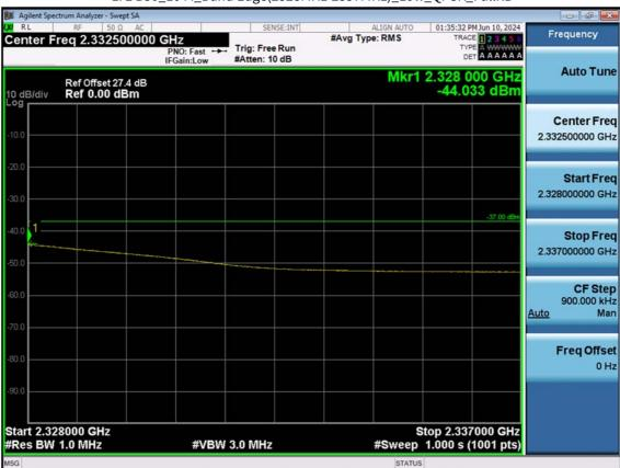
LTE B30\_10 M\_Band Edge(2328MHz-2337MHz)\_Low\_QPSK\_FullRB
