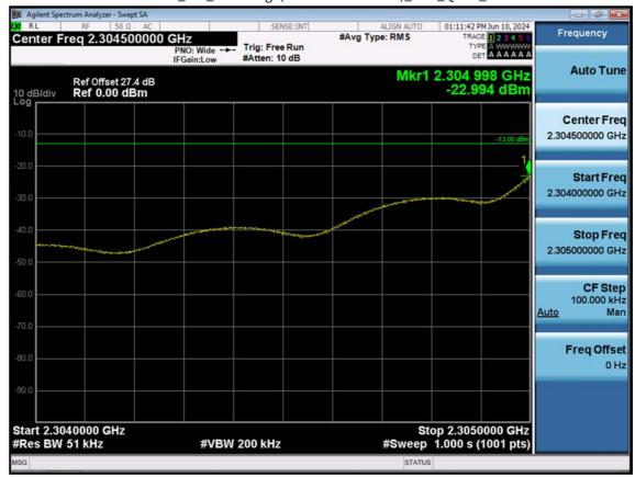
LTE B30\_5 M\_Band Edge(2304MHz-2305MHz)\_Low\_QPSK\_1RB
