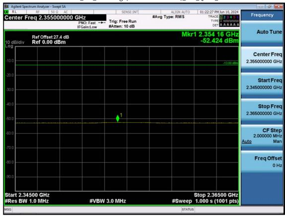
LTE B30\_5 M\_Band Edge(2345MHz-2365MHz)\_Mid\_QPSK\_1RB
