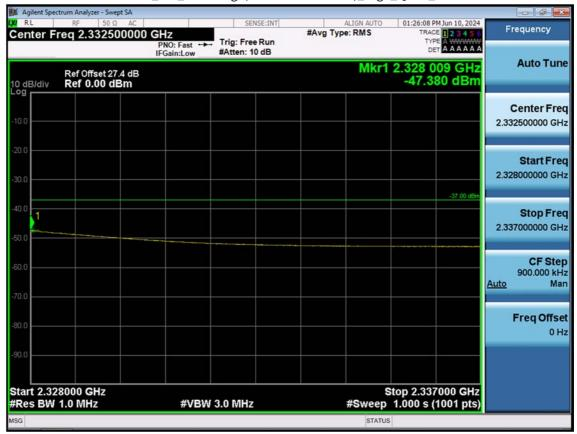
LTE B30\_5 M\_Band Edge(2328MHz-2337MHz)\_High\_QPSK\_FullRB
