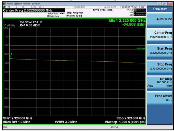
LTE B30\_5 M\_Band Edge(2320MHz-2324MHz)\_High\_QPSK\_FullRB
