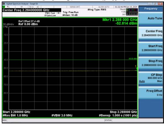
LTE B30\_10 M\_Band Edge(2280MHz-2288MHz)\_Low\_QPSK\_FullRB
