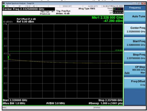
LTE B30\_5 M\_Band Edge(2328MHz-2337MHz)\_High\_QPSK\_1RB
