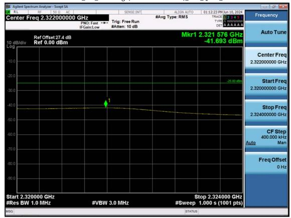
LTE B30\_5 M\_Band Edge(2320MHz-2324MHz)\_Low\_QPSK\_1RB
