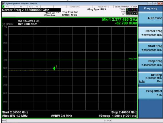
LTE B30\_10 M\_Band Edge(2365MHz-2400MHz)\_Low\_QPSK\_FullRB
