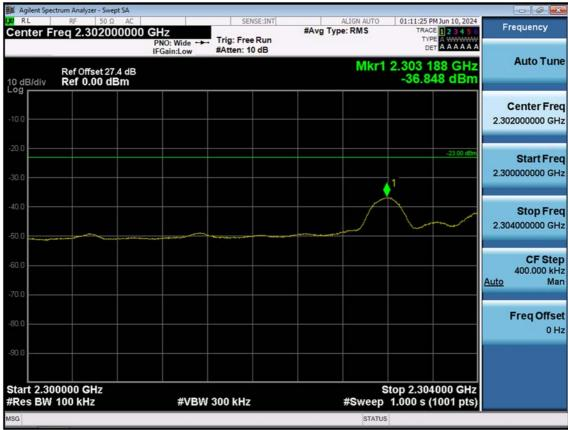
LTE B30\_5 M\_Band Edge(2300MHz-2304MHz)\_Low\_QPSK\_1RB
