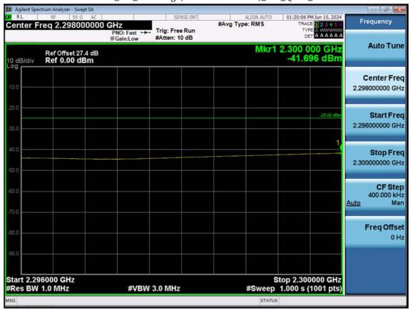
LTE B30\_5 M\_Band Edge(2296MHz-2300MHz)\_Mid\_QPSK\_1RB
