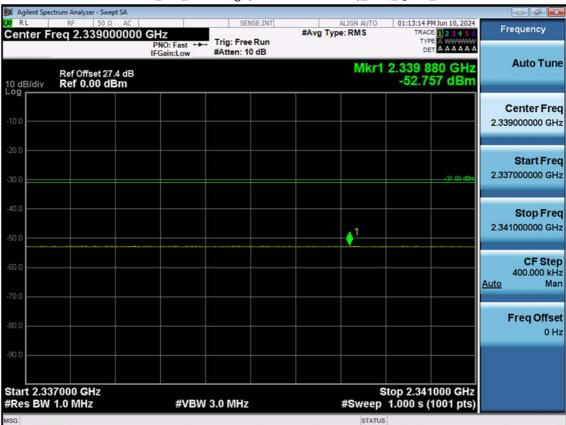
LTE B30\_5 M\_Band Edge(2337MHz-2341MHz)\_Low\_QPSK\_1RB
