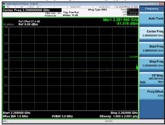
LTE B30\_5 M\_Band Edge(2288MHz-2292MHz)\_Mid\_QPSK\_1RB
