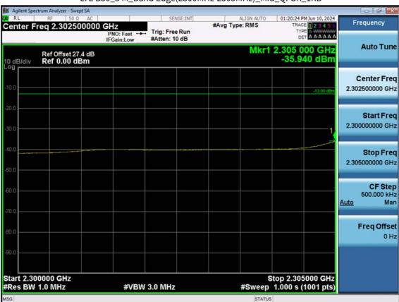
LTE B30\_5 M\_Band Edge(2300MHz-2305MHz)\_Mid\_QPSK\_1RB
