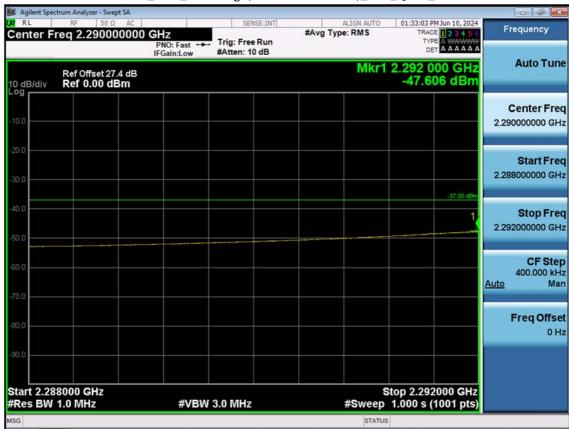
LTE B30\_10 M\_Band Edge(2288MHz-2292MHz)\_Low\_QPSK\_FullRB
