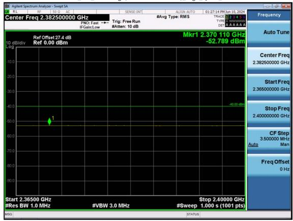
LTE B30\_5 M\_Band Edge(2365MHz-2400MHz)\_High\_QPSK\_FullRB
