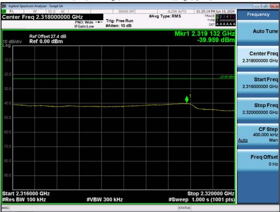
LTE B30\_5 M\_Band Edge(2316MHz-2320MHz)\_High\_QPSK\_FullRB
