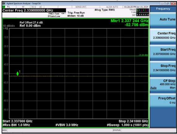
LTE B30\_5 M\_Band Edge(2337MHz-2341MHz)\_High\_QPSK\_FullRB
