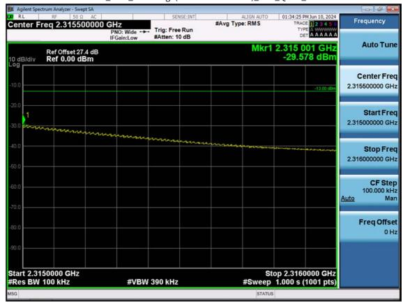
LTE B30\_10 M\_Band Edge(2315MHz-2316MHz)\_Low\_QPSK\_FullRB
