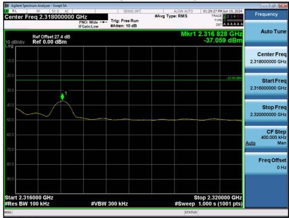
LTE B30\_5 M\_Band Edge(2316MHz-2320MHz)\_High\_QPSK\_1RB
