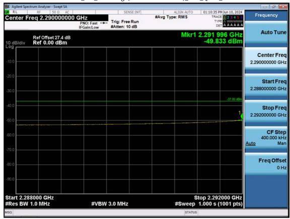
LTE B30\_5 M\_Band Edge(2288MHz-2292MHz)\_Low\_QPSK\_1RB
