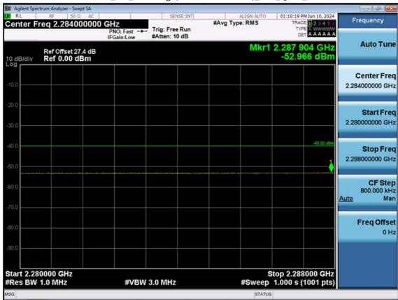
LTE B30\_5 M\_Band Edge(2280MHz-2288MHz)\_Low\_QPSK\_1RB
