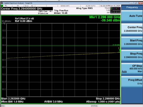
LTE B30\_10 M\_Band Edge(2292MHz-2296MHz)\_Low\_QPSK\_FullRB
