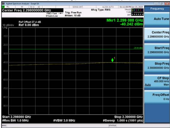
LTE B30\_5 M\_Band Edge(2296MHz-2300MHz)\_Low\_QPSK\_1RB
