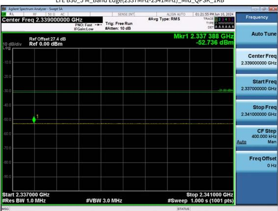
LTE B30\_5 M\_Band Edge(2337MHz-2341MHz)\_Mid\_QPSK\_1RB
