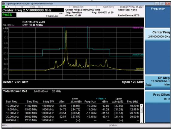
LTE B7\_20 M\_Channel Edge\_Low\_QPSK\_1RB
