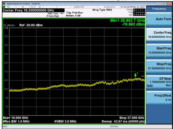
LTE B7\_15 M\_Conducted Spurious(10 G-26.5 G)\_High\_QPSK\_1RB
