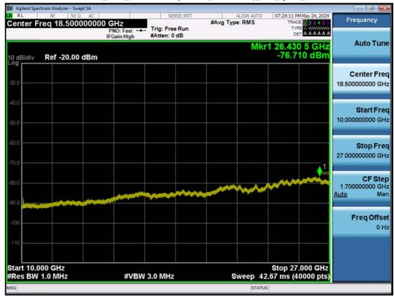
LTE B7\_15 M\_Conducted Spurious(10 G-26.5 G)\_Mid\_QPSK\_1RB
