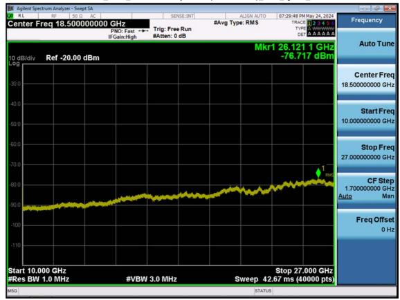
LTE B7\_20 M\_Conducted Spurious(10 G-26.5 G)\_Low\_QPSK\_1RB
