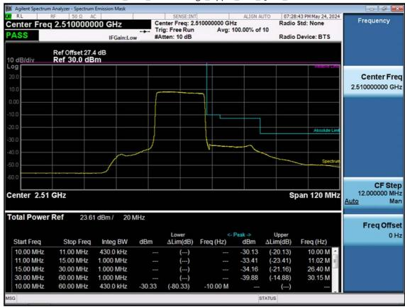
LTE B7\_20 M\_Channel Edge\_Upper\_Low\_QPSK\_FullRB
