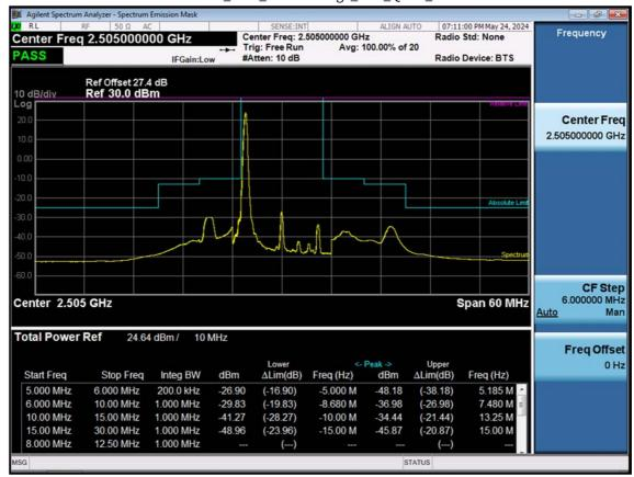
LTE B7\_10 M\_Channel Edge\_Low\_QPSK\_1RB
