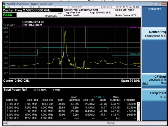
LTE B7\_5 M\_Channel Edge\_Low\_QPSK\_1RB
