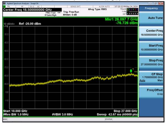
LTE B7\_20 M\_Conducted Spurious(10 G-26.5 G)\_High\_QPSK\_1RB
