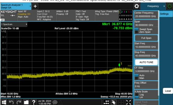
n77(3700~3980 MHz)\_20 M\_Conducted Spurious(Above10 G)\_Low\_BPSK\_1RB
