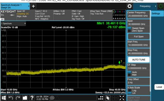
n77(3700~3980 MHz)\_40 M\_Conducted Spurious(Above10 G)\_Low\_BPSK\_1RB
