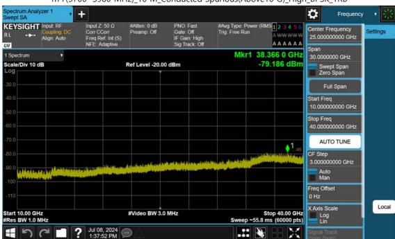
n77(3700~3980 MHz)\_10 M\_Conducted Spurious(Above10 G)\_High\_BPSK\_1RB
