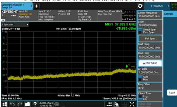
n77(3700~3980 MHz)\_15 M\_Conducted Spurious(Above10 G)\_Mid\_BPSK\_1RB
