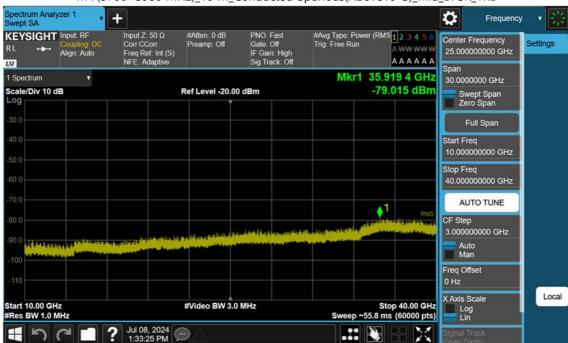
n77(3700~3980 MHz)\_10 M\_Conducted Spurious(Above10 G)\_Mid\_BPSK\_1RB
