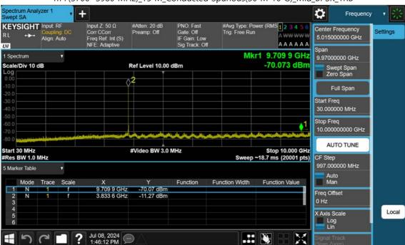
n77(3700~3980 MHz)\_15 M\_Conducted Spurious(30 M-10 G)\_Mid\_BPSK\_1RB
