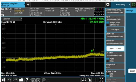
n77(3700~3980 MHz)\_10 M\_Conducted Spurious(Above10 G)\_Low\_BPSK\_1RB
