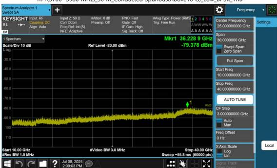
n77(3700~3980 MHz)\_30 M\_Conducted Spurious(Above10 G)\_Low\_BPSK\_1RB
