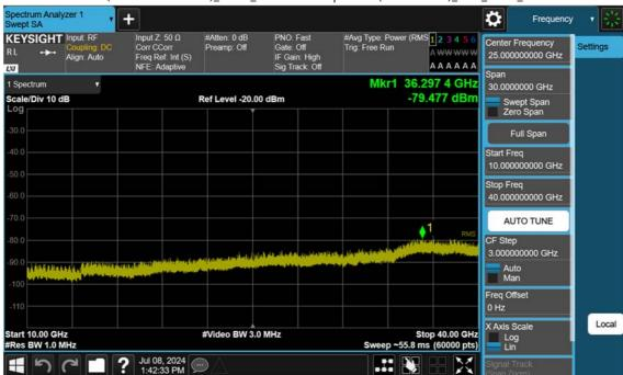
n77(3700~3980 MHz)\_15 M\_Conducted Spurious(Above10 G)\_Low\_BPSK\_1RB
