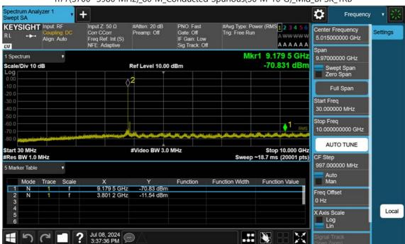
n77(3700~3980 MHz)\_80 M\_Conducted Spurious(30 M-10 G)\_Mid\_BPSK\_1RB
