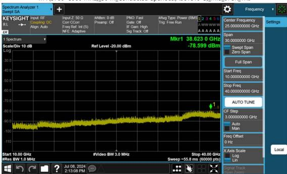
n77(3700~3980 MHz)\_30 M\_Conducted Spurious(Above10 G)\_Mid\_BPSK\_1RB
