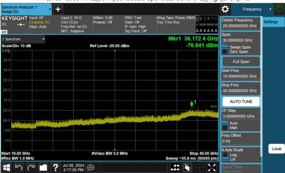
n77(3700~3980 MHz)\_30 M\_Conducted Spurious(Above10 G)\_High\_BPSK\_1RB
