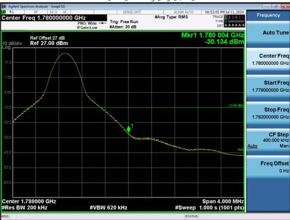
LTE B66\_20 M\_Band Edge\_High\_QPSK\_1RB
