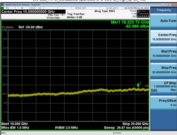
LTE B66\_1.4 M\_Conducted Spurious(10 G-26.5 G)\_High\_QPSK\_1RB
