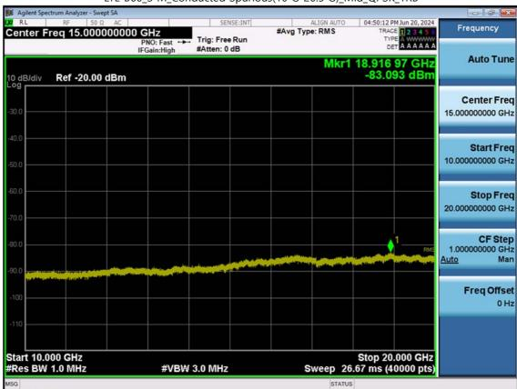
LTE B66\_3 M\_Conducted Spurious(10 G-26.5 G)\_Mid\_QPSK\_1RB
