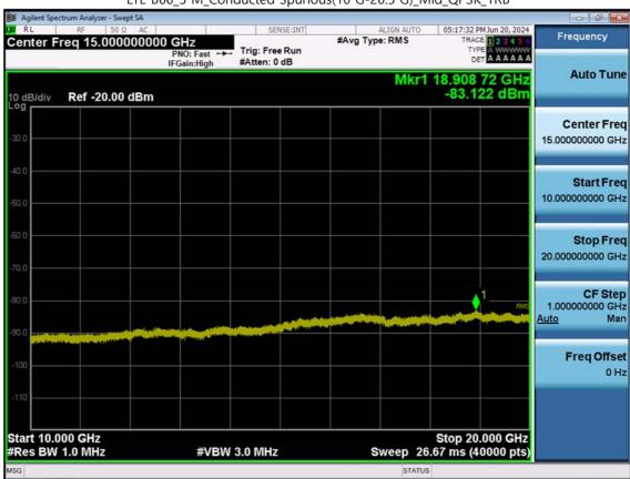
LTE B66\_5 M\_Conducted Spurious(10 G-26.5 G)\_Mid\_QPSK\_1RB
