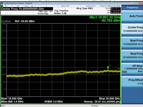
LTE B66\_3 M\_Conducted Spurious(10 G-26.5 G)\_Low\_QPSK\_1RB
