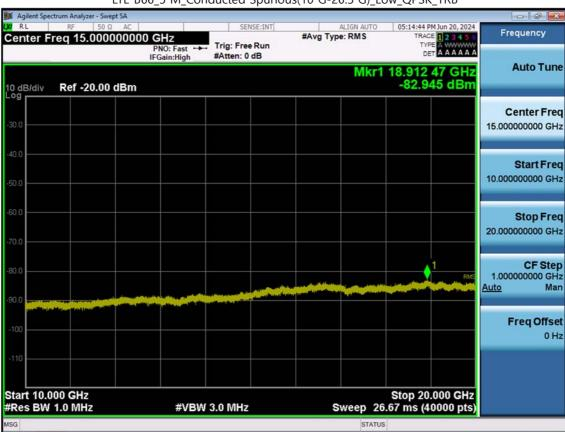
LTE B66\_5 M\_Conducted Spurious(10 G-26.5 G)\_Low\_QPSK\_1RB
