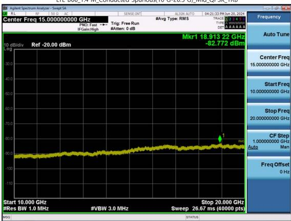
LTE B66\_1.4 M\_Conducted Spurious(10 G-26.5 G)\_Mid\_QPSK\_1RB
