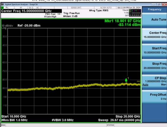
LTE B66\_10 M\_Conducted Spurious(10 G-26.5 G)\_Mid\_QPSK\_1RB
