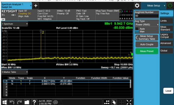
LTE B41\_5 M\_Conducted Spurious(30 M-10 G)\_High\_QPSK\_1RB
