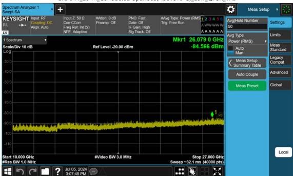
LTE B41\_20 M\_Conducted Spurious(Above10 G)\_Low\_QPSK\_1RB
