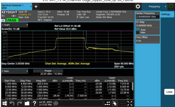
LTE B41\_15 M\_Channel Edge\_Upper\_Low\_QPSK\_FullRB
