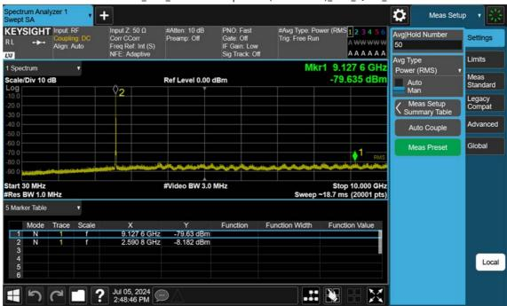
LTE B41\_5 M\_Conducted Spurious(30 M-10 G)\_Mid\_QPSK\_1RB
