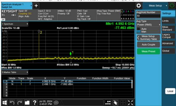
LTE B41\_5 M\_Conducted Spurious(30 M-10 G)\_Low\_QPSK\_1RB
