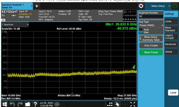
LTE B41\_15 M\_Conducted Spurious(Above10 G)\_Low\_QPSK\_1RB
