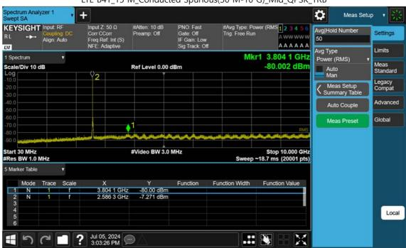
LTE B41\_15 M\_Conducted Spurious(30 M-10 G)\_Mid\_QPSK\_1RB
