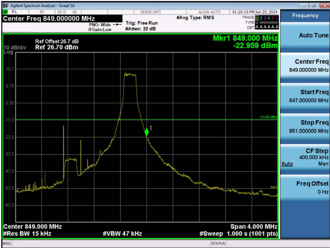
BAND26. Upper Band Edge Plot (1.4 M BW Ch.27033 QPSK_RB1_Offset 5)
