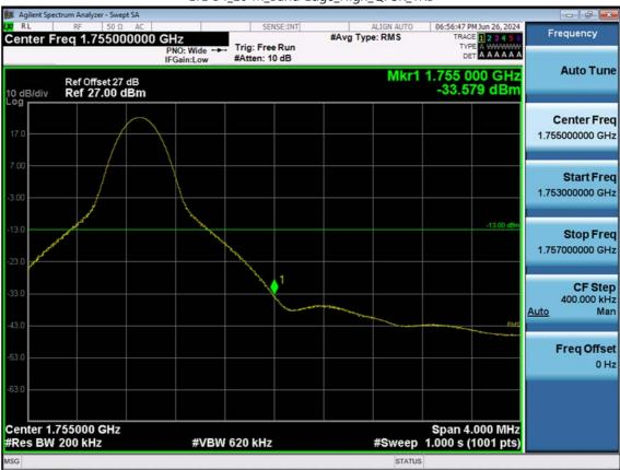
LTE B4\_20 M\_Band Edge\_High\_QPSK\_1RB
