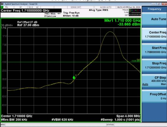
LTE B4\_20 M\_Band Edge\_Low\_QPSK\_1RB
