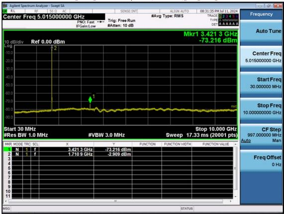
LTE B4\_1.4 M\_Conducted Spurious(30 M-10 G)\_Low\_QPSK\_1RB
