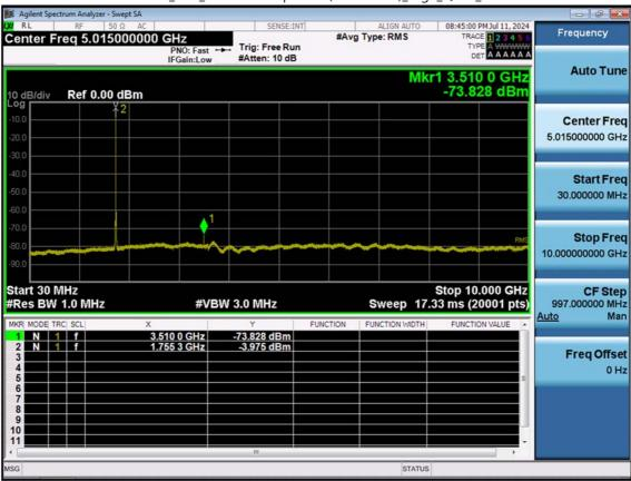
LTE B4\_3 M\_Conducted Spurious(30 M-10 G)\_High\_QPSK\_1RB
