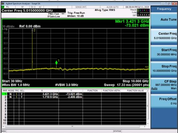
LTE B4\_3 M\_Conducted Spurious(30 M-10 G)\_Low\_QPSK\_1RB
