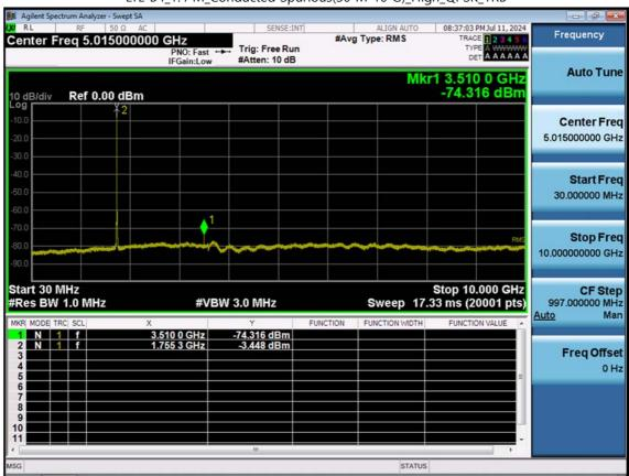
LTE B4\_1.4 M\_Conducted Spurious(30 M-10 G)\_High\_QPSK\_1RB
