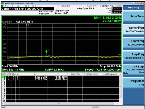
LTE B4\_3 M\_Conducted Spurious(30 M-10 G)\_Mid\_QPSK\_1RB
