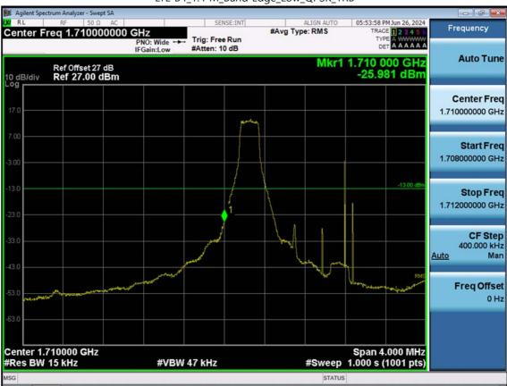
LTE B4\_1.4 M\_Band Edge\_Low\_QPSK\_1RB
