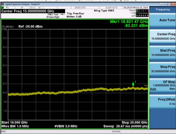
LTE B4\_10 M\_Conducted Spurious(10 G-26.5 G)\_High\_QPSK\_1RB
