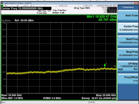
LTE B4\_3 M\_Conducted Spurious(10 G-26.5 G)\_Mid\_QPSK\_1RB
