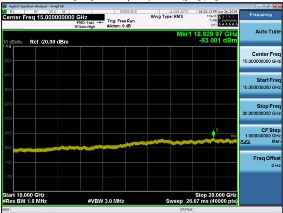
LTE B4\_20 M\_Conducted Spurious(10 G-26.5 G)\_Low\_QPSK\_1RB
