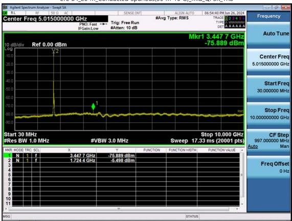
LTE B4\_20 M\_Conducted Spurious(30 M-10 G)\_Mid\_QPSK\_1RB
