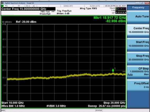
LTE B4\_1.4 M\_Conducted Spurious(10 G-26.5 G)\_Low\_QPSK\_1RB
