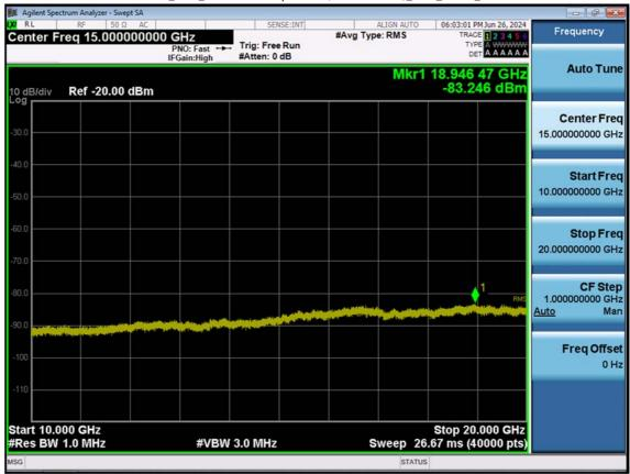
LTE B4\_3 M\_Conducted Spurious(10 G-26.5 G)\_Low\_QPSK\_1RB
