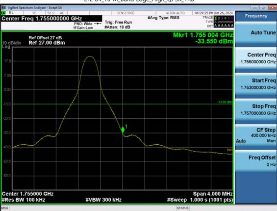
LTE B4\_10 M\_Band Edge\_High\_QPSK\_1RB
