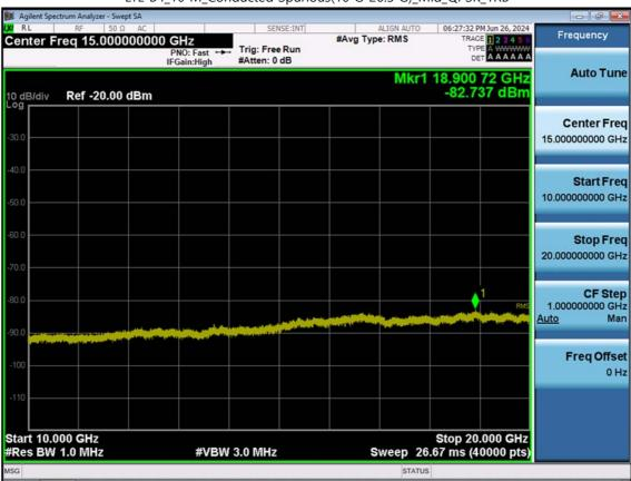
LTE B4\_10 M\_Conducted Spurious(10 G-26.5 G)\_Mid\_QPSK\_1RB
