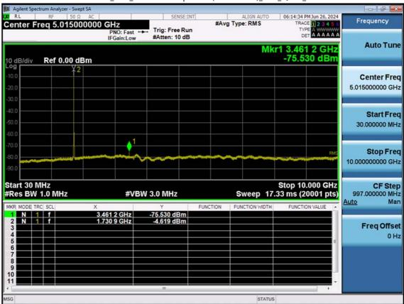
LTE B4\_5 M\_Conducted Spurious(30 M-10 G)\_Mid\_QPSK\_1RB
