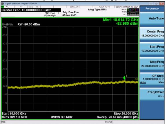
LTE B4\_5 M\_Conducted Spurious(10 G-26.5 G)\_High\_QPSK\_1RB
