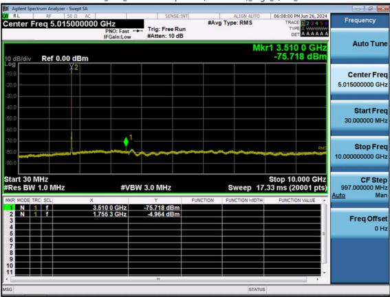
LTE B4\_3 M\_Conducted Spurious(30 M-10 G)\_High\_QPSK\_1RB
