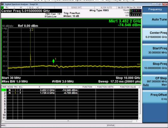
LTE B4\_15 M\_Conducted Spurious(30 M-10 G)\_Mid\_QPSK\_1RB
