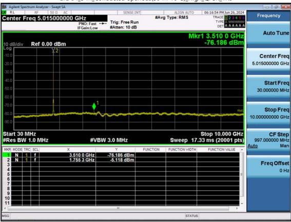
LTE B4\_5 M\_Conducted Spurious(30 M-10 G)\_High\_QPSK\_1RB
