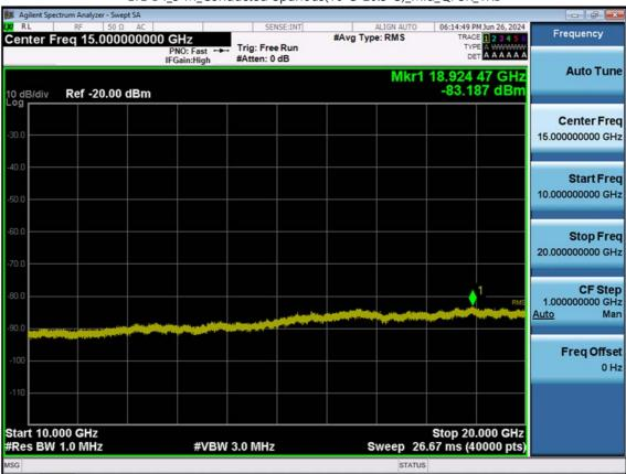
LTE B4\_5 M\_Conducted Spurious(10 G-26.5 G)\_Mid\_QPSK\_1RB
