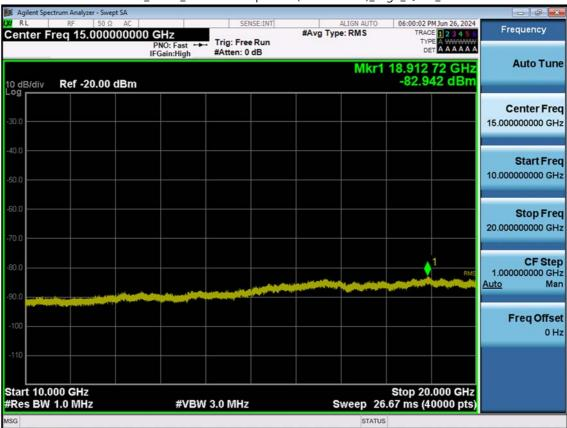
LTE B4\_1.4 M\_Conducted Spurious(10 G-26.5 G)\_High\_QPSK\_1RB
