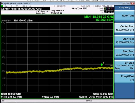
LTE B4\_20 M\_Conducted Spurious(10 G-26.5 G)\_Mid\_QPSK\_1RB
