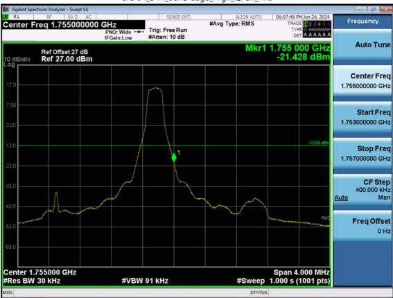
LTE B4\_3 M\_Band Edge\_High\_QPSK\_1RB
