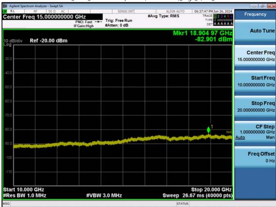
LTE B4\_15 M\_Conducted Spurious(10 G-26.5 G)\_High\_QPSK\_1RB
