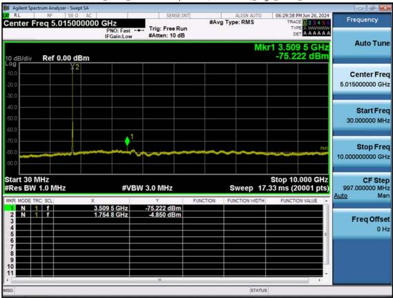
LTE B4\_10 M\_Conducted Spurious(30 M-10 G)\_High\_QPSK\_1RB
