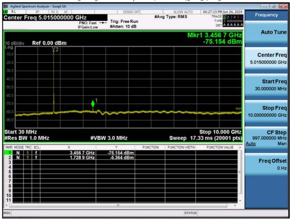
LTE B4\_10 M\_Conducted Spurious(30 M-10 G)\_Mid\_QPSK\_1RB
