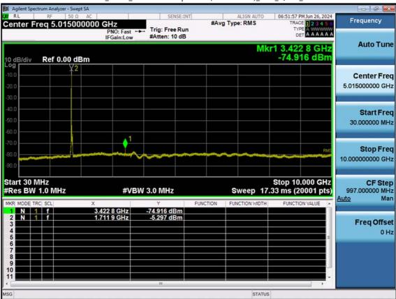
LTE B4\_20 M\_Conducted Spurious(30 M-10 G)\_Low\_QPSK\_1RB
