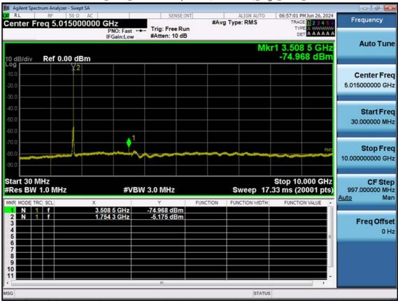
LTE B4\_20 M\_Conducted Spurious(30 M-10 G)\_High\_QPSK\_1RB
