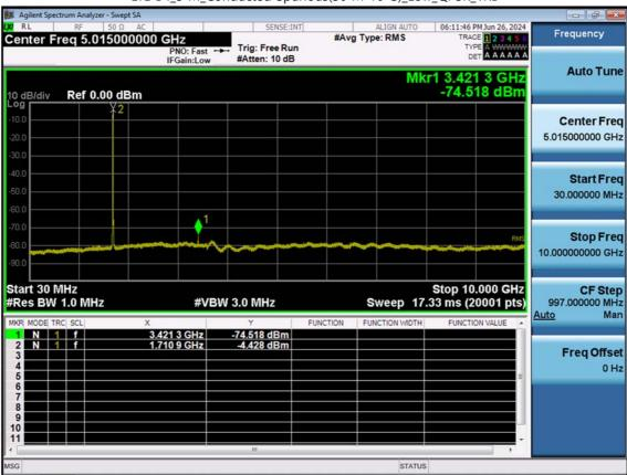
LTE B4\_5 M\_Conducted Spurious(30 M-10 G)\_Low\_QPSK\_1RB
