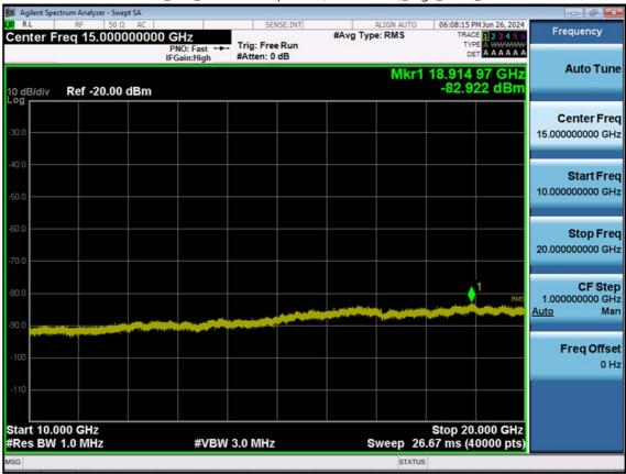
LTE B4\_3 M\_Conducted Spurious(10 G-26.5 G)\_High\_QPSK\_1RB
