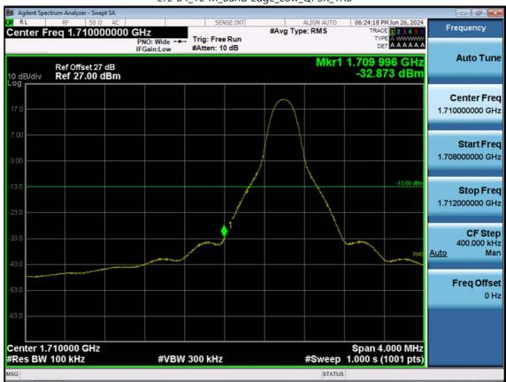
LTE B4\_10 M\_Band Edge\_Low\_QPSK\_1RB
