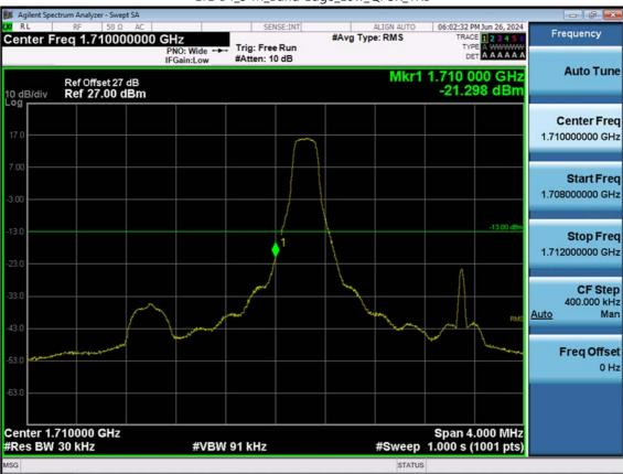
LTE B4\_3 M\_Band Edge\_Low\_QPSK\_1RB
