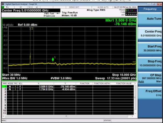
LTE B4\_15 M\_Conducted Spurious(30 M-10 G)\_High\_QPSK\_1RB
