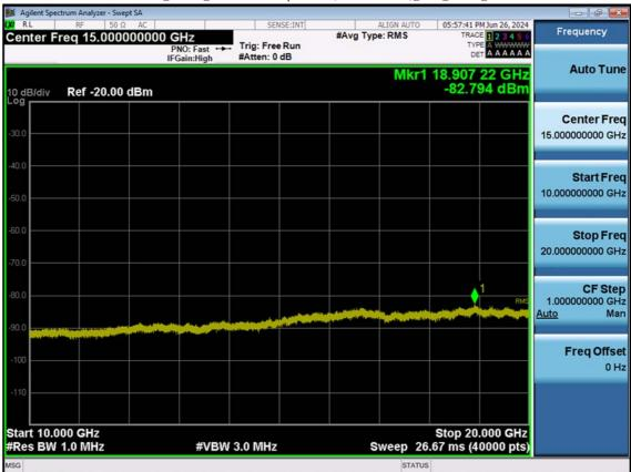
LTE B4\_1.4 M\_Conducted Spurious(10 G-26.5 G)\_Mid\_QPSK\_1RB
