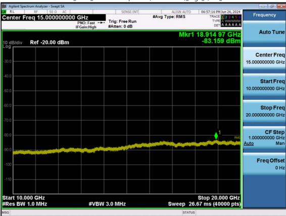
LTE B4\_20 M\_Conducted Spurious(10 G-26.5 G)\_High\_QPSK\_1RB
