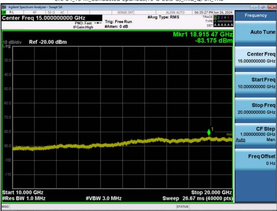
LTE B4\_15 M\_Conducted Spurious(10 G-26.5 G)\_Mid\_QPSK\_1RB
