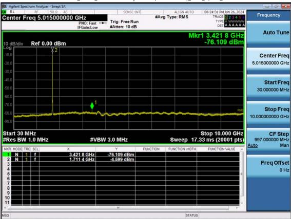
LTE B4\_10 M\_Conducted Spurious(30 M-10 G)\_Low\_QPSK\_1RB
