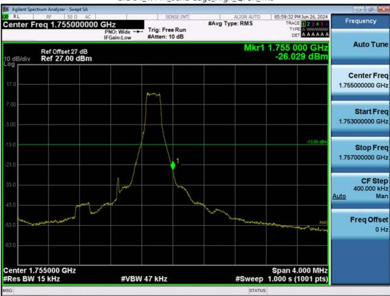
LTE B4\_1.4 M\_Band Edge\_High\_QPSK\_1RB
