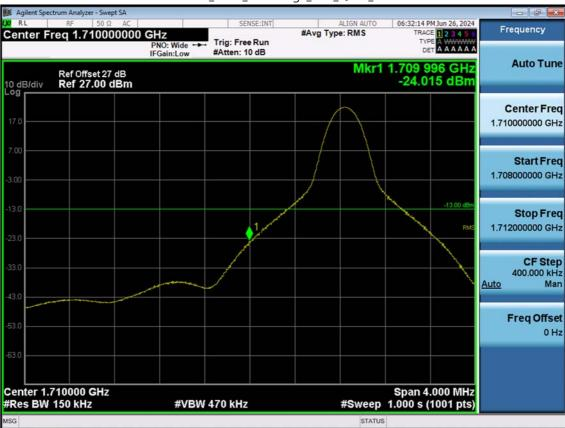
LTE B4\_15 M\_Band Edge\_Low\_QPSK\_1RB
