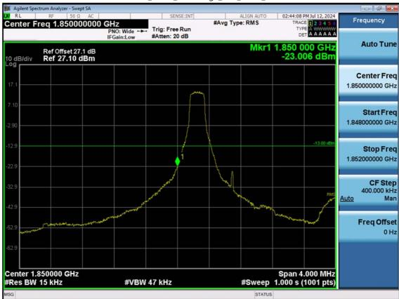
LTE B2\_1.4 M\_Band Edge\_Low\_QPSK\_1RB
