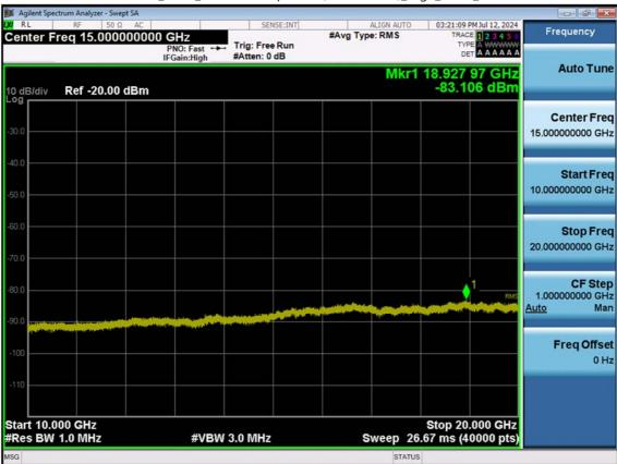
LTE B2\_10 M\_Conducted Spurious(10 G-26.5 G)\_High\_QPSK\_1RB
