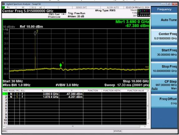
LTE B2\_5 M\_Conducted Spurious(30 M-10 G)\_Mid\_QPSK\_1RB
