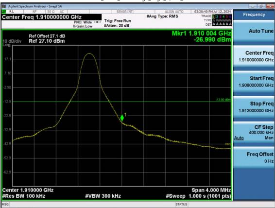
LTE B2\_10 M\_Band Edge\_High\_QPSK\_1RB
