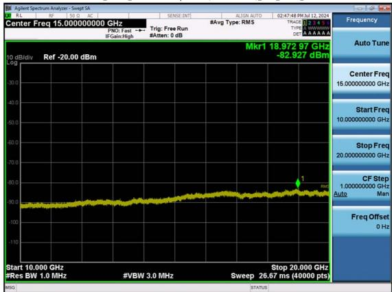
LTE B2\_1.4 M\_Conducted Spurious(10 G-26.5 G)\_Mid\_QPSK\_1RB
