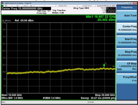
LTE B2\_15 M\_Conducted Spurious(10 G-26.5 G)\_High\_QPSK\_1RB
