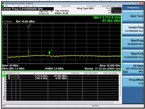
LTE B2\_10 M\_Conducted Spurious(30 M-10 G)\_Low\_QPSK\_1RB
