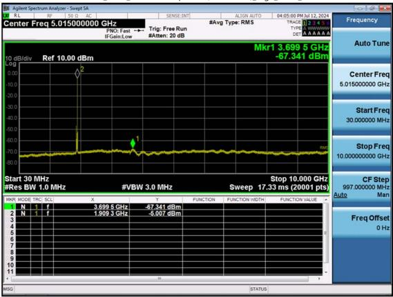
LTE B2\_20 M\_Conducted Spurious(30 M-10 G)\_High\_QPSK\_1RB
