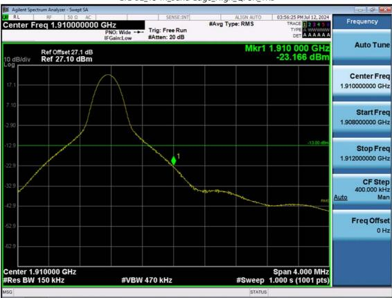
LTE B2\_15 M\_Band Edge\_High\_QPSK\_1RB
