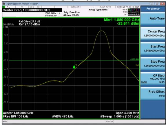
LTE B2\_15 M\_Band Edge\_Low\_QPSK\_1RB
