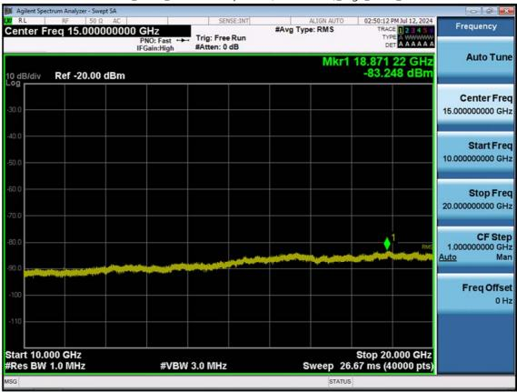
LTE B2\_1.4 M\_Conducted Spurious(10 G-26.5 G)\_High\_QPSK\_1RB
