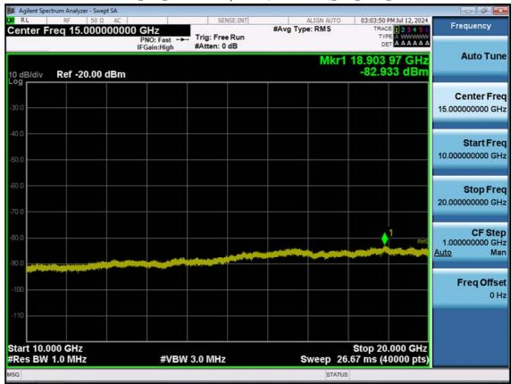
LTE B2\_5 M\_Conducted Spurious(10 G-26.5 G)\_Mid\_QPSK\_1RB
