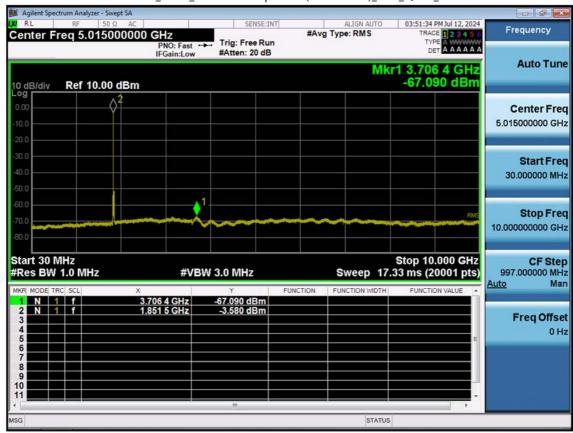
LTE B2\_15 M\_Conducted Spurious(30 M-10 G)\_Low\_QPSK\_1RB
