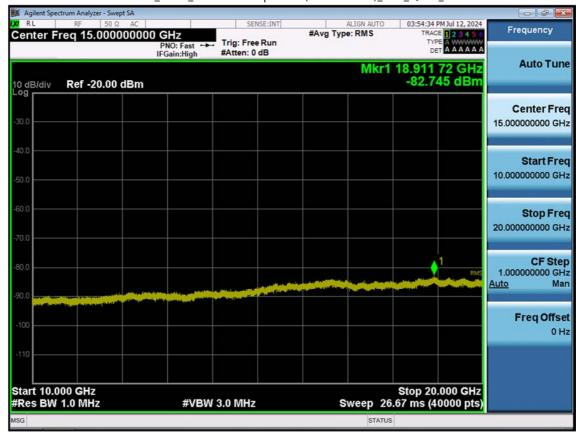
LTE B2\_15 M\_Conducted Spurious(10 G-26.5 G)\_Mid\_QPSK\_1RB
