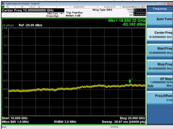
LTE B2\_10 M\_Conducted Spurious(10 G-26.5 G)\_Low\_QPSK\_1RB
