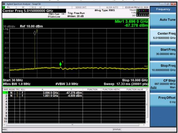
LTE B2\_5 M\_Conducted Spurious(30 M-10 G)\_Low\_QPSK\_1RB
