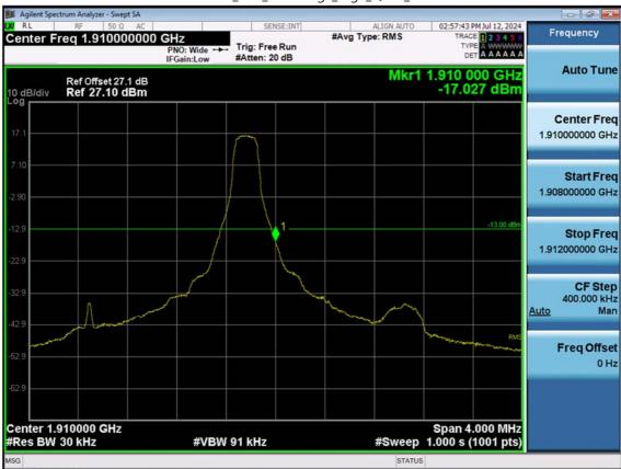
LTE B2\_3 M\_Band Edge\_High\_QPSK\_1RB
