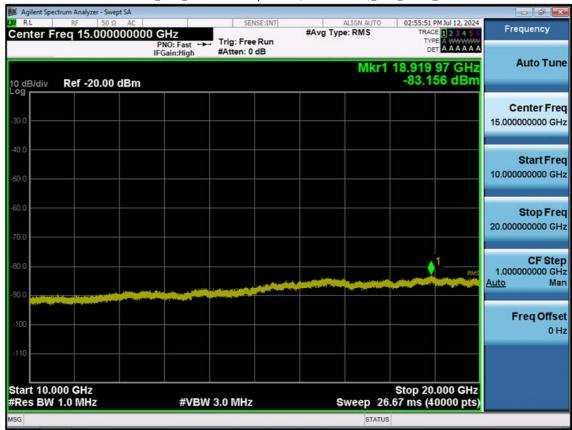
LTE B2\_3 M\_Conducted Spurious(10 G-26.5 G)\_Mid\_QPSK\_1RB
