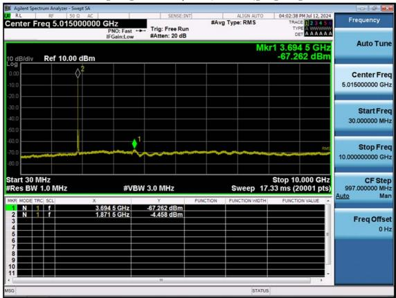
LTE B2\_20 M\_Conducted Spurious(30 M-10 G)\_Mid\_QPSK\_1RB
