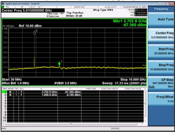
LTE B2\_10 M\_Conducted Spurious(30 M-10 G)\_High\_QPSK\_1RB
