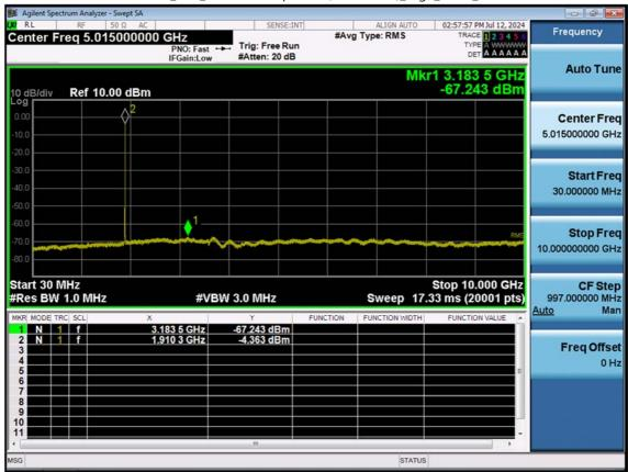
LTE B2\_3 M\_Conducted Spurious(30 M-10 G)\_High\_QPSK\_1RB
