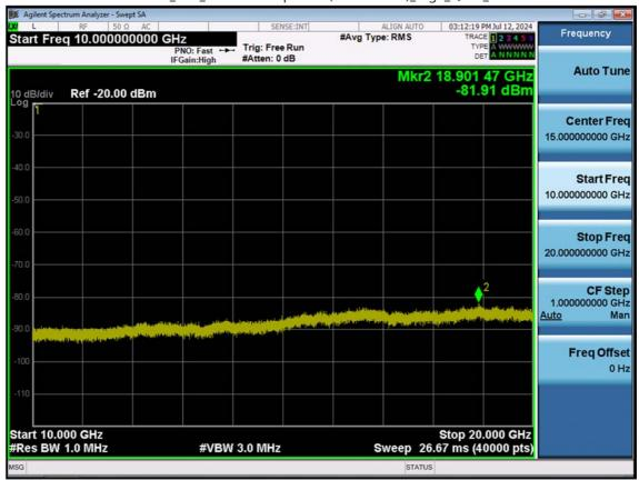
LTE B2\_5 M\_Conducted Spurious(10 G-26.5 G)\_High\_QPSK\_1RB
