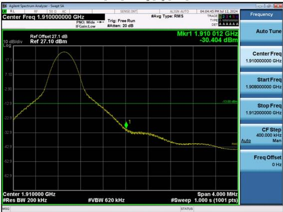
LTE B2\_20 M\_Band Edge\_High\_QPSK\_1RB
