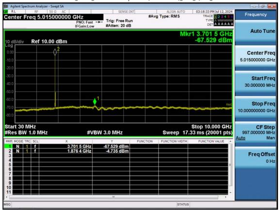
LTE B2\_10 M\_Conducted Spurious(30 M-10 G)\_Mid\_QPSK\_1RB
