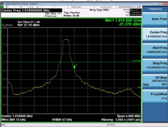
LTE B2\_1.4 M\_Band Edge\_High\_QPSK\_1RB
