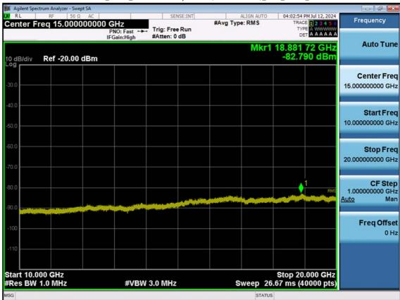
LTE B2\_20 M\_Conducted Spurious(10 G-26.5 G)\_Mid\_QPSK\_1RB
