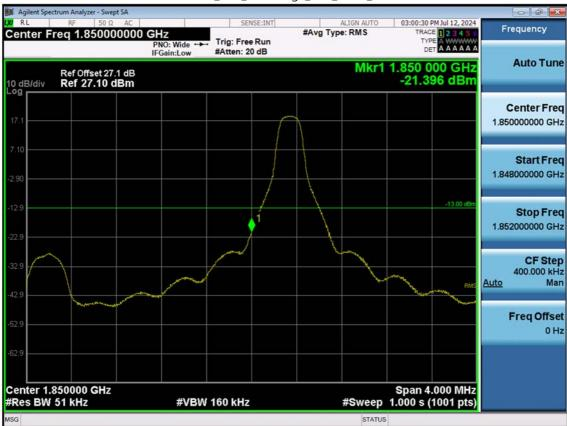
LTE B2\_5 M\_Band Edge\_Low\_QPSK\_1RB
