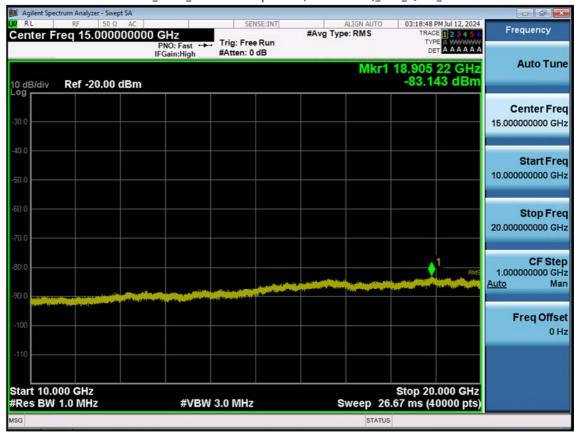
LTE B2\_10 M\_Conducted Spurious(10 G-26.5 G)\_Mid\_QPSK\_1RB
