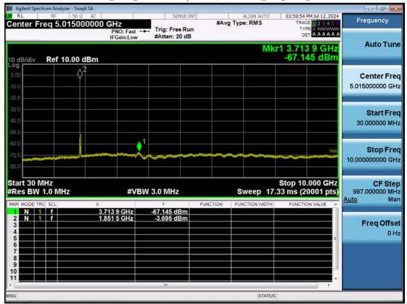
LTE B2\_20 M\_Conducted Spurious(30 M-10 G)\_Low\_QPSK\_1RB
