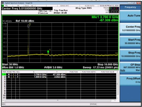
LTE B2\_15 M\_Conducted Spurious(30 M-10 G)\_High\_QPSK\_1RB
