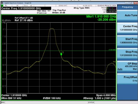
LTE B2\_5 M\_Band Edge\_High\_QPSK\_1RB
