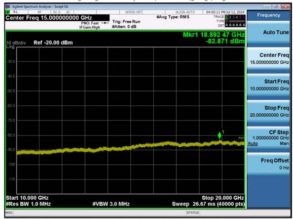
LTE B2\_20 M\_Conducted Spurious(10 G-26.5 G)\_Low\_QPSK\_1RB
