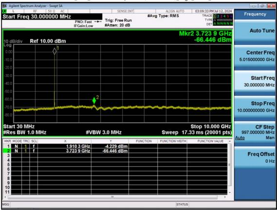
LTE B2\_5 M\_Conducted Spurious(30 M-10 G)\_High\_QPSK\_1RB
