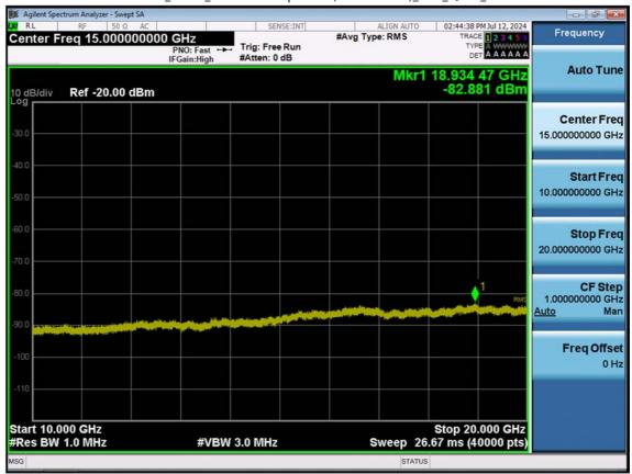
LTE B2\_1.4 M\_Conducted Spurious(10 G-26.5 G)\_Low\_QPSK\_1RB
