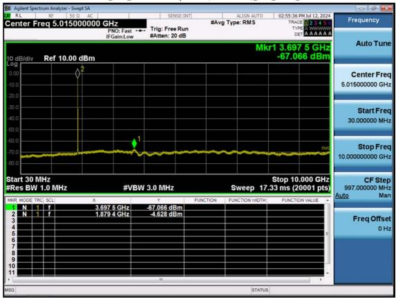
LTE B2\_3 M\_Conducted Spurious(30 M-10 G)\_Mid\_QPSK\_1RB
