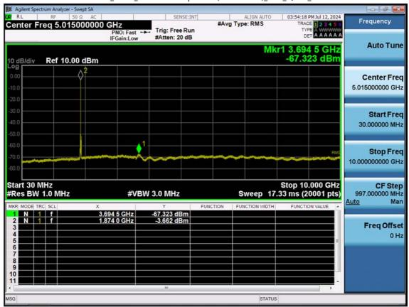
LTE B2\_15 M\_Conducted Spurious(30 M-10 G)\_Mid\_QPSK\_1RB
