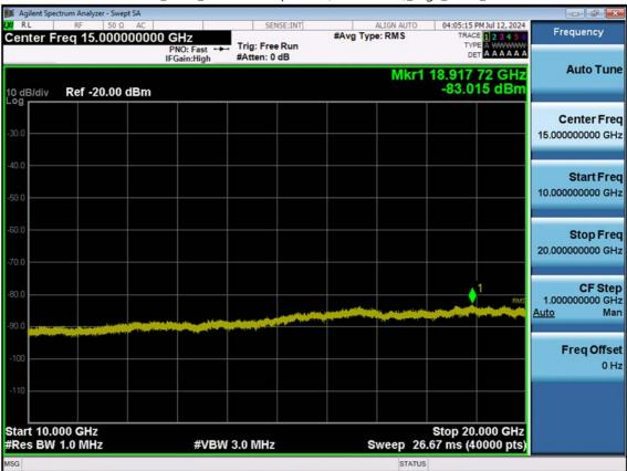
LTE B2\_20 M\_Conducted Spurious(10 G-26.5 G)\_High\_QPSK\_1RB
