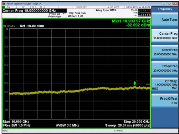
LTE B2\_15 M\_Conducted Spurious(10 G-26.5 G)\_Low\_QPSK\_1RB
