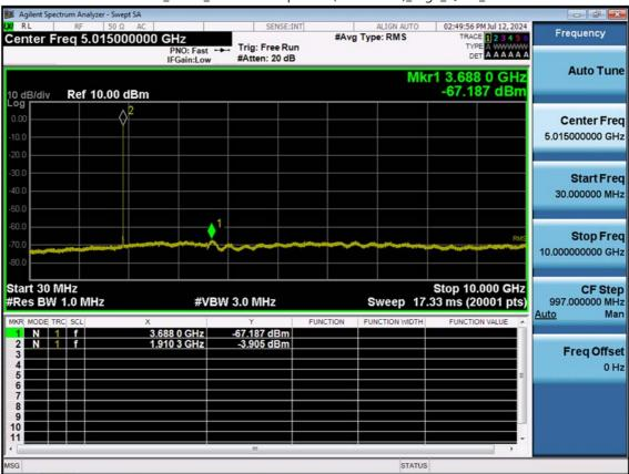
LTE B2\_1.4 M\_Conducted Spurious(30 M-10 G)\_High\_QPSK\_1RB
