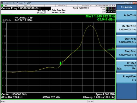
LTE B2\_20 M\_Band Edge\_Low\_QPSK\_1RB
