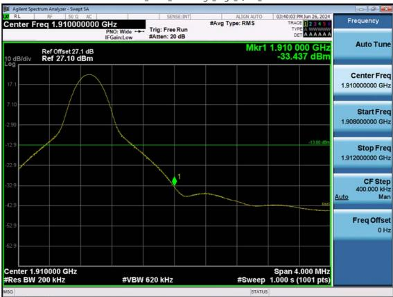
LTE B2\_20 M\_Band Edge\_High\_QPSK\_1RB
