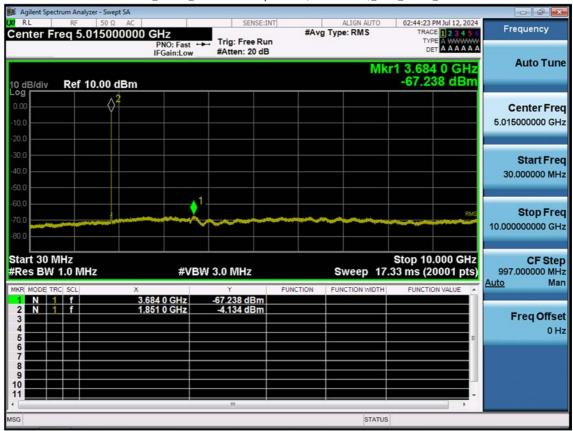
LTE B2\_1.4 M\_Conducted Spurious(30 M-10 G)\_Low\_QPSK\_1RB
