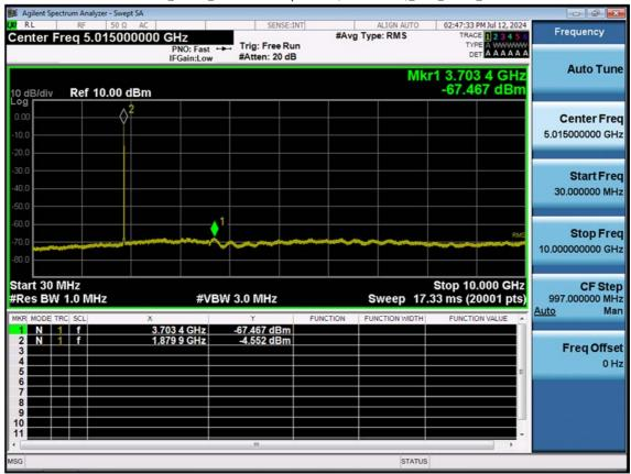
LTE B2\_1.4 M\_Conducted Spurious(30 M-10 G)\_Mid\_QPSK\_1RB
