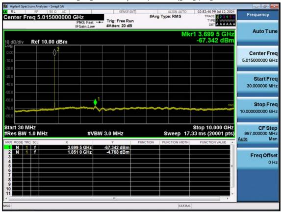
LTE B2\_3 M\_Conducted Spurious(30 M-10 G)\_Low\_QPSK\_1RB
