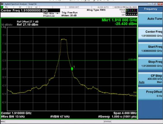
LTE B2\_1.4 M\_Band Edge\_High\_QPSK\_1RB
