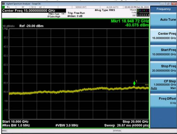
LTE B2\_20 M\_Conducted Spurious(10 G-26.5 G)\_High\_QPSK\_1RB
