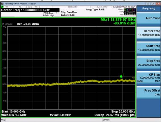
LTE B2\_10 M\_Conducted Spurious(10 G-26.5 G)\_High\_QPSK\_1RB
