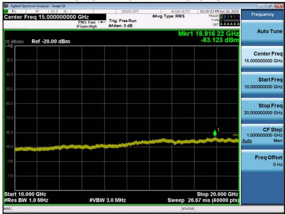
LTE B2\_15 M\_Conducted Spurious(10 G-26.5 G)\_Mid\_QPSK\_1RB
