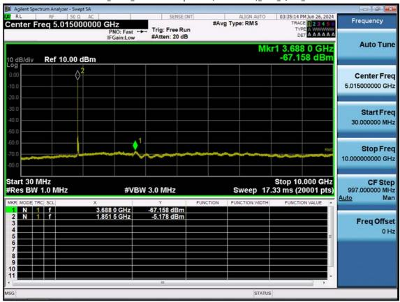
LTE B2\_20 M\_Conducted Spurious(30 M-10 G)\_Low\_QPSK\_1RB
