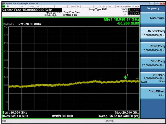
LTE B2\_15 M\_Conducted Spurious(10 G-26.5 G)\_Low\_QPSK\_1RB
