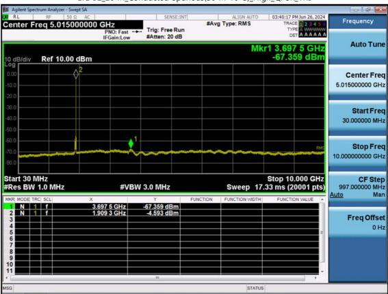
LTE B2\_20 M\_Conducted Spurious(30 M-10 G)\_High\_QPSK\_1RB
