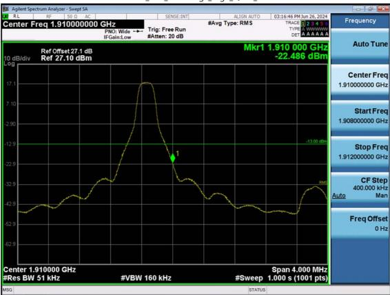
LTE B2\_5 M\_Band Edge\_High\_QPSK\_1RB
