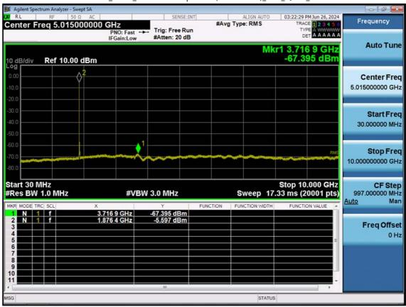
LTE B2\_10 M\_Conducted Spurious(30 M-10 G)\_Mid\_QPSK\_1RB
