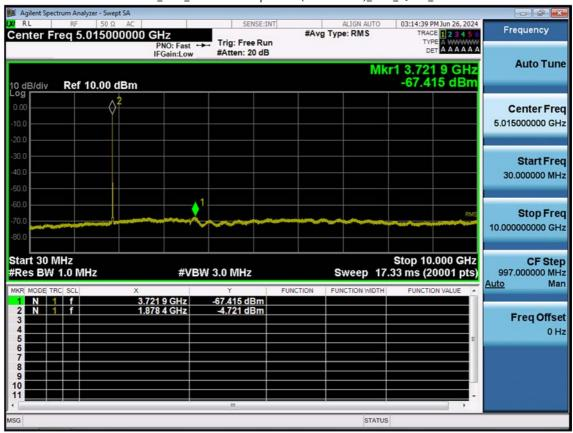
LTE B2\_5 M\_Conducted Spurious(30 M-10 G)\_Mid\_QPSK\_1RB
