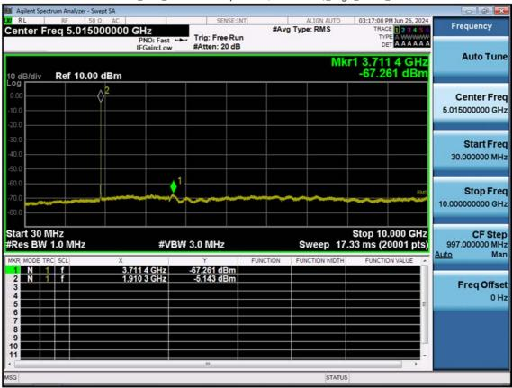
LTE B2\_5 M\_Conducted Spurious(30 M-10 G)\_High\_QPSK\_1RB
