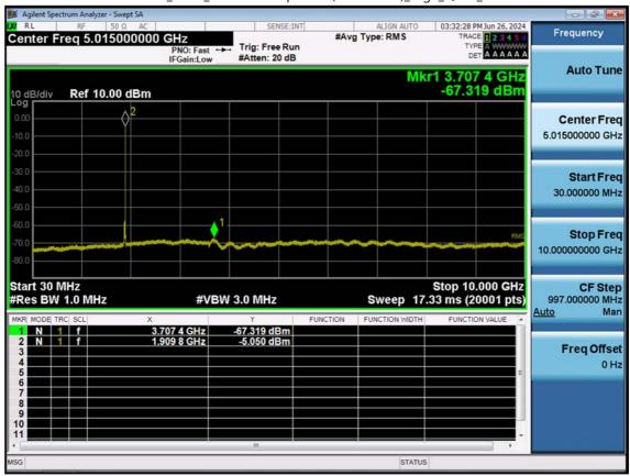
LTE B2\_15 M\_Conducted Spurious(30 M-10 G)\_High\_QPSK\_1RB
