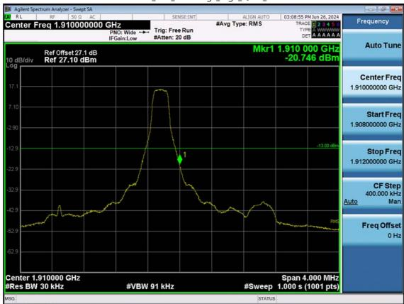
LTE B2\_3 M\_Band Edge\_High\_QPSK\_1RB
