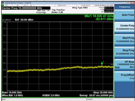
LTE B2\_20 M\_Conducted Spurious(10 G-26.5 G)\_Low\_QPSK\_1RB
