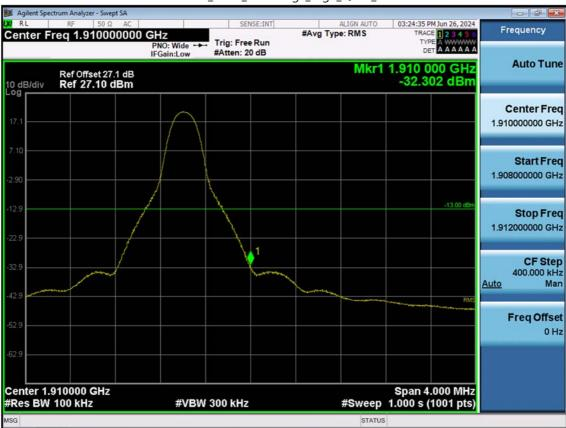
LTE B2\_10 M\_Band Edge\_High\_QPSK\_1RB
