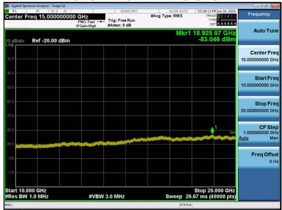
LTE B2\_20 M\_Conducted Spurious(10 G-26.5 G)\_Mid\_QPSK\_1RB
