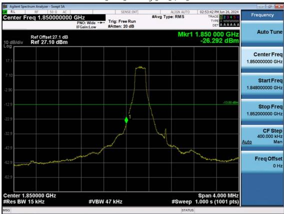
LTE B2\_1.4 M\_Band Edge\_Low\_QPSK\_1RB
