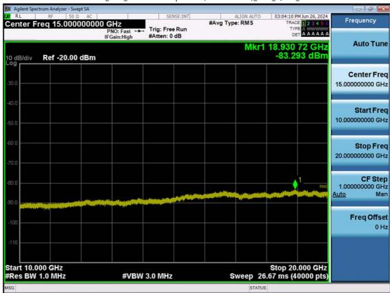
LTE B2\_3 M\_Conducted Spurious(10 G-26.5 G)\_Low\_QPSK\_1RB
