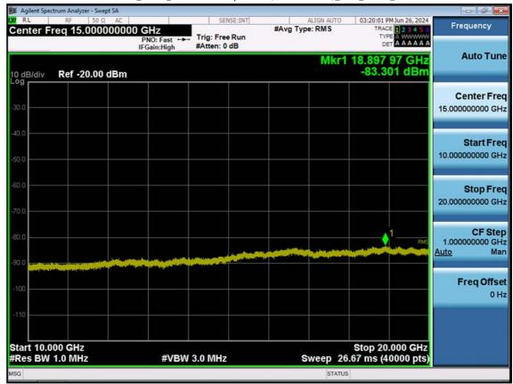
LTE B2\_10 M\_Conducted Spurious(10 G-26.5 G)\_Low\_QPSK\_1RB
