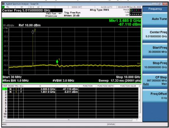
LTE B2\_10 M\_Conducted Spurious(30 M-10 G)\_Low\_QPSK\_1RB
