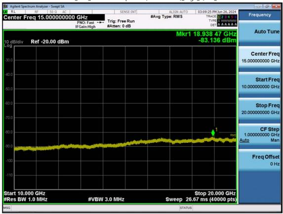
LTE B2\_3 M\_Conducted Spurious(10 G-26.5 G)\_High\_QPSK\_1RB
