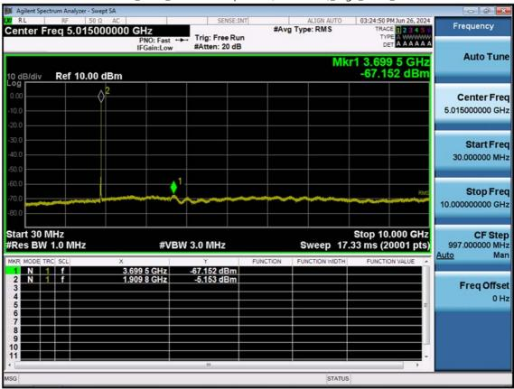
LTE B2\_10 M\_Conducted Spurious(30 M-10 G)\_High\_QPSK\_1RB
