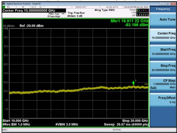
LTE B2\_10 M\_Conducted Spurious(10 G-26.5 G)\_Mid\_QPSK\_1RB
