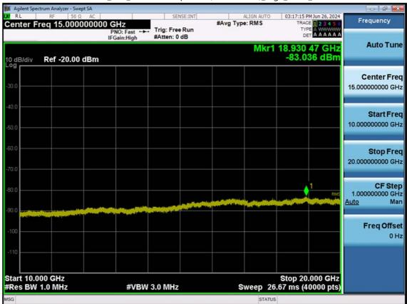
LTE B2\_5 M\_Conducted Spurious(10 G-26.5 G)\_High\_QPSK\_1RB
