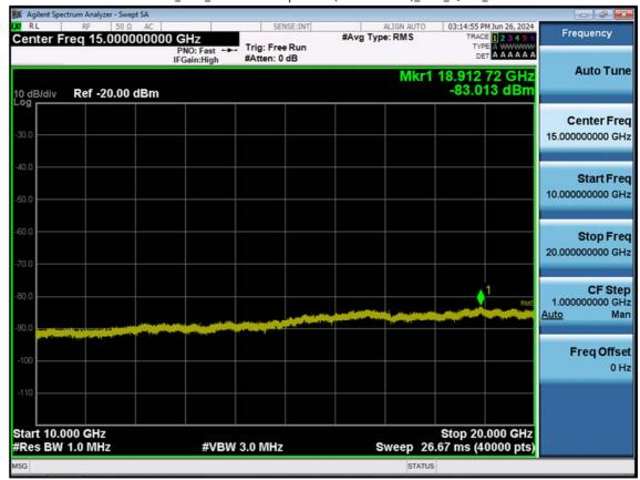
LTE B2\_5 M\_Conducted Spurious(10 G-26.5 G)\_Mid\_QPSK\_1RB
