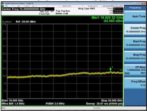
LTE B2\_15 M\_Conducted Spurious(10 G-26.5 G)\_High\_QPSK\_1RB
