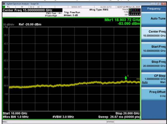
LTE B2\_1.4 M\_Conducted Spurious(10 G-26.5 G)\_Mid\_QPSK\_1RB
