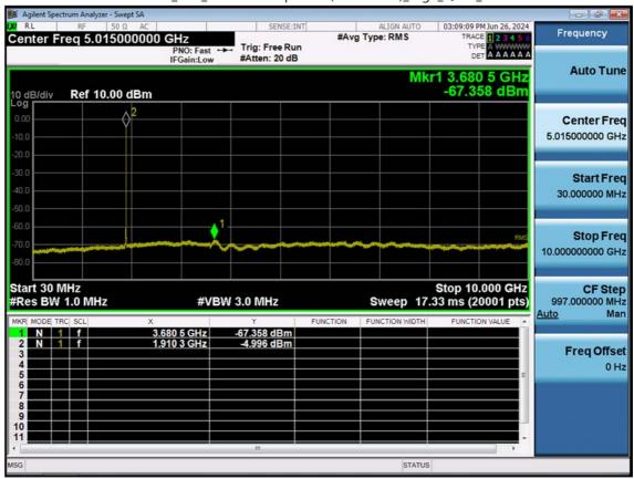
LTE B2\_3 M\_Conducted Spurious(30 M-10 G)\_High\_QPSK\_1RB
