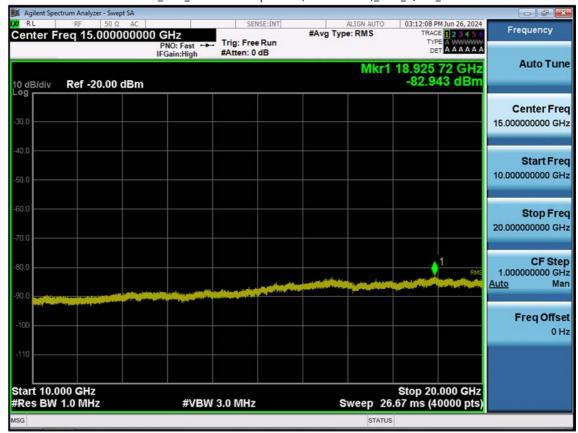
LTE B2\_5 M\_Conducted Spurious(10 G-26.5 G)\_Low\_QPSK\_1RB
