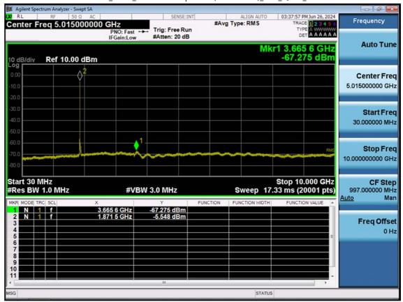
LTE B2\_20 M\_Conducted Spurious(30 M-10 G)\_Mid\_QPSK\_1RB
