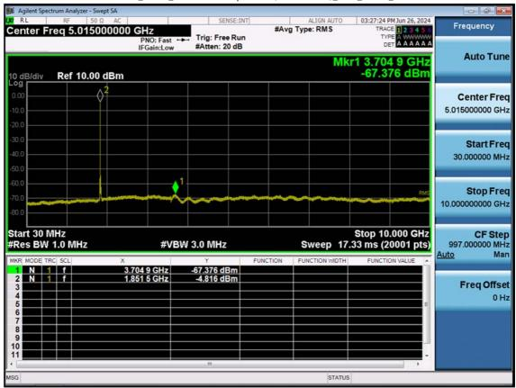
LTE B2\_15 M\_Conducted Spurious(30 M-10 G)\_Low\_QPSK\_1RB
