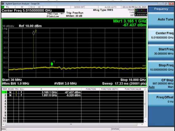
LTE B2\_5 M\_Conducted Spurious(30 M-10 G)\_Low\_QPSK\_1RB
