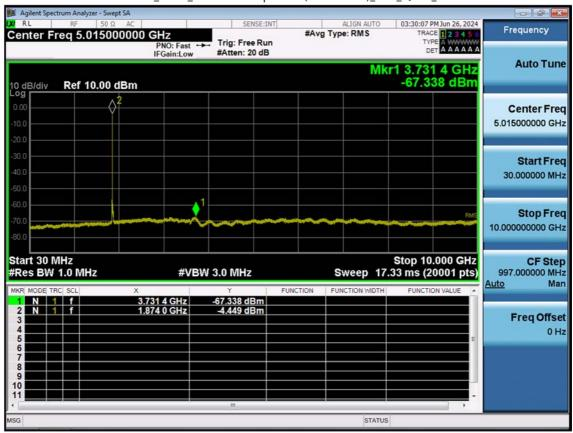
LTE B2\_15 M\_Conducted Spurious(30 M-10 G)\_Mid\_QPSK\_1RB
