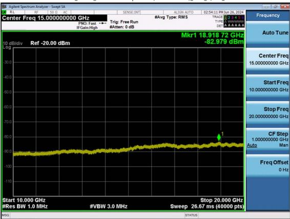
LTE B2\_1.4 M\_Conducted Spurious(10 G-26.5 G)\_Low\_QPSK\_1RB
