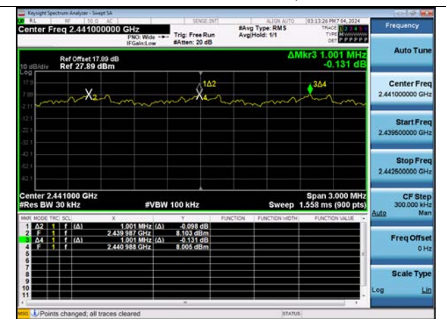
ANT. 2 8DPSK : Channel Separation
