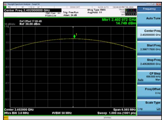
ANT.2 \pi /4DQPSK : Peak Power (CH. 0)
