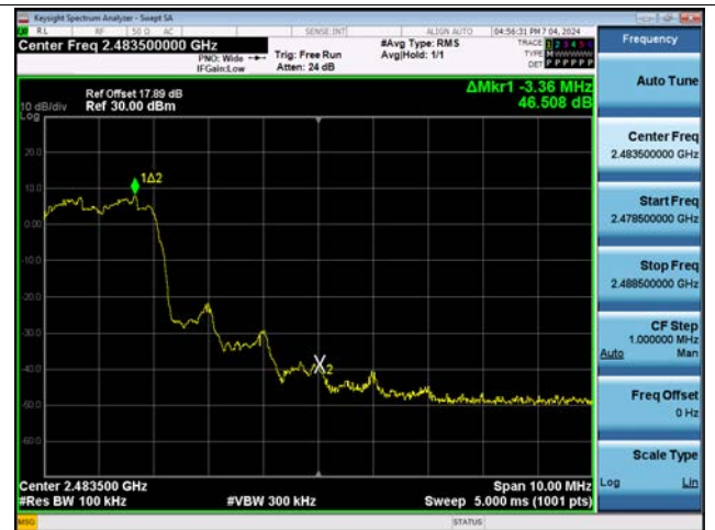
Dual ANT.2 8DPSK Band Edge(CH.78)
