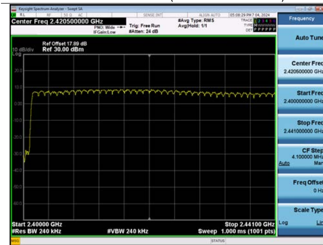
Dual ANT.2 \pi/4 DQPSK Number of Channels (2.4 GHz - 2.441 GHz)
