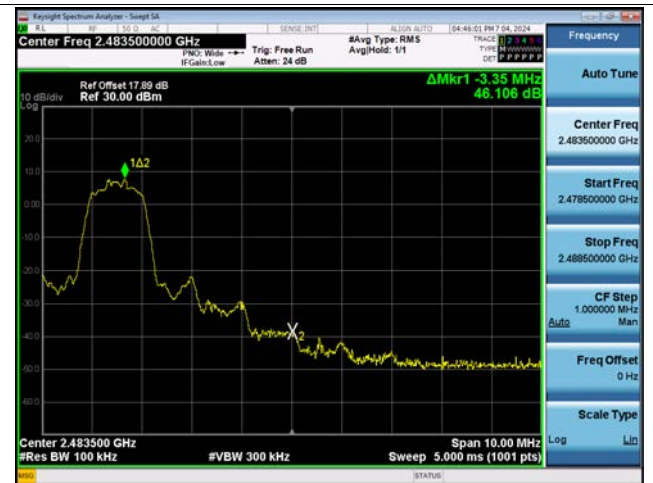
Dual ANT.2 \pi/4 DQPSK Band Edge(CH.78)
