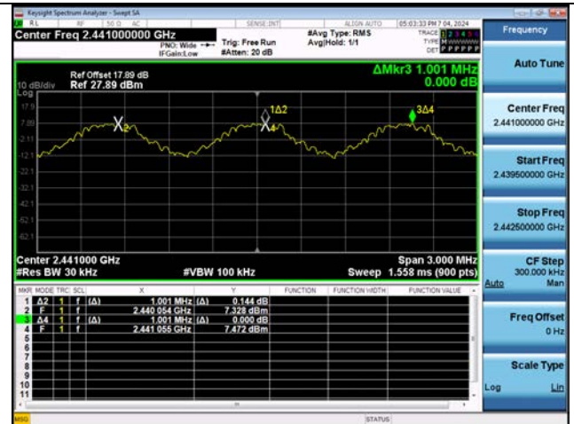
Dual ANT. 2 \pi/4 DQPSK : Channel Separation
