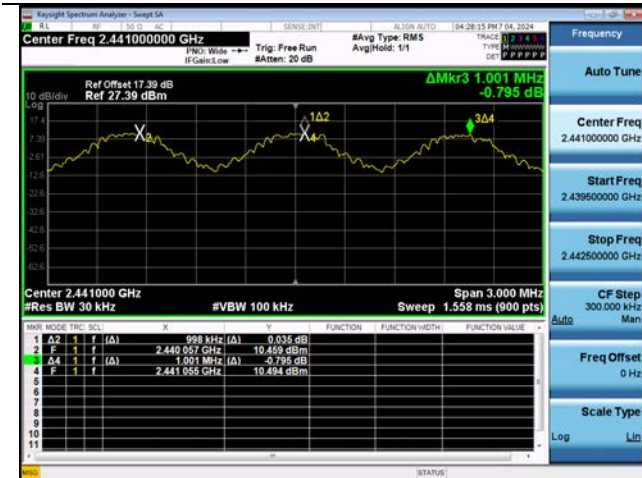
Dual ANT. 1 \pi/4 DQPSK : Channel Separation
