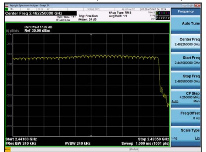
Dual ANT.2 \pi/4 DQPSK Number of Channels (2.441 GHz - 2.483.5 GHz)
