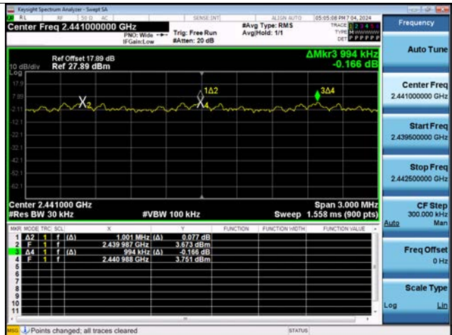
Dual ANT. 2 8DPSK : Channel Separation
