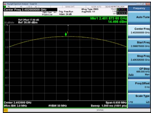
ANT.2 \pi /4DQPSK : Peak Power (CH. 0)
