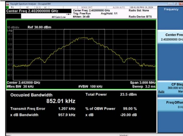
ANT. 1 8DPSK 20 dB BW & 99% OBW (CH. 39)
