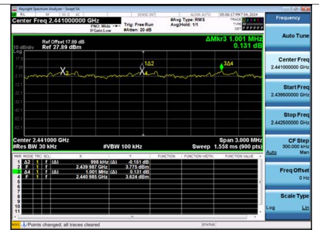
Dual ANT. 2 8DPSK : Channel Separation
