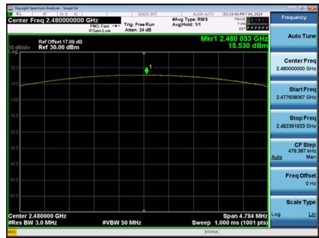
ANT.2 8DPSK : Peak Power (CH. 0)
