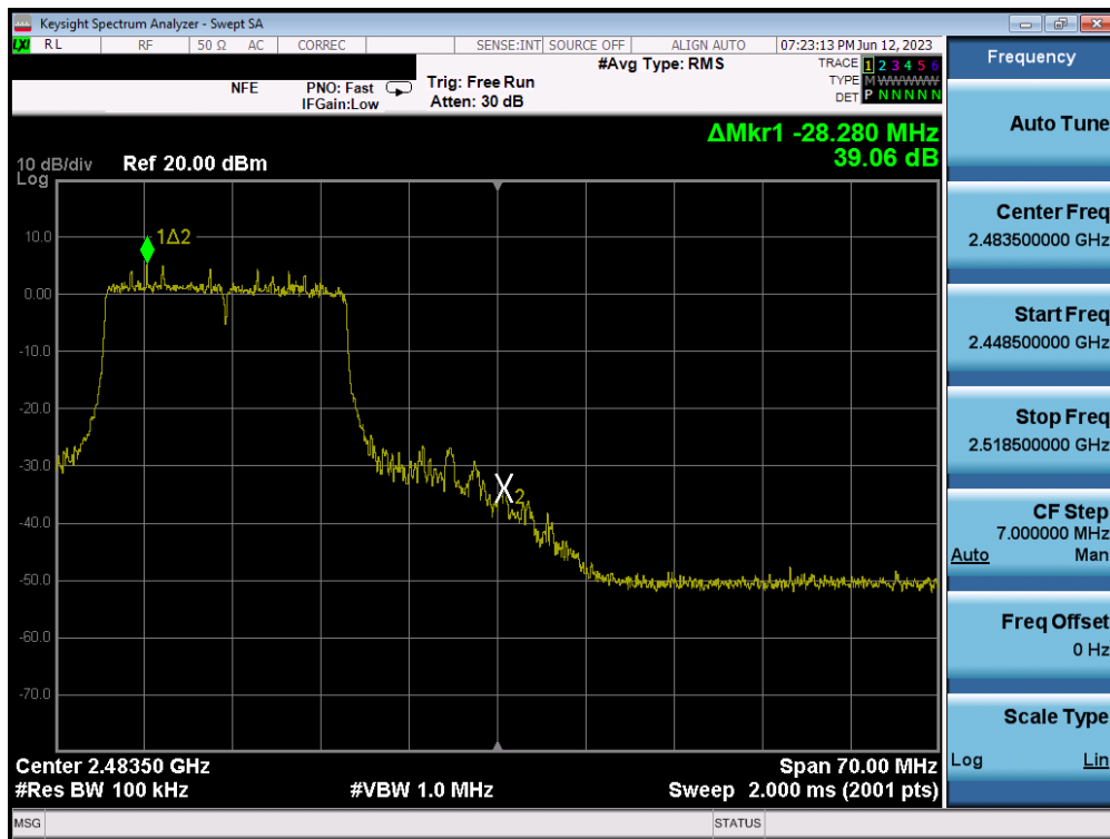
Plot 7-40. Band Edge Plot SISO ANT2 (802.11ax OFDMA – 242 Tones – Ch. 11)
